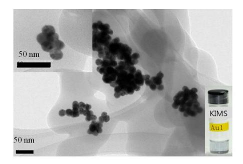
Supporting 1 Au nanoparticles synthesized in the present work were characterized using Transmission electron microscopy (TEM).
