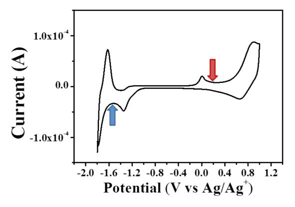
Supporting 2 Cyclic voltammetry (CV) data of PTB7-F20. It was found that the energy positions of Highest Occupied Molecular Orbital (HOMO) and Lowest Unoccupied Molecular Orbital (LUMO) of PTB7-F20 are between the respective values PTBF0 (without F, X=0, see Fig. 1) and PTBF1 (with F, X=1, See Fig. 1). 9,11
