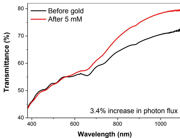
**Figure S6.** Transmittance of the super acid SWNT films change with the doping of gold salt.
