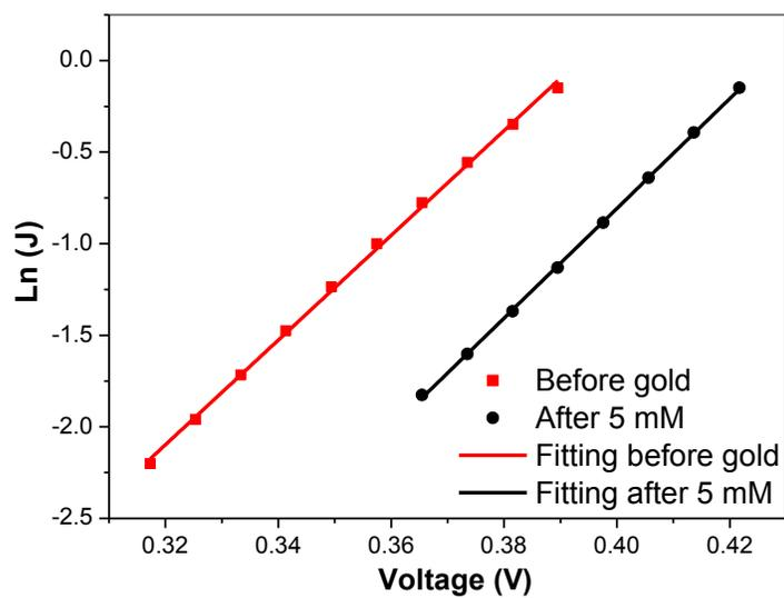
**Figure S8.**  $J$ - $V$  characteristics in the semi-logarithmic scale at the forward linear region.
