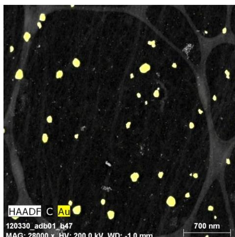
**Figure S7.** Energy-dispersive x-ray spectroscopy elemental mapping of gold doped SWNT films.
