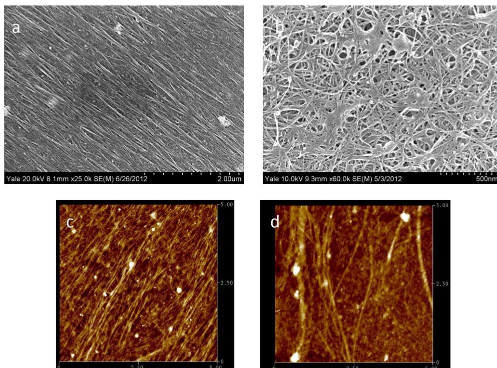
**Figure S1.** SEM image of (a) superacid SWNTs looking from bottom side (side in contact with silicon in final device). Carbon nanotubes are aligned in the shearing direction. (b) Mayer rod coated thin films. AFM image on the top side of superacid film (c) slowly dried in anhydrous air with roughness of 4.12 nm (d) coagulated in water with roughness of 9.99 nm.
