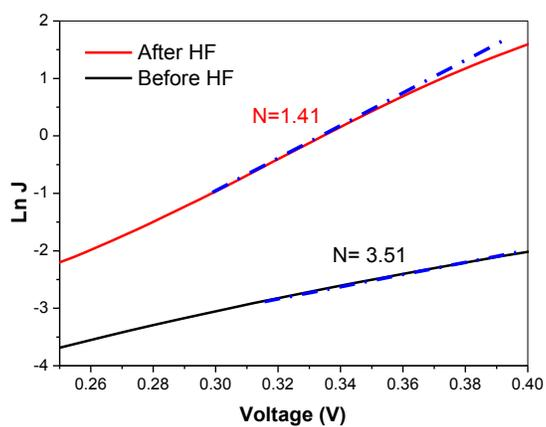
**Figure S2.**  $\ln(J)$ - $V$  under small forward bias assesses the quality of the solar cell devices: Mayer rod fabricated SWNT/Si device before and after HF treatment.
