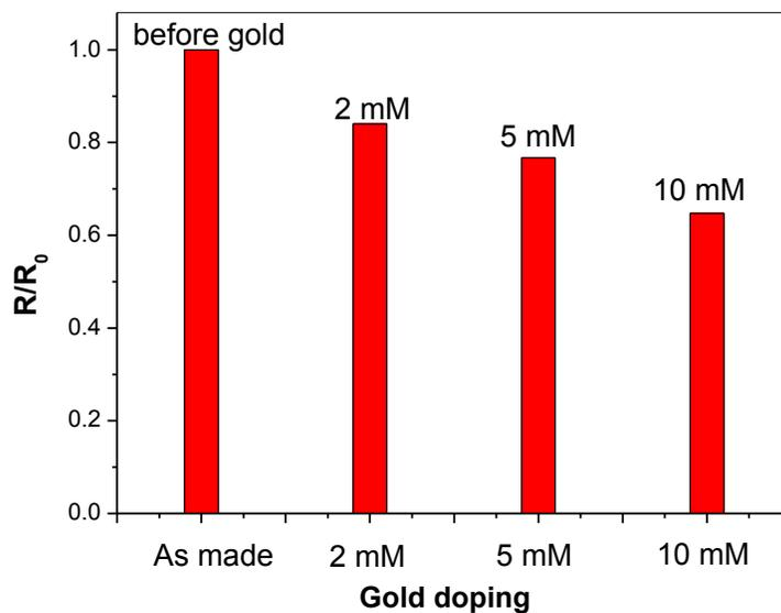
**Figure S9.** Sheet resistance of the super acid SWNT films change with the gold salt doping.
