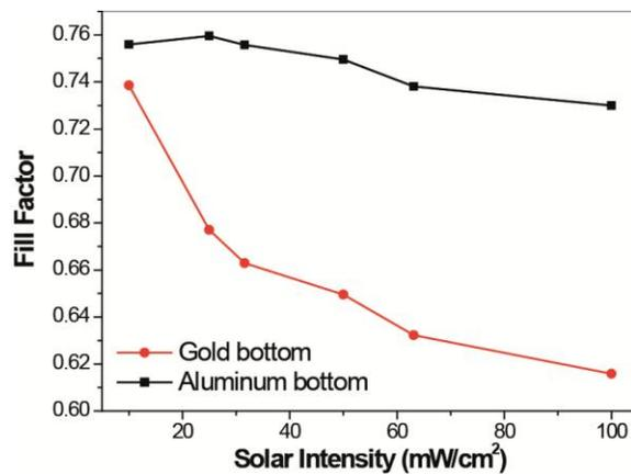
**Figure S10.** Solar intensity dependent variation of fill factor (FF) with back contacts of Au and Al.
