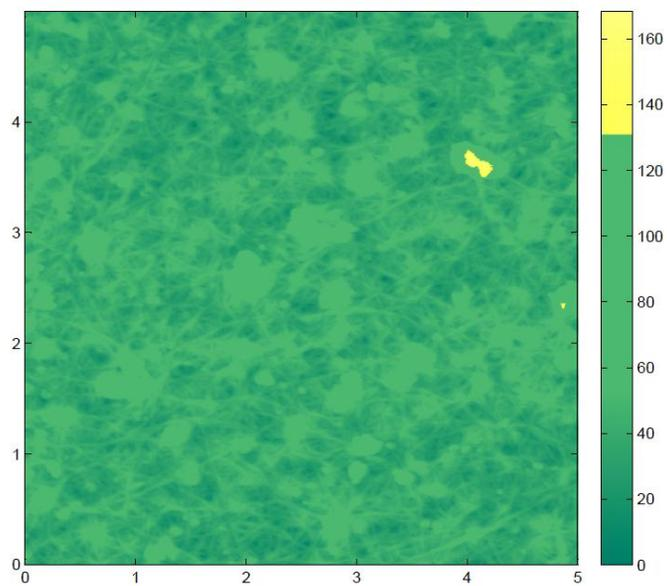
**Figure S3.** Visualization of the SWNTs in contact with Si (yellow) and not in contact with Si (green) for a Mayer rod SWNT film assuming a depth of 37.88 nm.
