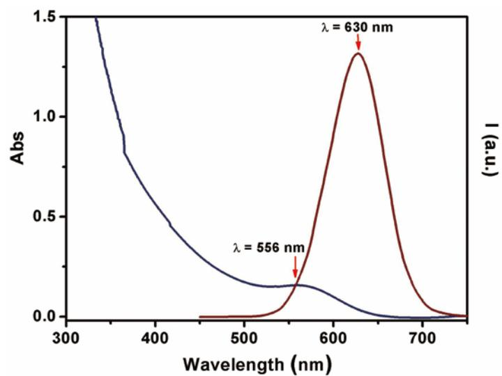
Figure S1. UV-vis absorption and luminescent spectra of MPA-CdTe QDs ( $0.2 \text{ mg}\cdot\text{mL}^{-1}$ ,  $1.2 \times 10^{-6} \text{ M}$ ) in water (excitation wavelength: 406 nm).
