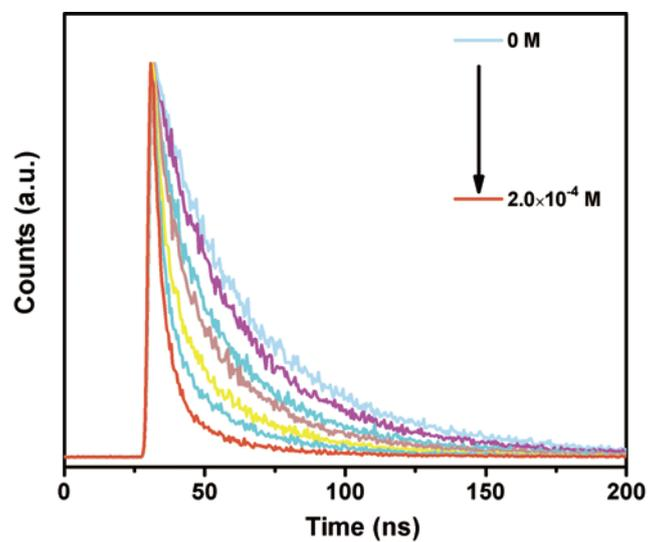
Figure S7. The luminescence decays (630-665 nm) of MPA-CdTe QDs ( $4.8 \times 10^{-7}$  M,  $8.0 \times 10^{-2}$   $\text{mg} \cdot \text{mL}^{-1}$ ) with various concentrations of  $\text{CoCl}_2 \cdot 6\text{H}_2\text{O}$  (0 to  $2.0 \times 10^{-4}$  M) in water (excitation wavelength: 406 nm).
