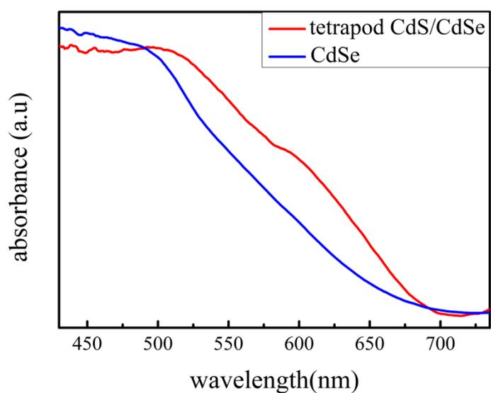
Figure S5: UV-Vis spectra of photoanodes with TiO<sub>2</sub> sensitized by CdSe (SILAR) and tetrapod-CdS(linker assisted)
