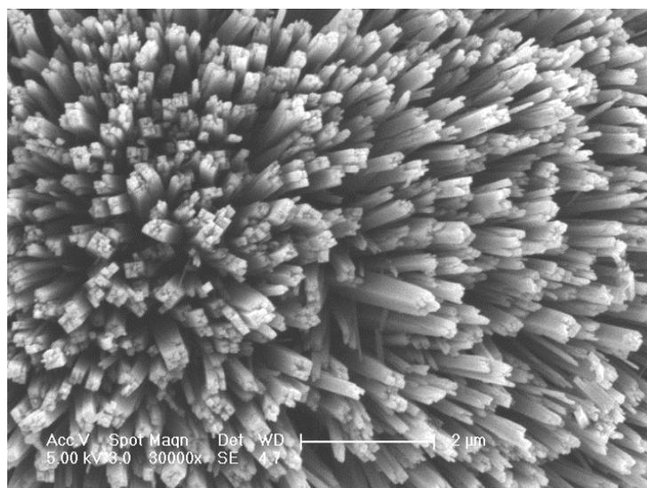
Figure S3: SEM micrograph of as-synthesized TiO<sub>2</sub> nanorod (absorption layer) vertically aligned on FTO substrate coated with a compact and transparent layer of TiO<sub>2</sub>.
