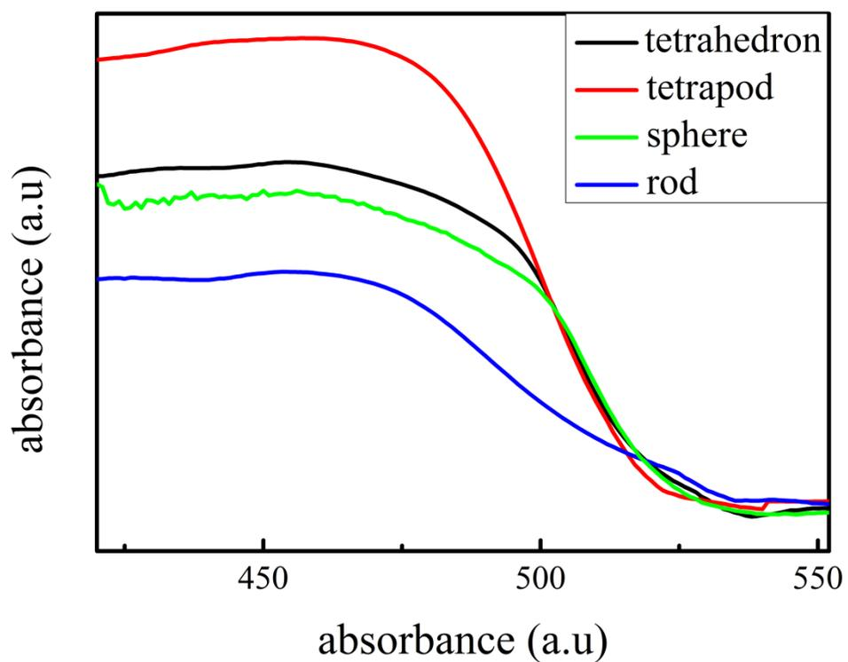
Figure S4: UV-Vis spectra of photoanodes with TiO<sub>2</sub> sensitized by various shapes of CdS
