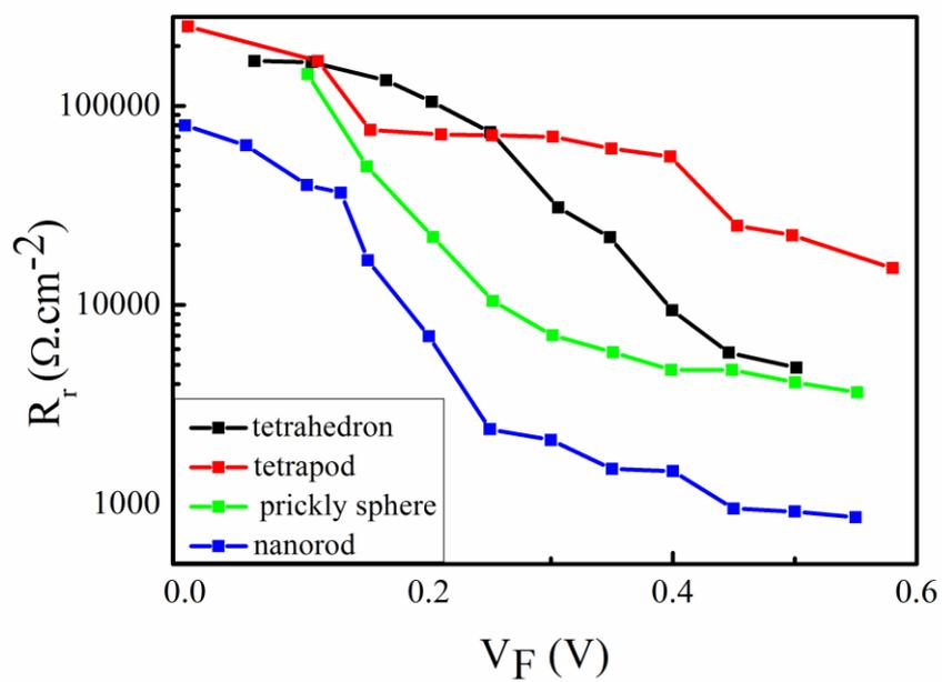
Figure S6: Recombination resistances of solar cells sensitized by various shapes of CdS
