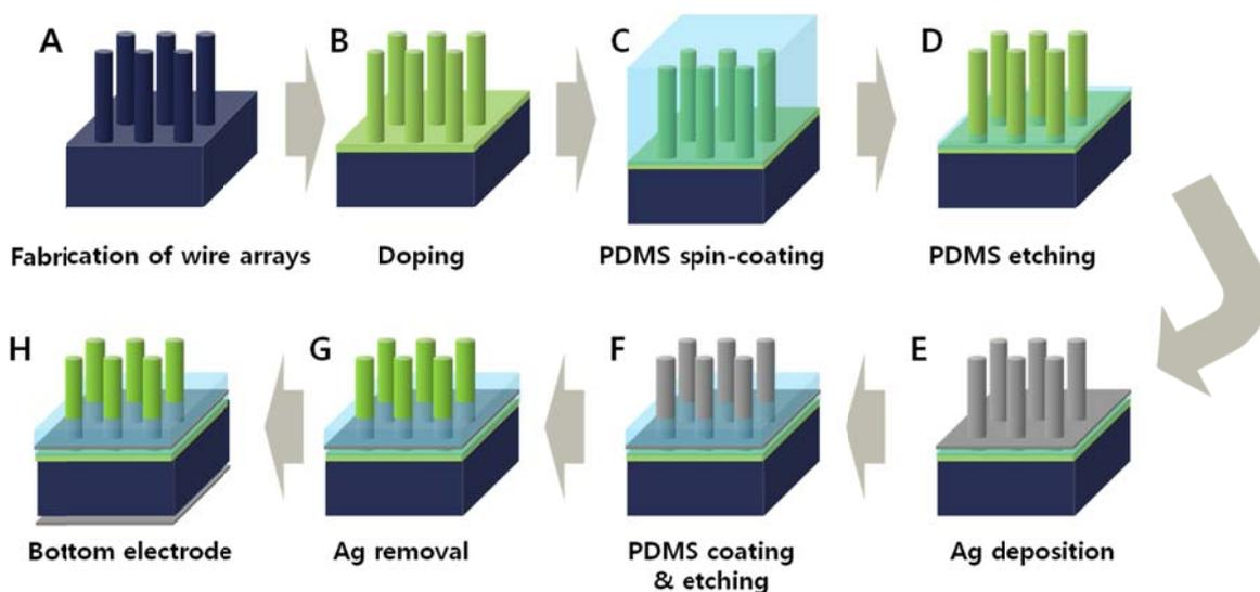
**Step A:** A periodic array of silicon microwires
