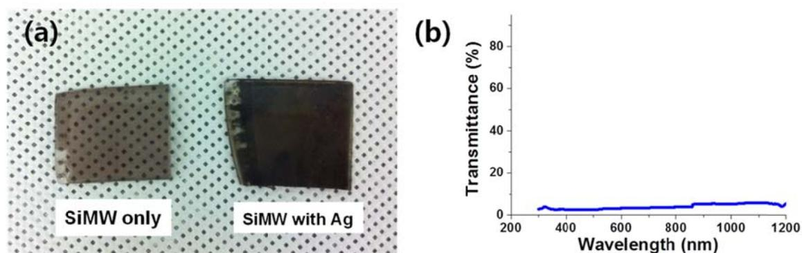
Our light absorptance (Fig. 1c) data were measured by using the wire arrays [Fig. S2(a)] detached from the substrate. However, the electrical properties were measured before removing from the substrate because we have confirmed that light absorption into a substrate was negligible [Fig. S2(b)]. After removing from the substrate, low transmittance of 3~4% was observed from the wire arrays containing Ag electrodes.
