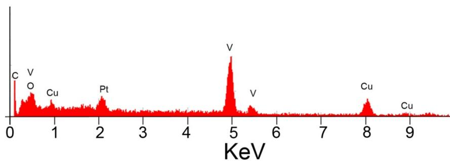
**Figure S2.** The EDX spectrum of the precursor hollow microflowers. Cu and Pt signals are from the substrate and Pt sputtering for FESEM observation, respectively.
