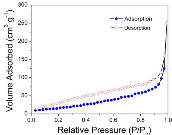
**Figure S3.** Nitrogen adsorption-desorption isotherm of  $V_2O_5$  nanosheet-assembled hollow microflowers.
