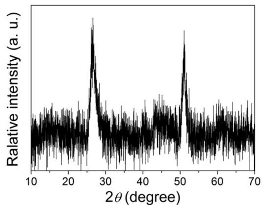
**Figure S1.** XRD pattern for the precursor hierarchical hollow microflowers solvothermally prepared from the solution of 0.2 mL of VOT in 30 mL of IPA at 200 °C for 12 h.
