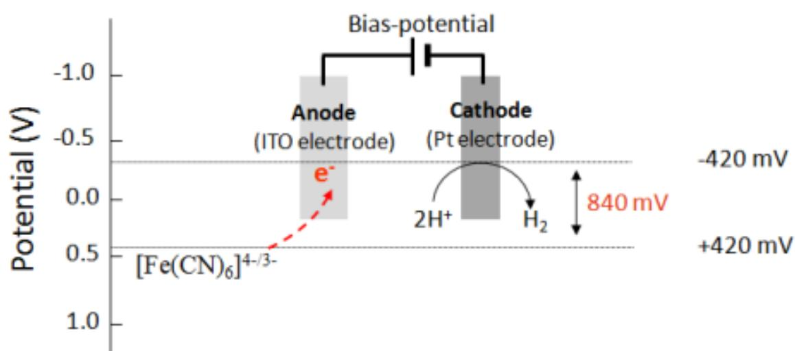
**Supp. Figure 3.** Summary of reaction potentials of anodic and cathodic half-reactions in the BPE system. In the absence of an applied bias-potential the reaction is thermodynamically unfavourable. The  $\text{Fe}(\text{CN})_6^{4-/3-}$  couple (+420 mV) is more positive than the  $\text{H}_2 / 2\text{H}^+$  couple (-420 mV), so an extra energy input in the form of a bias potential (a minimum of 840 mV) is required to drive the reaction forward.
