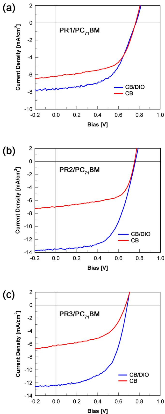
**Fig. S3** J-V curves of PSCs of random copolymers fabricated under different conditions.
