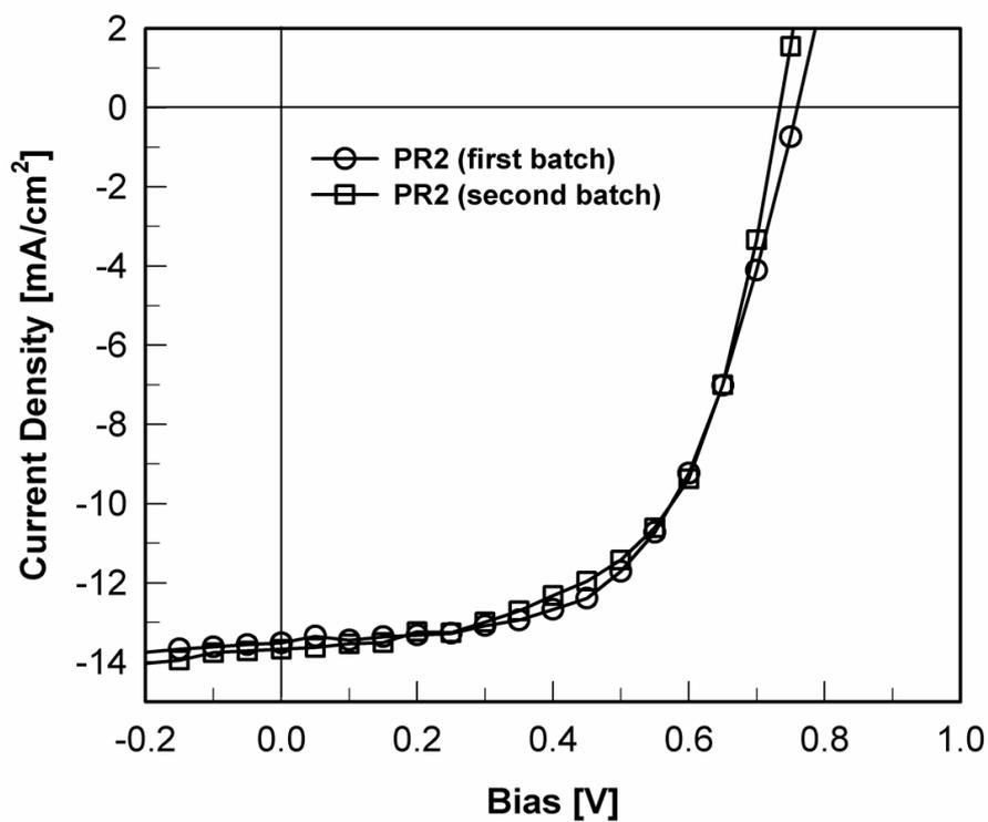
**Fig. S9** *J*-*V* curves of polymer solar cells made of first and second batches of PR2, respectively.
