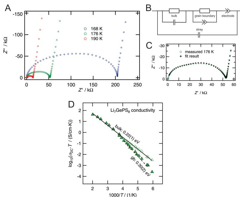
**Fig. 4:** Impedance spectroscopy on  $\text{Li}_7\text{GePS}_8$ . (A): Nyquist impedance plot for selected temperatures. (B): Equivalent circuit used for the analysis. (>) denotes a constant phase element. (C): Fit result exemplarily shown for 176 K. (D): Full triangles: normalized total impedance as read out (model-independent) from the Nyquist plots shown in (A). Empty triangles: bulk impedance as obtained from the model-dependent fit.
