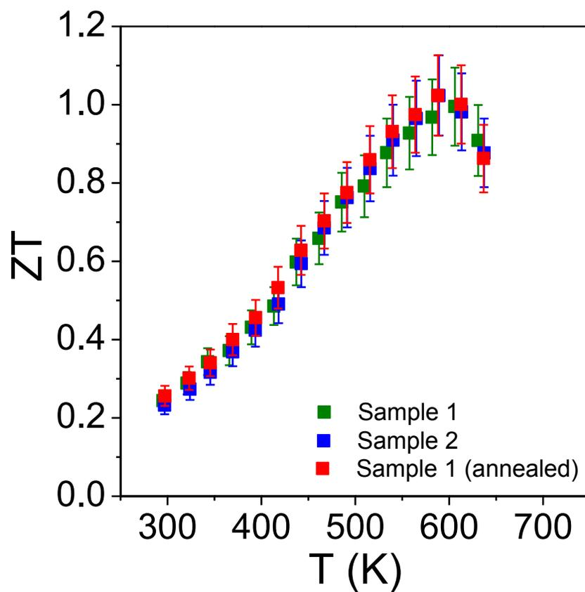
**Fig. S5**  $ZT$  (with 10% error bar) obtained on multiple  $\text{AgSb}_{0.96}\text{Pb}_{0.04}\text{Se}_2$  samples with same nominal composition obtained from different synthesis. Annealed (673 K for 15 h) samples also show similar  $ZT$ , which confirms the thermal stability at high temperature.
