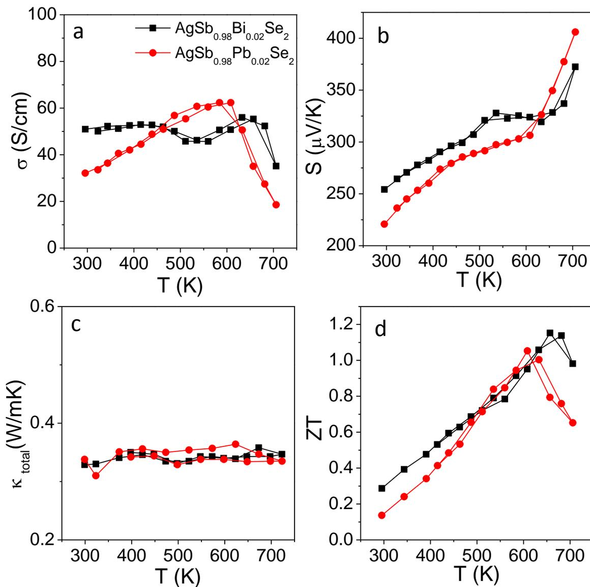
**Fig. S6** Heating-cooling cycle of temperature-dependent (a) electrical conductivity ( $\sigma$ ), (b) Seebeck coefficient ( $S$ ), (c) total thermal conductivity ( $\kappa_{\text{total}}$ ) and (d) thermoelectric figure of merit ( $ZT$ ) plot of  $\text{AgSb}_{0.98}\text{Bi}_{0.02}\text{Se}_2$  and  $\text{AgSb}_{0.98}\text{Pb}_{0.02}\text{Se}_2$ . Heating and cooling cycles give repeatable transport properties for a given sample, which confirms the high temperature stability of the samples.
