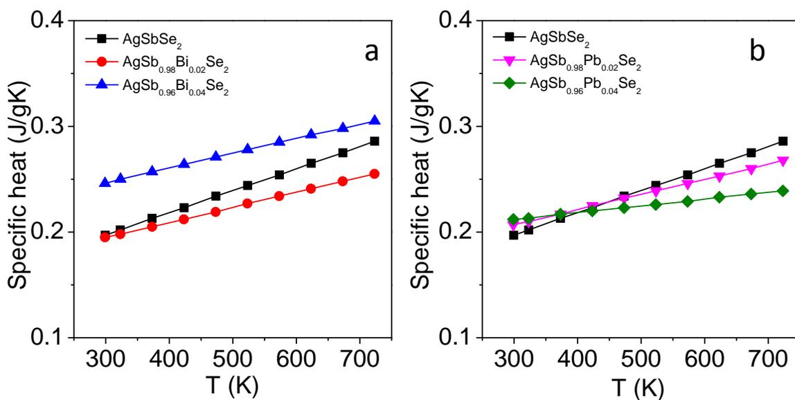
**Fig. S3** Temperature dependent specific heat of (a)  $\text{AgSb}_{1-x}\text{Bi}_x\text{Se}_2$  ( $x= 0-0.04$ ) and (b)  $\text{AgSb}_{1-x}\text{Pb}_x\text{Se}_2$  ( $x= 0- 0.04$ ).
