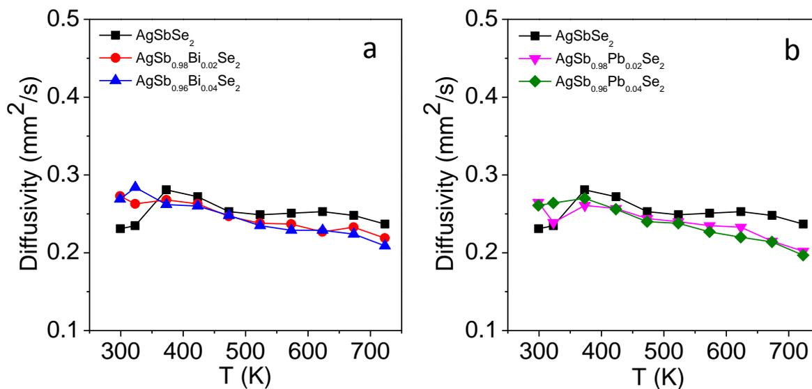
**Fig. S2** Temperature dependent thermal diffusivity of (a) AgSb<sub>1-x</sub>Bi<sub>x</sub>Se<sub>2</sub> (x= 0-0.04) and (b) AgSb<sub>1-x</sub>Pb<sub>x</sub>Se<sub>2</sub> (x= 0- 0.04).
