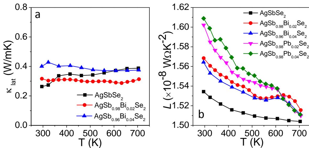
**Fig. S4** (a) Temperature dependent lattice thermal conductivity ( $\kappa_{lat}$ ) of  $\text{AgSb}_{1-x}\text{Bi}_x\text{Se}_2$  ( $x= 0.02, 0.04$ ) and pristine  $\text{AgSbSe}_2$ . (b) Calculated Lorenz numbers based on the fitting of respective Seebeck coefficient values to estimate the reduced chemical for pristine and doped samples.
