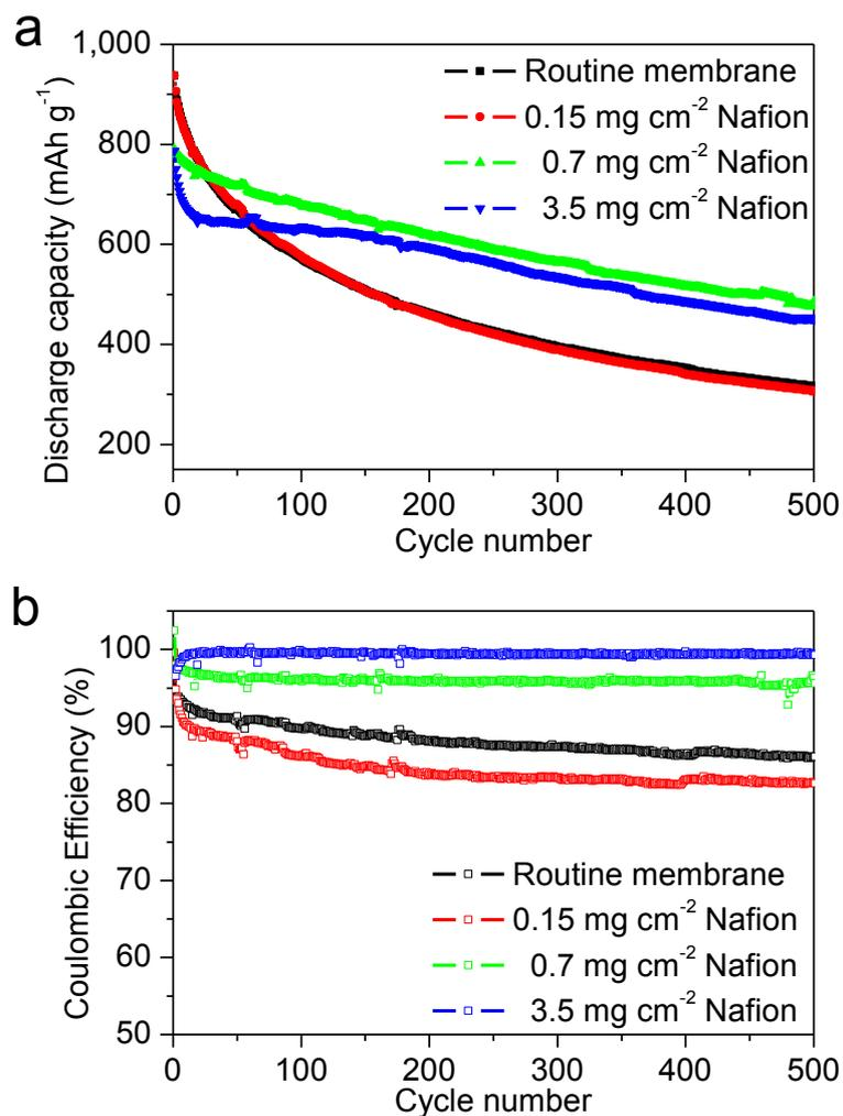
**Figure S2.** The electrochemical performances. (a) The change of discharge capacities vs. the cycle number and (b) The coulombic efficiencies vs. the cycle number. Charge and discharge current density of 1 C, corresponding to a current density of 0.89 mA cm<sup>-2</sup>.
