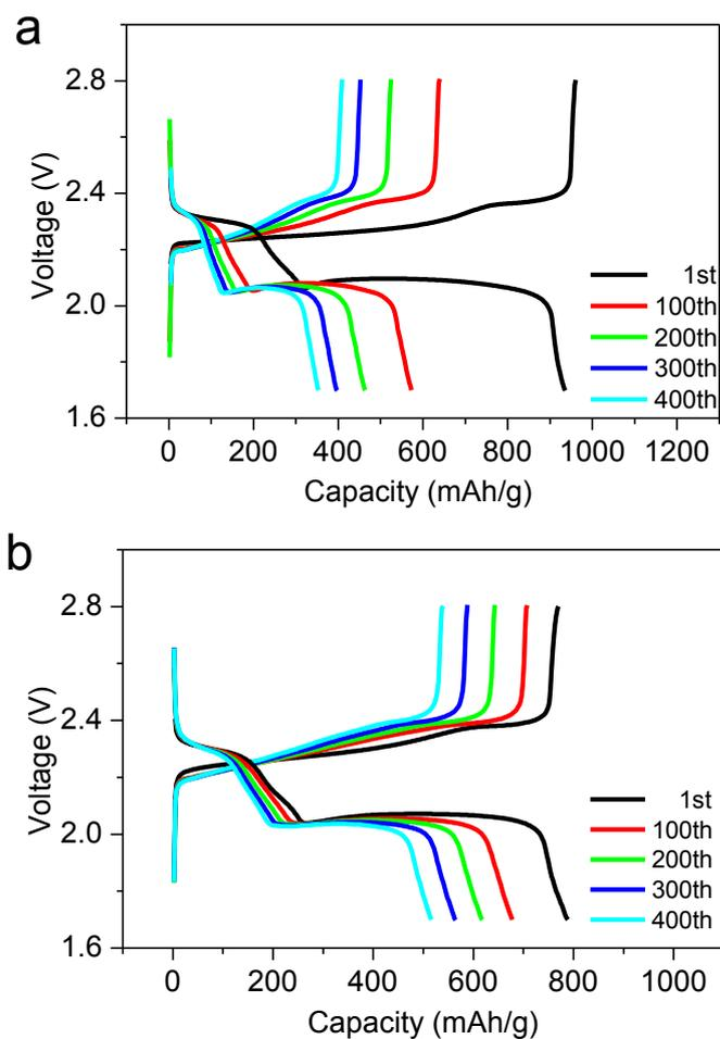
**Figure S3.** The voltage profiles of cells with routine and ion selective membranes. (a) The voltage profile of cell with routine membrane. (b) The voltage profile of cell with ion selective membranes. Charge and discharge current density of 1 C, corresponding to a current density of  $0.89 \text{ mA cm}^{-2}$ .
