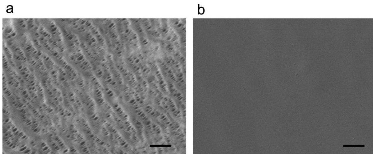
**Figure S1.** The morphologies of membranes. (a) The SEM image for Celgard membrane with the Nafion loading amount of  $0.15 \text{ mg cm}^{-2}$ . (b) The SEM image for Celgard membrane with the Nafion loading amount of  $3.5 \text{ mg cm}^{-2}$  (b). Scale bar:  $1 \mu\text{m}$ .
