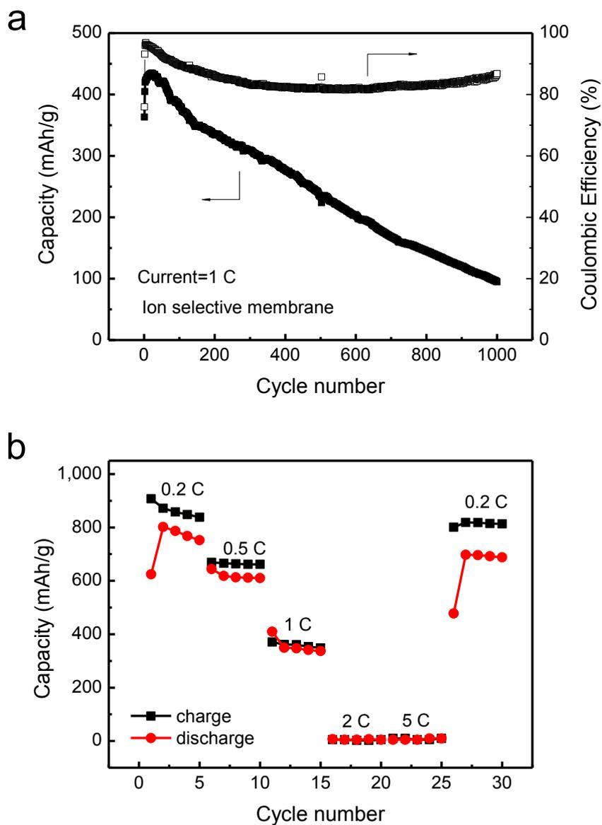
**Figure S6.** Electrochemical performances with different loading methods. (a) The cyclic performance of cell with direct Nafion loading on carbon/sulfur electrode, current density of 1C, corresponding to  $0.89 \text{ mA cm}^{-2}$ . (b) The rate performance of cell. Nafion loading amount of  $0.7 \text{ mg cm}^{-2}$ .
