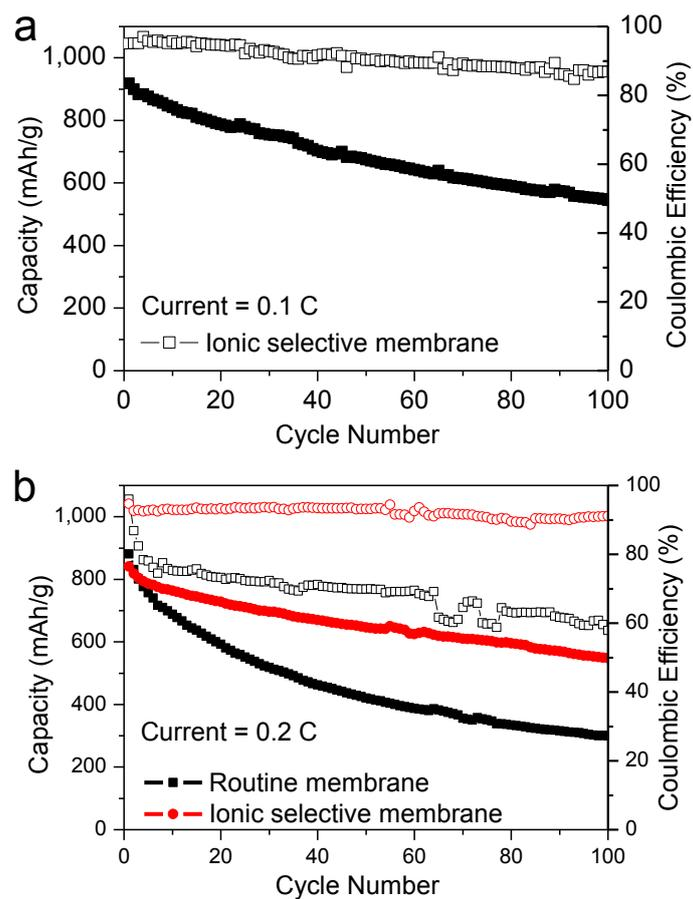
**Figure S4.** Electrochemical performances at low current densities. (a) The performance of ion selective membrane at 0.1 C, corresponding to a current density of  $0.09 \text{ mA cm}^{-2}$ . (b) The performance of routine and ion selective membrane at 0.2 C, corresponding to a current density of  $0.18 \text{ mA cm}^{-2}$ .
