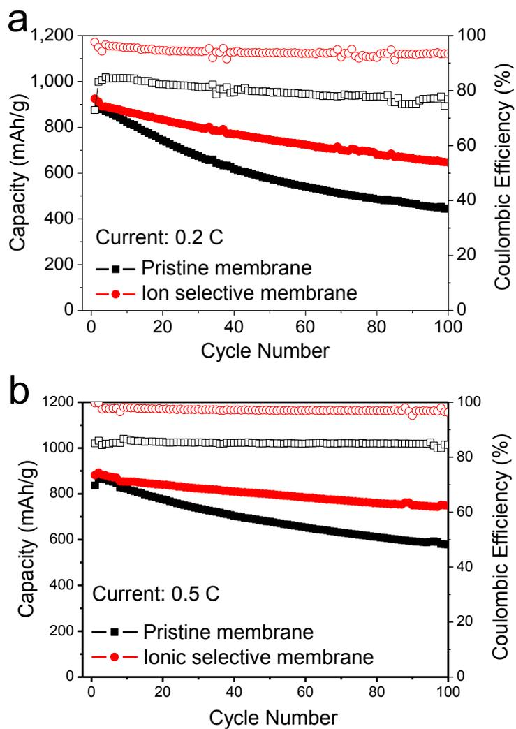
**Figure S5.** Electrochemical performances with different electrodes. The performance of ion selective membrane on SWCNT/S electrodes: (a) cyclic performance at 0.2 C (0.18 mA cm<sup>-2</sup>). (b) cyclic performance at 0.5 C (0.46 mA cm<sup>-2</sup>).
