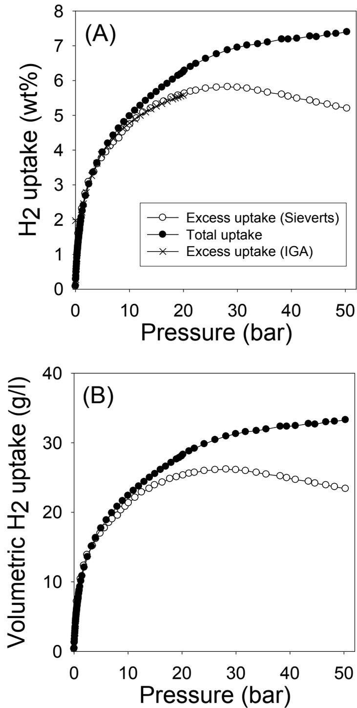
**Supporting Figure S3.** Gravimetric (A) and volumetric (B) excess and total hydrogen uptake isotherms at -196 °C and up to 50 bar for a representative zeolite templated carbon. The gravimetric hydrogen uptake obtained from IGA measurements is shown in (A).
