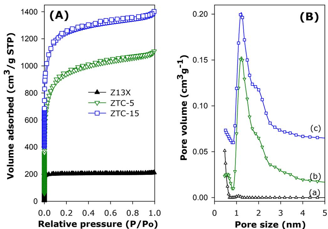
**Supporting Figure S2.** Nitrogen sorption isotherms (A) and pore size distribution (PSD) curves (B) for (a) zeolite 13X, and zeolite-templated carbons (b) ZTC-5 and (c) ZTC-15. For clarity, the isotherm of ZTC-15 is offset (y-axis) by 400 cm<sup>3</sup>/g, and the PSD curves (b) and (c) are offset (y-axis) by 0.01 and 0.06 cm<sup>3</sup>/g respectively.
