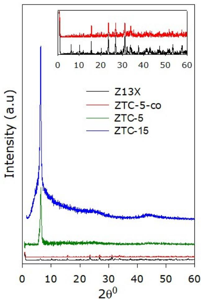
**Supporting Figure S1.** Powder XRD patterns of zeolite templated carbons (ZTC-5 and ZTC-15) prepared at variable heating ramp rate (5 and 15 °C/min, respectively). Patterns for the zeolite/carbon composite (ZTC-5-co) and zeolite 13X (Z13X) are also shown.
