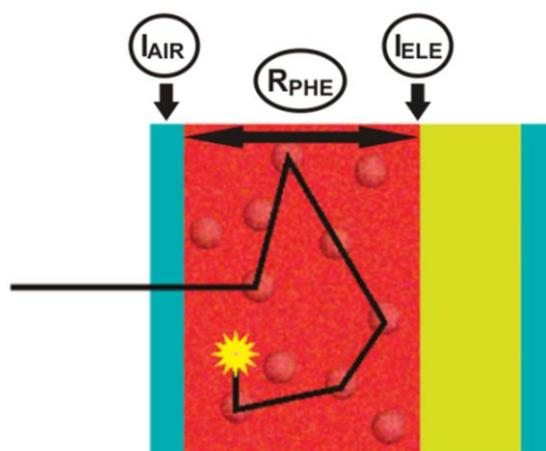
Scheme S1. A representation of the simulated DSC, in which the air-TCO entrance interface ( $I_{AIR}$ ) and the exit photoelectrode-electrolyte interface ( $I_{ELE}$ ) are considered. In between, the active photoelectrode region, composed of a dye sensitized nanocrystalline titania film with embedded scattering particles ( $R_{PHE}$ ).
