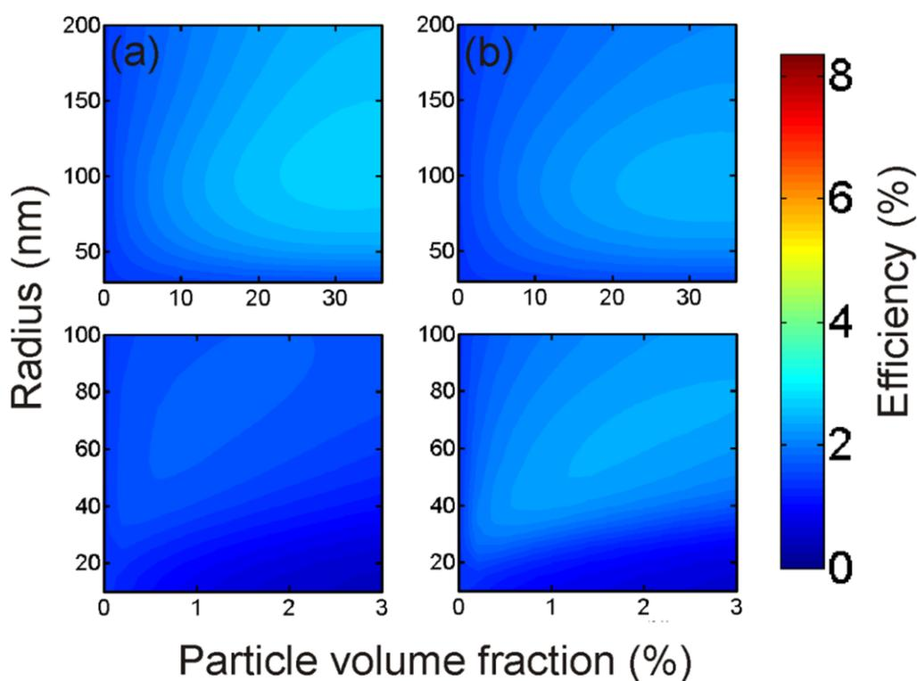
Figure S3. Power conversion efficiency versus sphere radius and volume fraction for electrodes of 1 micron thick electrodes including (a) titania, (b) electrolyte filled cavities, (c) gold, and (d) silver particles.
