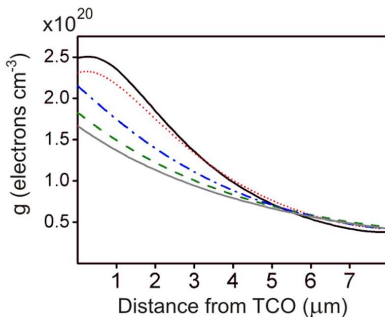
Figure S1. Examples of calculated electron generation rates for 8 micron thick dye sensitized electrodes with no scattering centres (gray solid line), containing anatase scattering particles (black solid line), electrolyte filled cavities (red dotted line), silver particles (blue dashed dotted line), and gold particles (green dashed line). In each case, particle size and concentration is that that optimizes the cell performance.
