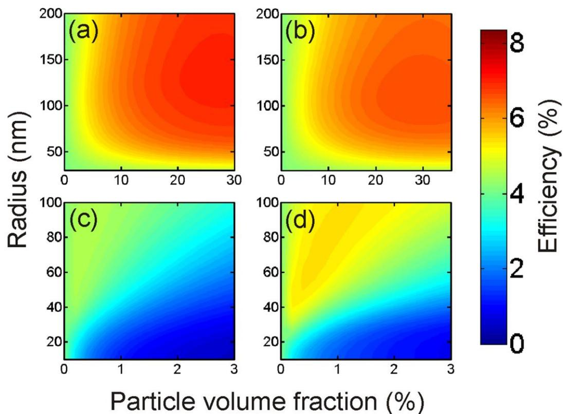
Figure S5. Power conversion efficiency versus sphere radius and volume fraction for electrodes of 4 micron thick electrodes including (a) titania, (b) electrolyte filled cavities, (c) gold, and (d) silver particles.
