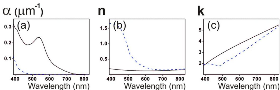
Figure S2. Optical constants employed in the calculations for the different materials considered. (a) Absorption coefficients for dye filling DSC porous (continuous line) and bulk electrolyte (dashed line); (b) real and (c) imaginary parts of the refractive index of silver (solid line) and gold (dashed line).
