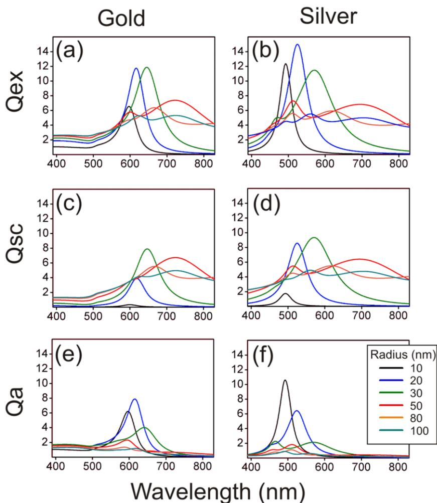
Figure S6. From top to bottom, extinction (total), scattering and absorption cross sections for (a) silver and (b) gold particles as a function of wavelength. Different particle radius are considered, as indicated in the legend.
