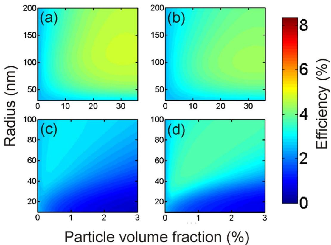
Figure S4. Power conversion efficiency versus sphere radius and volume fraction for electrodes of 2 micron thick electrodes including (a) titania, (b) electrolyte filled cavities, (c) gold, and (d) silver particles.
