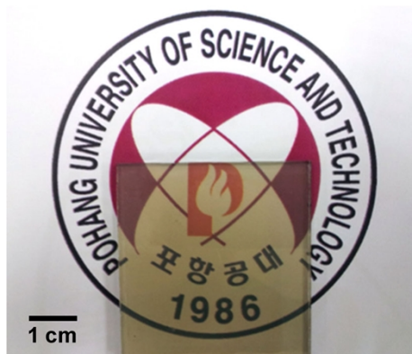
Figure S5. Photograph of the ZnCr:MMO/FTO glass fabricated by the Cr nitrate solution-dipping process followed by calcination at 527°C in air for 2 h.
