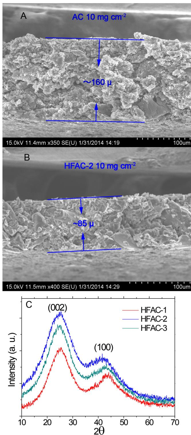
**Figure S1.** SEM images of AC (A) and HFAC-2 (B) electrode pressed at 100 MP; (C) X-Ray diffraction patterns of HFAC carbons.
