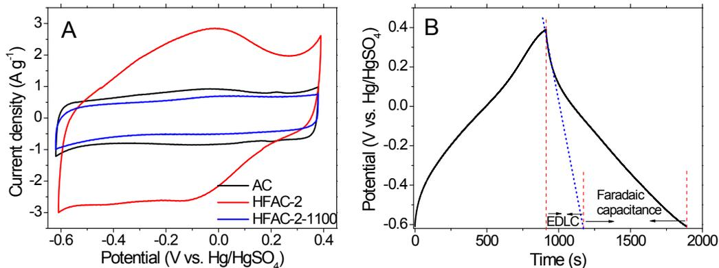
**Figure S5.** (A) Cyclic voltammograms (CVs) of HFAC-2 before and after an 1100°C anneal in Ar to eliminate the functional groups, AC being included as a baseline; (B) galvanostatic charge/discharge curve of HFAC-2 at 0.5 A g<sup>-1</sup> with the estimated EDLC and faradaic capacitance contributions being obtained from the discharge portions of differing slope. Testing was done in 1M H<sub>2</sub>SO<sub>4</sub> at 5mV/S.
