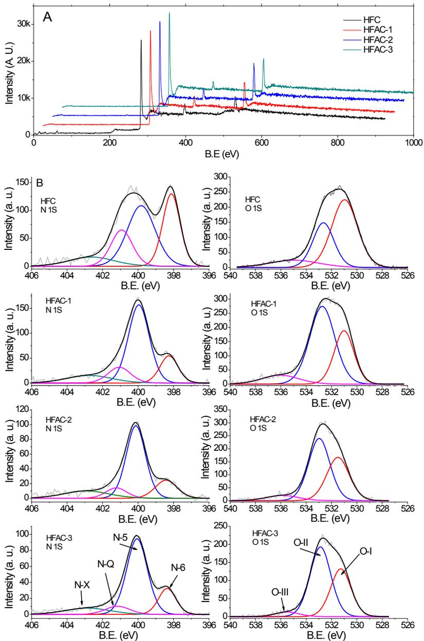
**Figure S2.** XPS spectra of HFAC materials. (A) XPS survey from 0 to 1000 eV; (B) N 1S and O 1S core level XPS spectra fitting.
