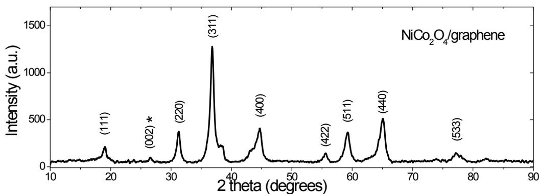
**Figure S8.** X-Ray diffraction pattern of NiCo<sub>2</sub>O<sub>4</sub>/graphene nanocomposite used as positive electrode in the asymmetric cell. The diffraction peak marked with \* is indexed as (002) graphitic peak associated with the graphene nanoflakes, while the other peaks are indexed as equilibrium NiCo<sub>2</sub>O<sub>4</sub>.
