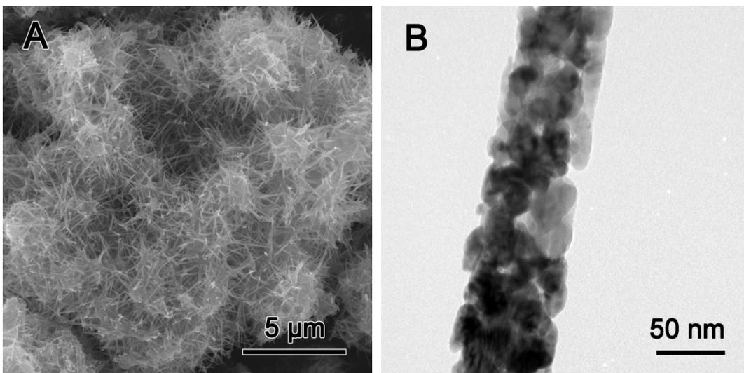
**Figure S7.** (A) SEM and (B) TEM micrographs of the NiCo<sub>2</sub>O<sub>4</sub>/graphene nanocomposite used as positive electrode in the asymmetric cell. Figure (B) shows a bright field image of a representative "nano-needle" of NiCo<sub>2</sub>O<sub>4</sub> that is composed of 10-20 nm crystallites interspersed with mesoporosity.
