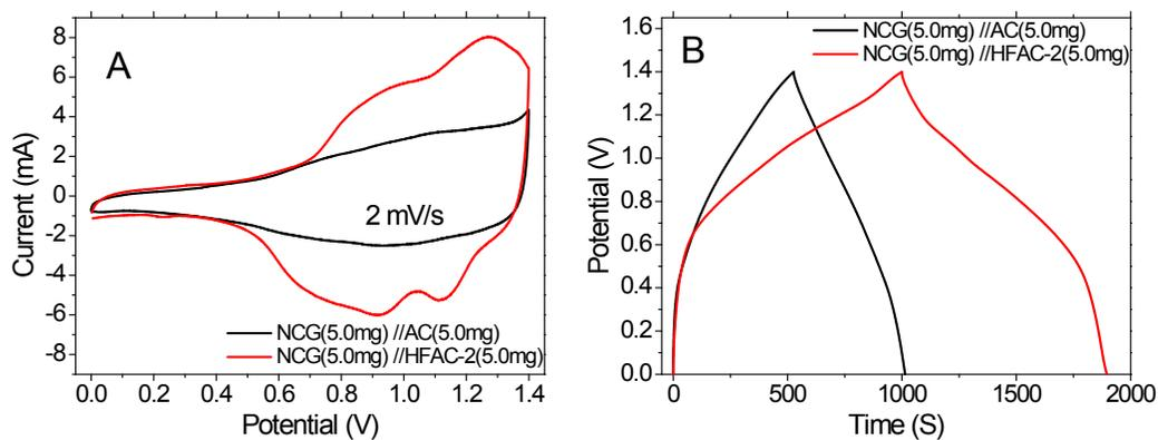
**Figure S9.** Comparative electrochemical performance of asymmetric supercapacitor cells, both of which employ 5 mg of the same positive electrode ( $\text{NiCo}_2\text{O}_4/\text{graphene}$ ), but with a different negative electrode (5 mg HFAC-2 vs. 5 mg AC). (A) CVs of the two asymmetric full cells; (B) galvanostatic charge/discharge curves of the two asymmetric cells at  $0.25 \text{ A g}^{-1}$ .
