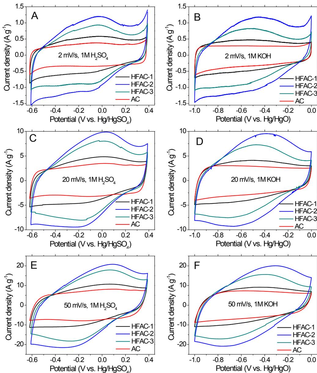
**Figure S3.** Cyclic voltammograms (CVs) of HFAC and of the baseline AC in 1M H<sub>2</sub>SO<sub>4</sub> (A, C, E) and in 1M KOH (B, D, F) at 2, 20 and 50 mV s<sup>-1</sup>.
