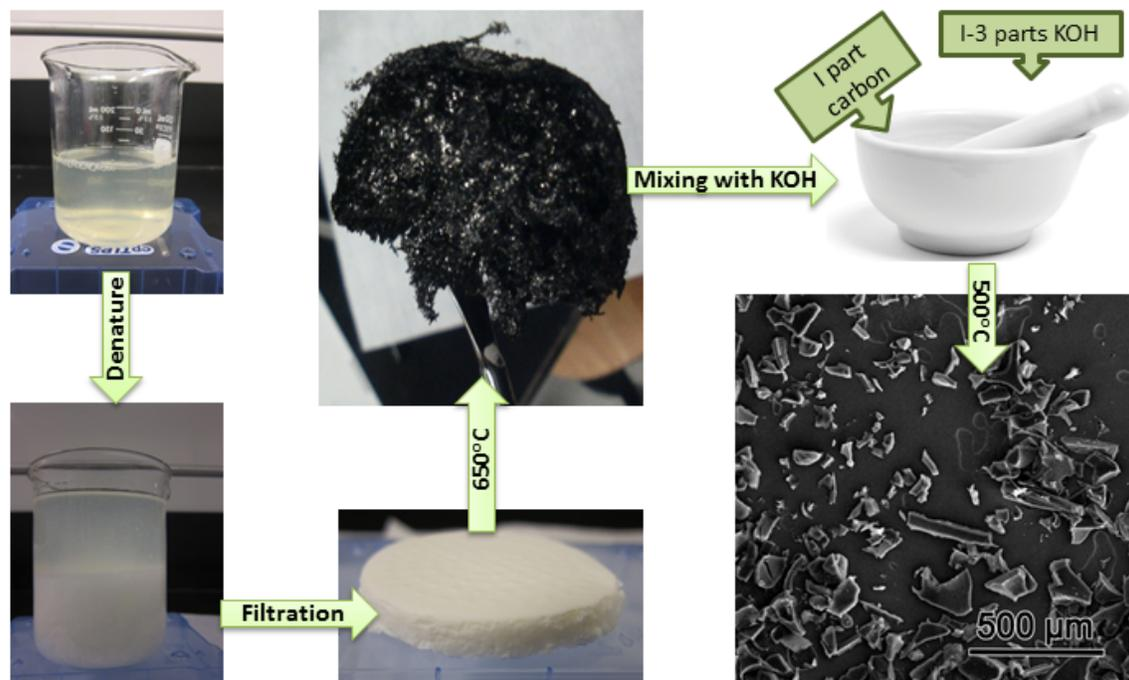
**Scheme S1.** Preparation process for highly functionalized activated carbons (HFAC).
