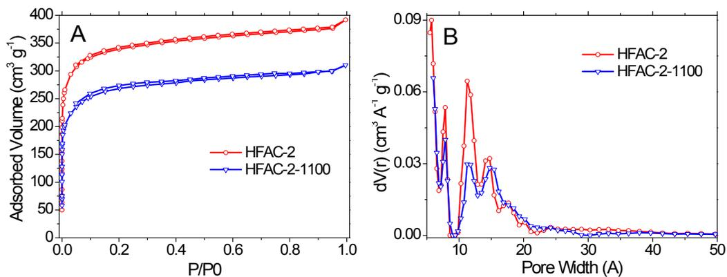
**Figure S4.** (A) Nitrogen adsorption isotherms at 77k and (B) NLDFT pore-size distribution of HFAC-2 before and after an 1100°C anneal in Ar to eliminate the functional groups.
