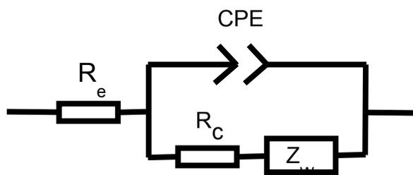
**Figure S6.** Corresponding equivalent circuit used for Nyquist plot simulation, where  $R_e$  is the total resistance of electrolyte, electrode, current collector and separator,  $R_{ct}$  is the charge transfer resistance,  $Z_w$  is the Warburg impedance related to the diffusion of ions into the bulk electrode, CPE stands for constant phase element related to the capacitive behavior of electrodes.
