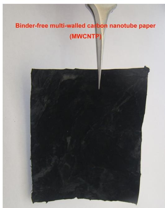
**Fig. S1** Photograph of a free-standing MWCNTP.
