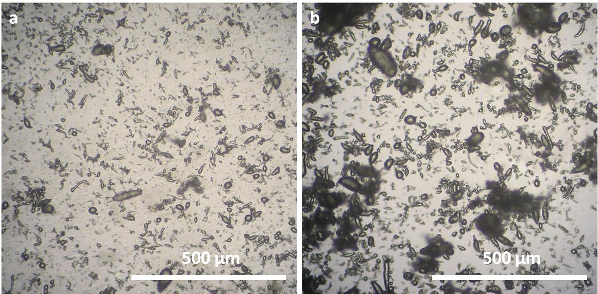
**Figure S2.4** Microscope images of **DryPEI(750k)** (a) before and (b) after CO<sub>2</sub> absorption
