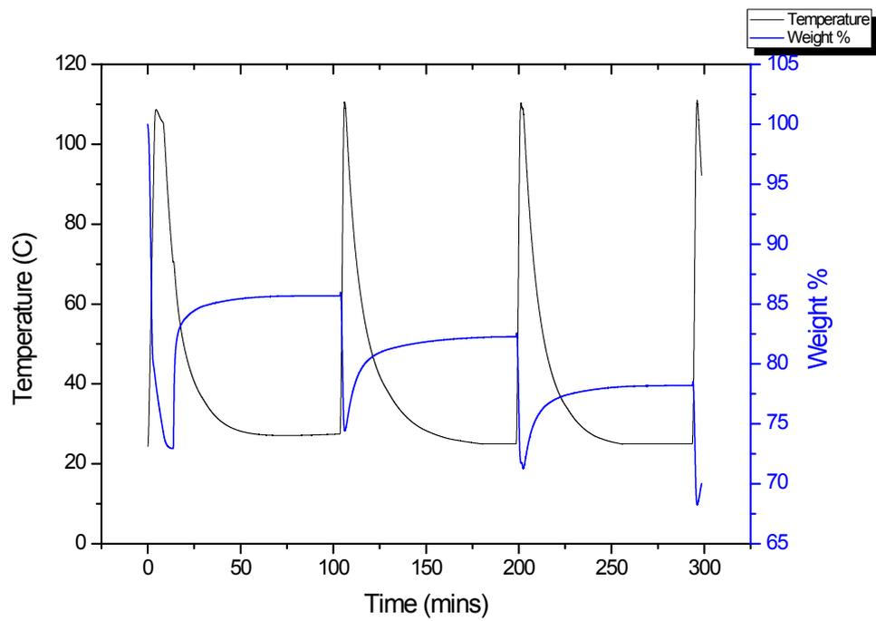
**Figure S4.5** Cycling of absorption of CO<sub>2</sub> at 25 °C by DryDEA and regeneration at 100 °C
