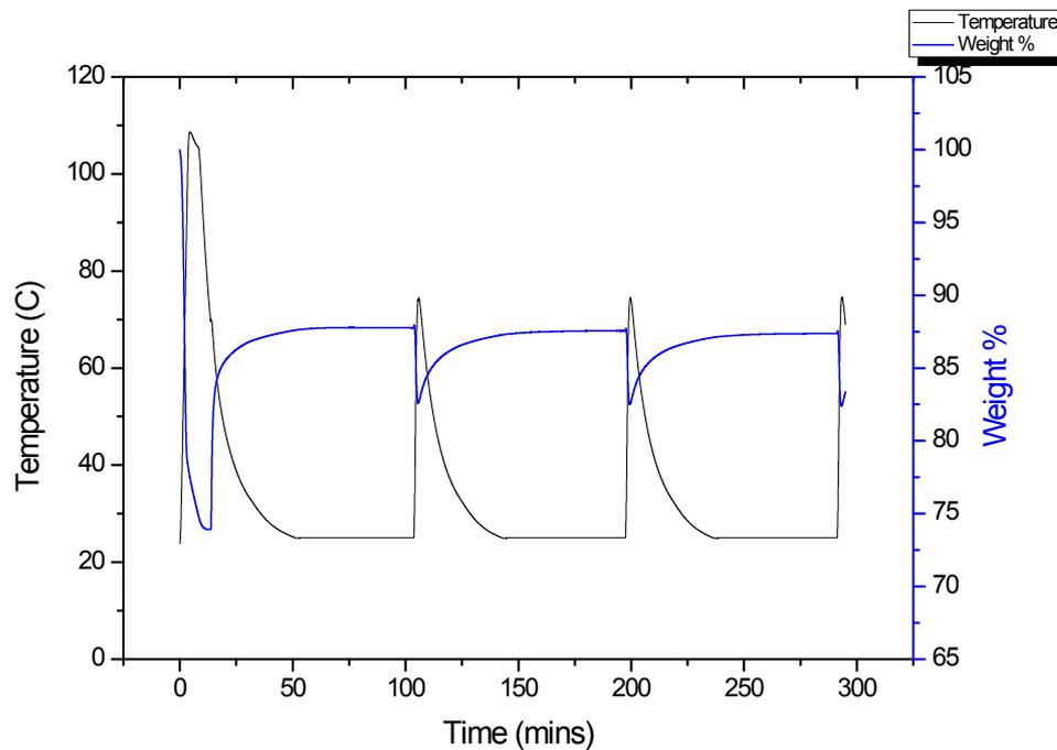
**Figure S4.2** Cycling of absorption of CO<sub>2</sub> at 25 °C by DryDEA and regeneration at 70 °C
