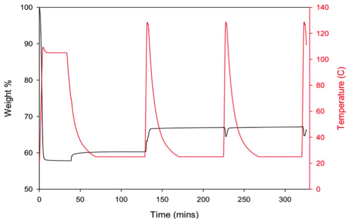
**Figure S5.1** Cycling of absorption of CO<sub>2</sub> at 25 °C by DryPEI and regeneration at 120 °C
