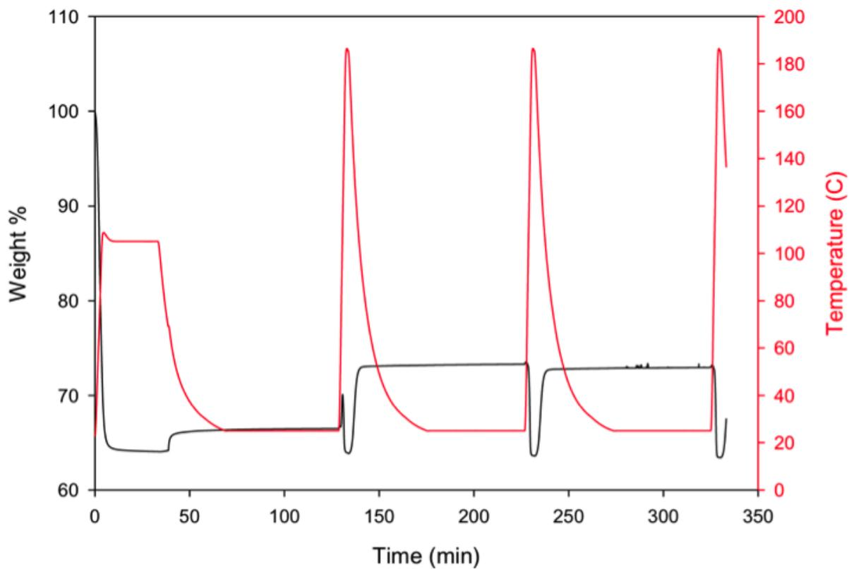
**Figure S5.4** Reg Cycling of absorption of CO<sub>2</sub> at 25 °C by DryPEI and regeneration at 180 °C
