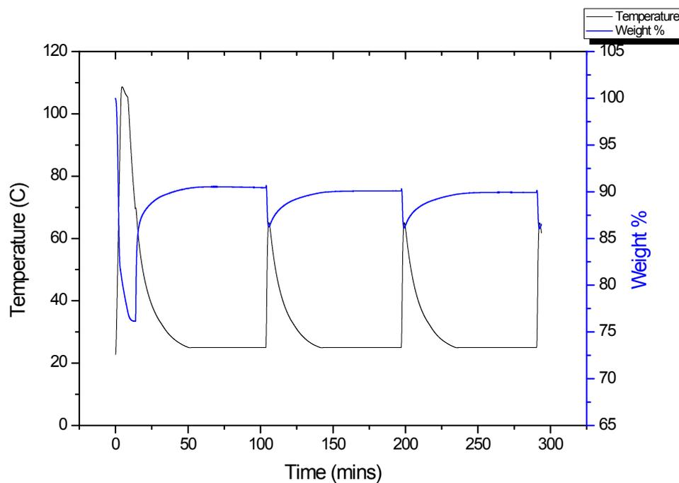
**Figure S4.1** Cycling of absorption of CO<sub>2</sub> at 25 °C by DryDEA and regeneration at 60 °C
