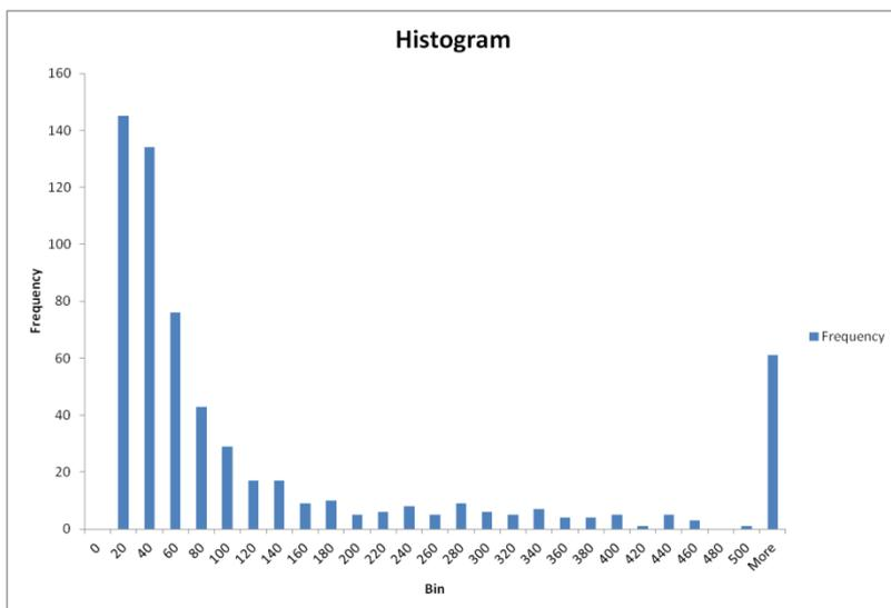
**Figure S2.6** Histogram showing particle sizes of **DryK<sub>2</sub>CO<sub>3</sub>(30)** before CO<sub>2</sub> capture. Data extracted by image analysis using ImageJ software from microscope images.
