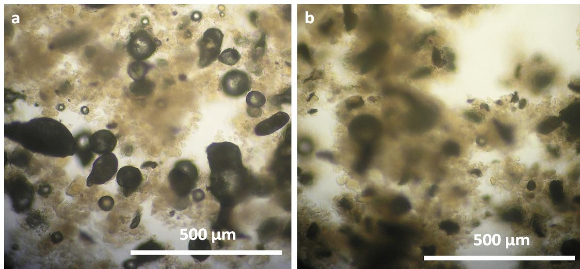
**Figure S2.1** Microscope images of **DryDEA** (a) before and (b) after CO<sub>2</sub> absorption
