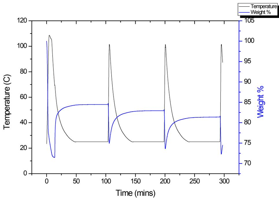
**Figure S4.4** Cycling of absorption of CO<sub>2</sub> at 25 °C by DryDEA and regeneration at 90 °C
