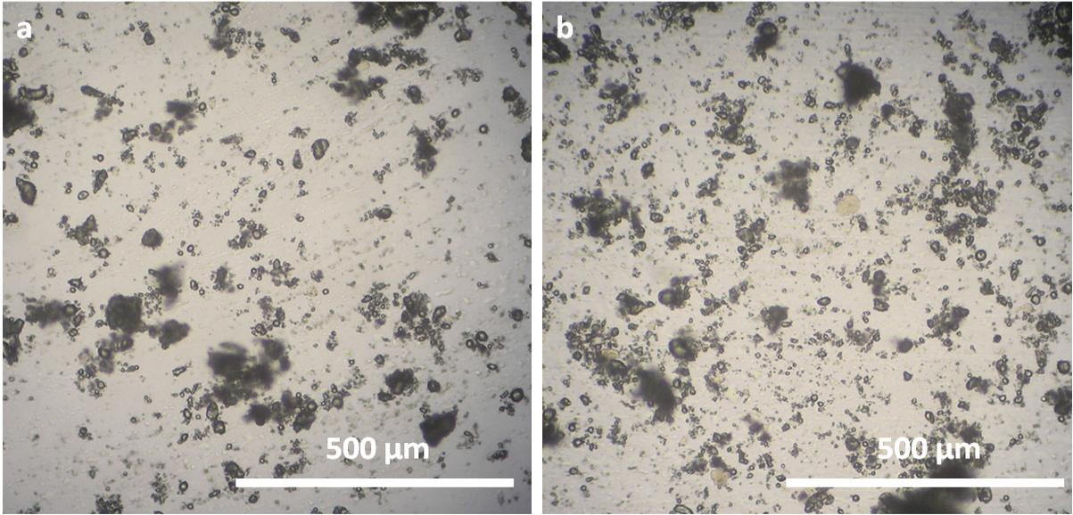
**Figure S2.3** Microscope images of **DryK<sub>2</sub>CO<sub>3</sub>(30)** (a) before and (b) after CO<sub>2</sub> absorption
