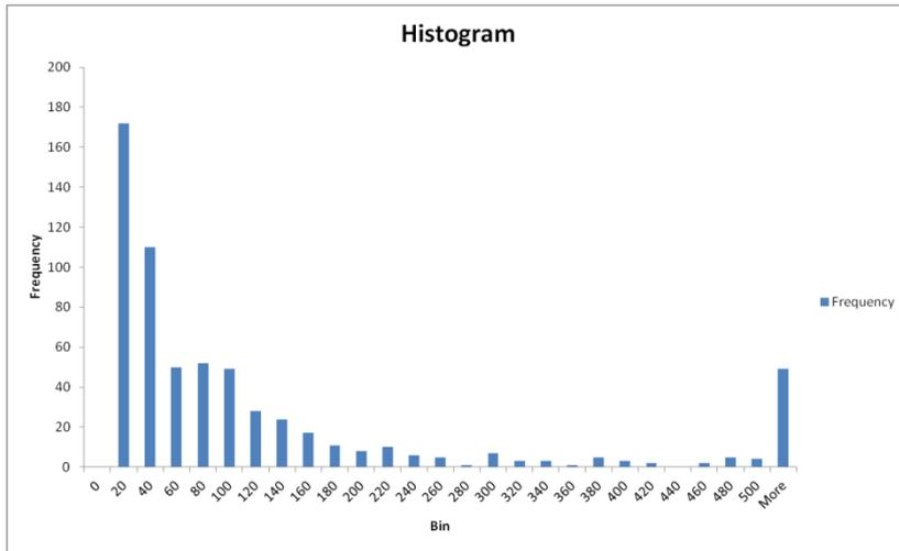
**Figure S2.8** Histogram showing particle sizes of **DryK<sub>2</sub>CO<sub>3</sub>(45)** before CO<sub>2</sub> capture. Data extracted by image analysis using ImageJ software from microscope images.
