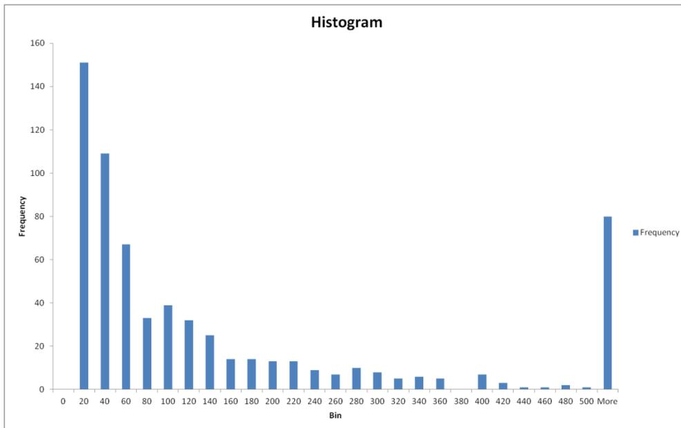
**Figure S2.8** Histogram showing particle sizes of **DryK<sub>2</sub>CO<sub>3</sub>(30)** after CO<sub>2</sub> capture. Data extracted by image analysis using ImageJ software from microscope images.
