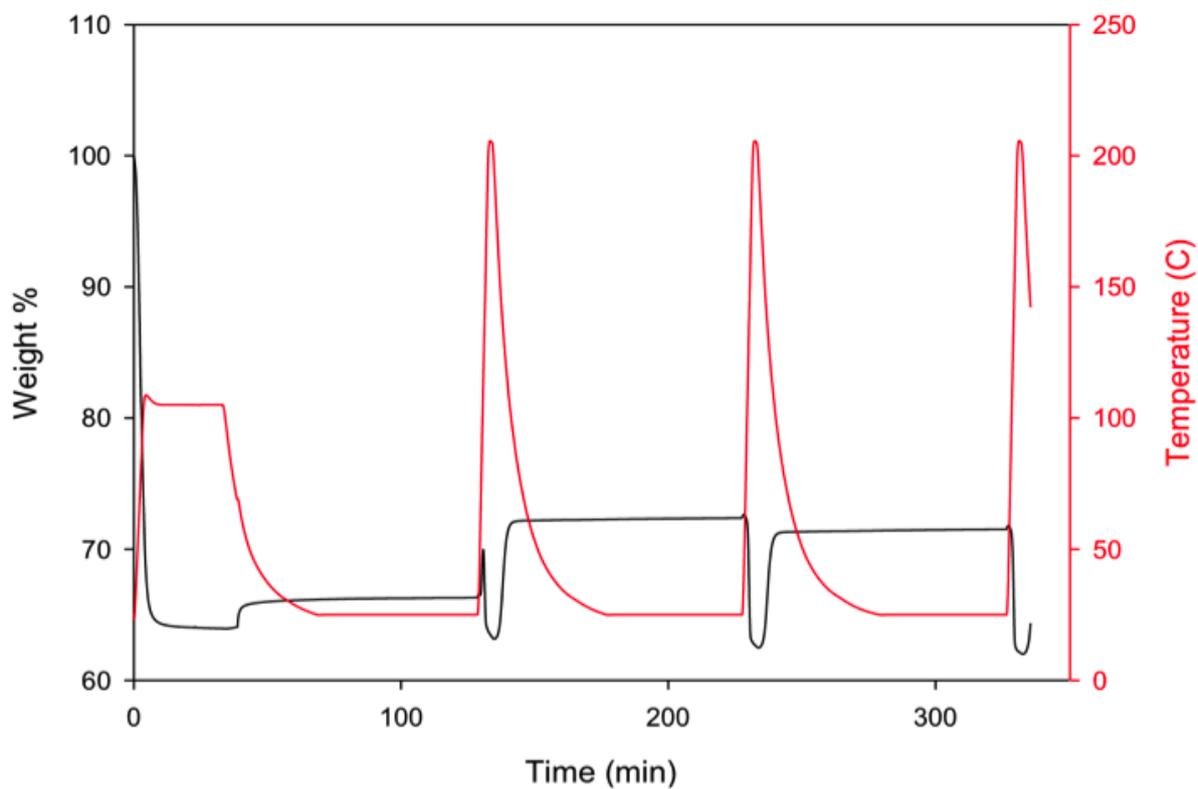
**Figure S5.5** Cycling of absorption of CO<sub>2</sub> at 25 °C by DryPEI and regeneration at 200 °C
