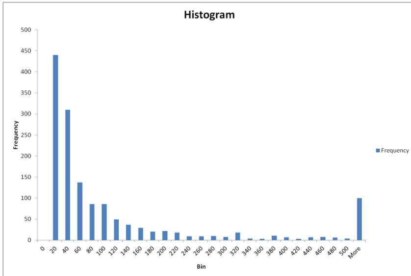
**Figure S2.9** Histogram showing particle sizes of **DryPEI** before CO<sub>2</sub> capture. Data extracted by image analysis using ImageJ software from microscope images.
