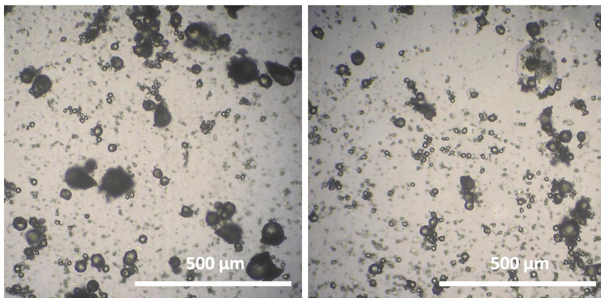
**Figure S2.2** Microscope images of **DryK<sub>2</sub>CO<sub>3</sub>(45)** (a) before and (b) after CO<sub>2</sub> absorption
