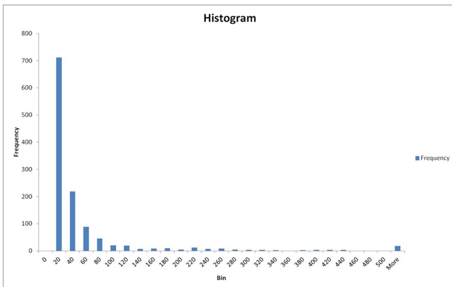
**Figure S2.5** Histogram showing particle sizes of **DryDEA** before CO<sub>2</sub> capture. Data extracted by image analysis using ImageJ software from microscope images.
