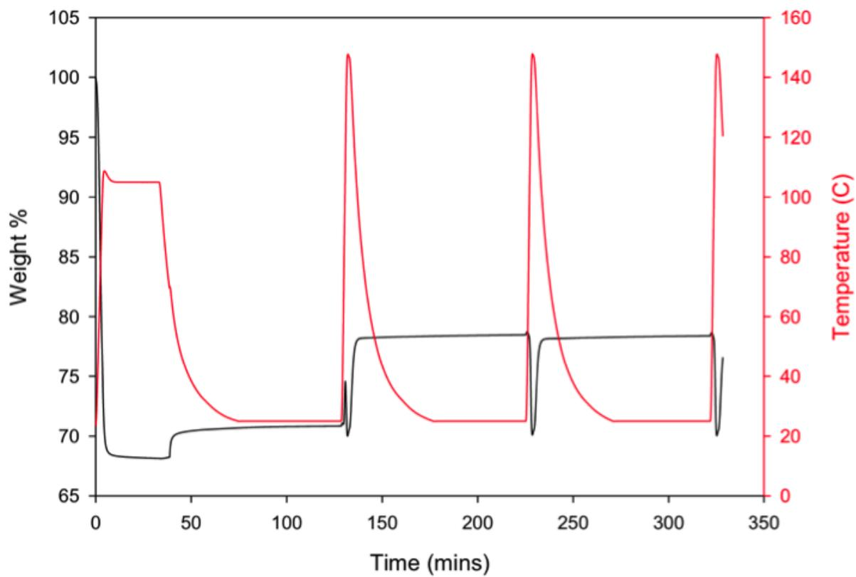
**Figure S5.2** Cycling of absorption of CO<sub>2</sub> at 25 °C by DryPEI and regeneration at 140 °C
