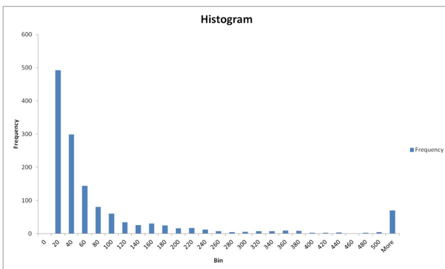
**Figure S2.7** Histogram showing particle sizes of **DryK<sub>2</sub>CO<sub>3</sub>(30)** after CO<sub>2</sub> capture. Data extracted by image analysis using ImageJ software from microscope images.
