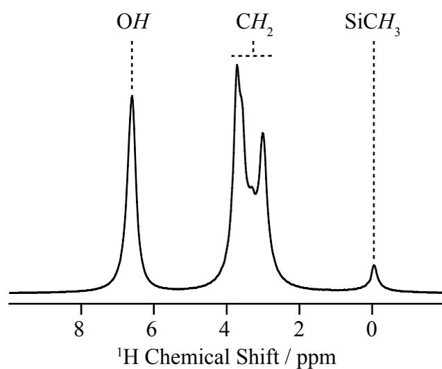
**Figure S6.1** Solid-state <sup>1</sup>H NMR spectrum of **DryDEA** post CO<sub>2</sub> adsorption. The chemical shifts are 6.6, 3.7-3.0 and -0.1 ppm and assigned to OH (either water or (OHCH<sub>2</sub>CH<sub>2</sub>)<sub>2</sub>NCO<sub>2</sub>H or (OHCH<sub>2</sub>CH<sub>2</sub>)<sub>2</sub>NH), CH<sub>2</sub> and SiCH<sub>3</sub> respectively.
