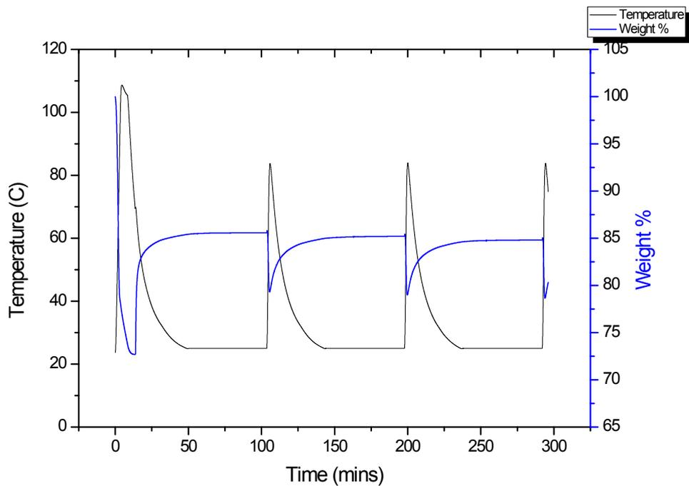
**Figure S4.3** Cycling of absorption of CO<sub>2</sub> at 25 °C by DryDEA and regeneration at 80 °C
