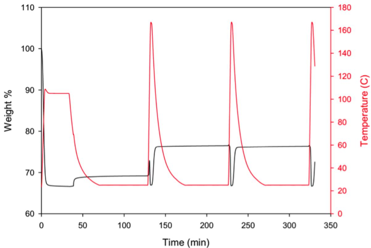
**Figure S5.3** Cycling of absorption of CO<sub>2</sub> at 25 °C by DryPEI and regeneration at 160 °C
