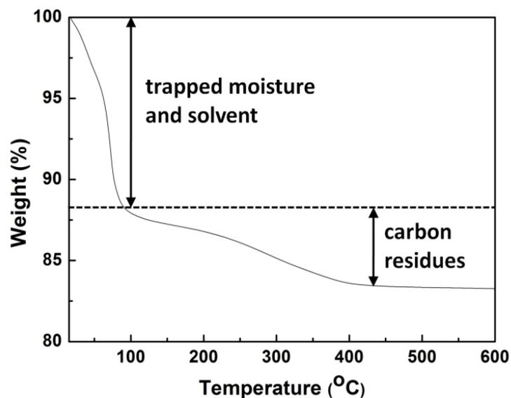
**Fig. S7** TGA curve of TiO<sub>2</sub> microspheres prepared at 200 °C for 12 h, using 2 ml of titanium isopropoxide in 60 ml anhydrous acetone.
