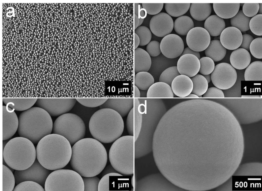
**Fig. S4** FESEM images of TiO<sub>2</sub> microspheres prepared at 200 °C for 12 h, using 4 ml of titanium isopropoxide.
