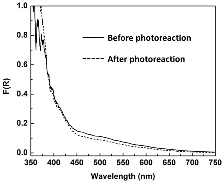
**Fig. S9** Diffuse reflectance spectra of TiO<sub>2</sub> microspheres prepared after annealing at 200 °C for 2 h before and after photoreaction for 12 h.
