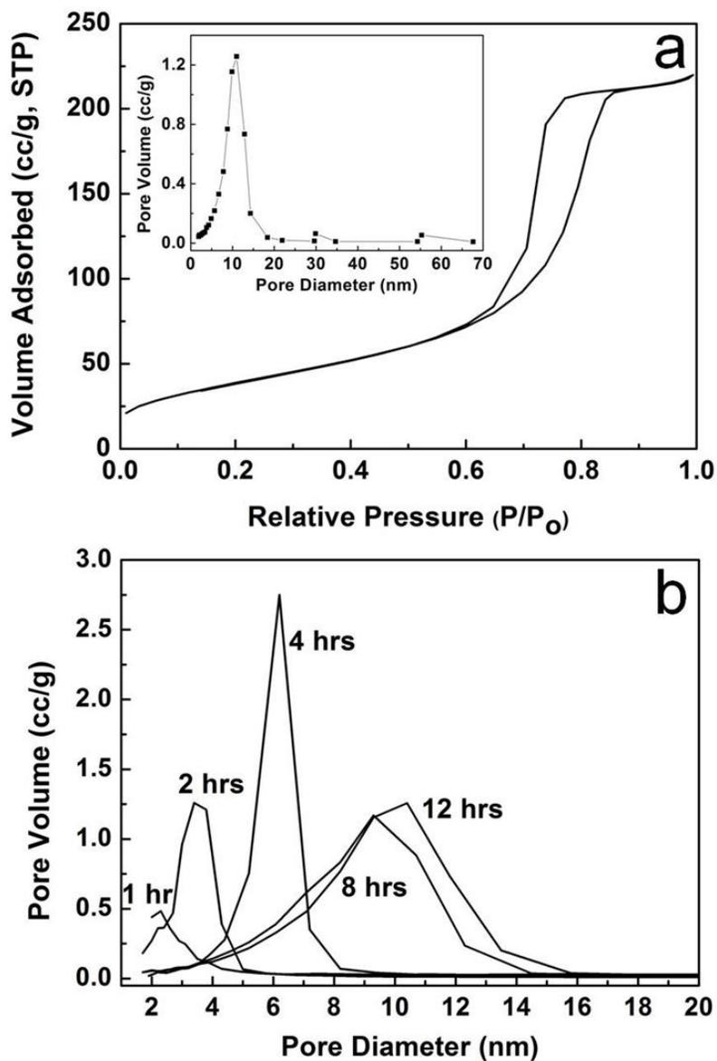
**Fig. S6** (a) Nitrogen adsorption-desorption isotherm of TiO<sub>2</sub> microspheres prepared at 200 °C for 12 h, using 2 ml of titanium isopropoxide in 60 ml anhydrous acetone. Inset is the corresponding BJH pore size distribution. (b) BJH pore size distribution of TiO<sub>2</sub> microspheres prepared at 200 °C for various solvothermal reaction times.
