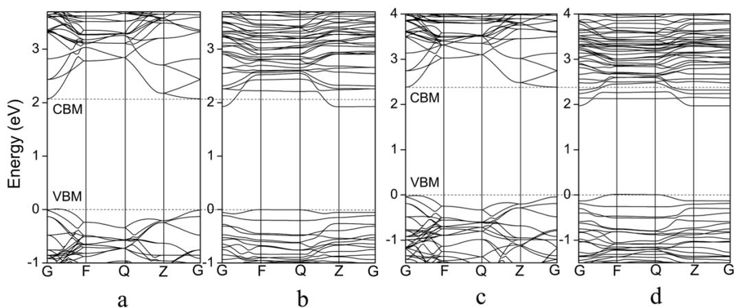
**Fig. S1** Band structures for undoped  $\text{TiO}_2$  (a and c) and carbonate-doped  $\text{TiO}_2$  (b and d). Band structures in a and b (c and d) are obtained by the PBE (PBE+U) calculations, respectively. All the energies of undoped  $\text{TiO}_2$  and carbonate-doped  $\text{TiO}_2$  are aligned by their valence band maxima (VBM). The dashed lines indicate the VBM and conduction band minimum (CBM) of undoped  $\text{TiO}_2$
