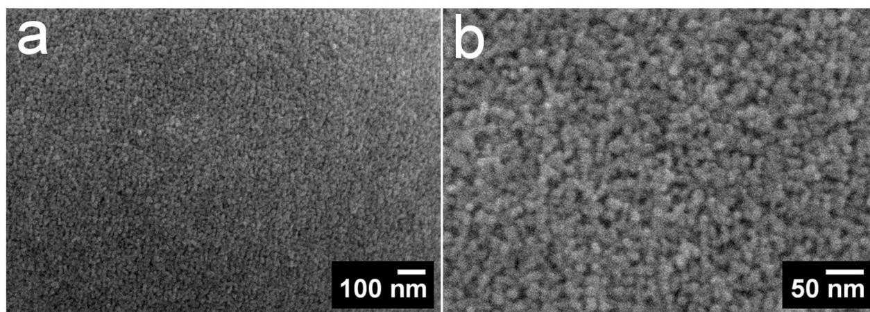
**Fig. S2** High-magnification FESEM images of  $\text{TiO}_2$  microspheres prepared at  $200\text{ }^\circ\text{C}$  for 12 h, using 2 ml of titanium isopropoxide.
