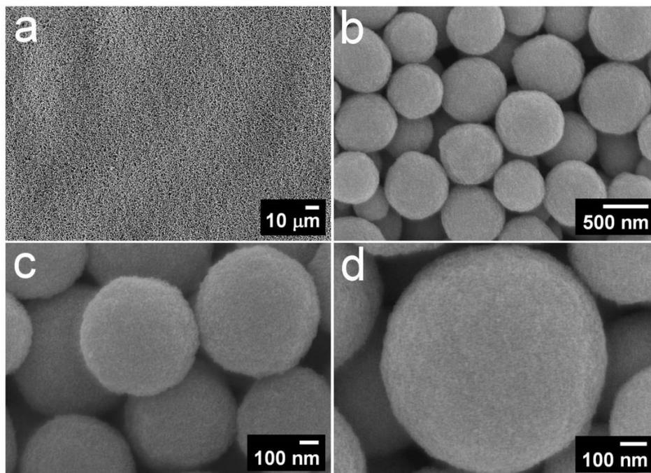
**Fig. S3** FESEM images of TiO<sub>2</sub> microspheres prepared at 200 °C for 12 h, using 1 ml of titanium isopropoxide.
