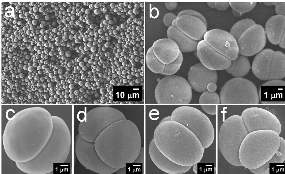
**Fig. S5** FESEM images of  $\text{TiO}_2$  multimers prepared at 200 °C for 12 h, using 8 ml of titanium isopropoxide.
