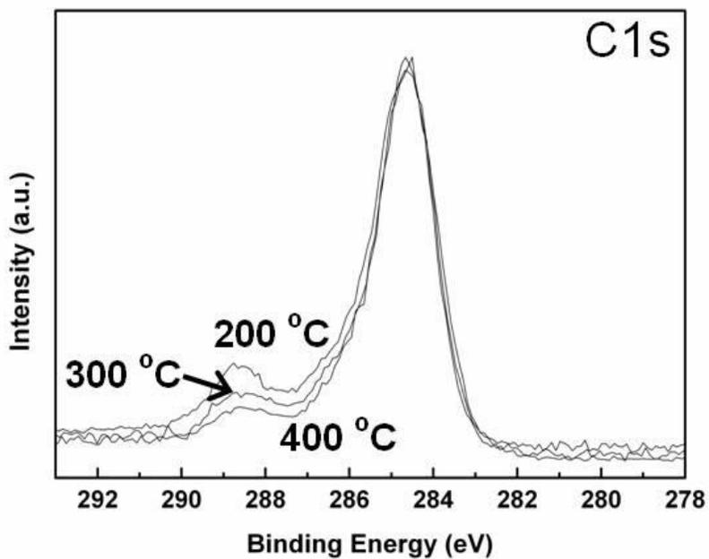
**Fig. S8** XPS spectra of C1s band for TiO<sub>2</sub> microspheres prepared at various calcination temperatures.
