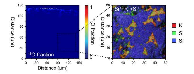
**Figure S2.** Map of the <sup>18</sup>O isotopic fraction (left) in a cross-sectional area post exchange. The inhomogeneity of the tracer diffusion front can be seen to be on the same scale as the chemical inhomogeneity mapped on the right (taken from Figure 5).
