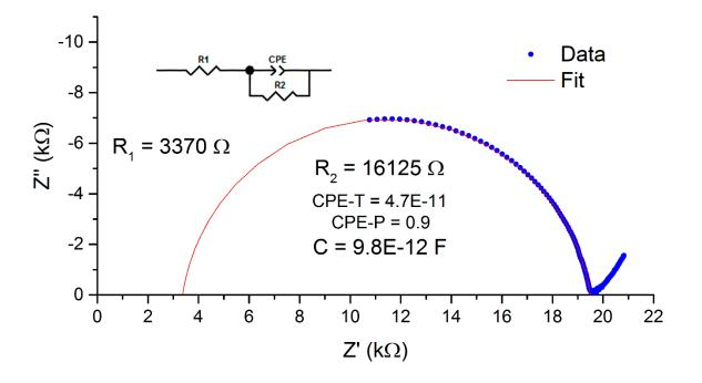
Figure S1. Example impedance spectra for the SKSG sample at ~ 415 °C.
