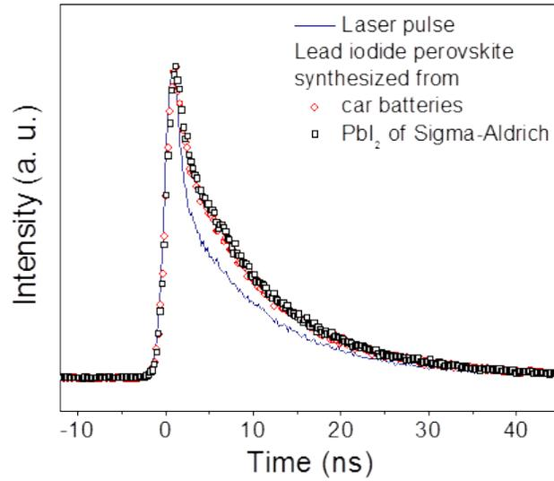
**Fig. S2** PL response of perovskite films. Normalized time resolved photoluminescence intensity from the lead iodide perovskite films synthesized from car batteries and commercial  $\text{PbI}_2$  powder (Sigma-Aldrich, #211168, >99.0%). The excitation laser pulse profile is shown in solid blue line. All samples exhibit a single exponential relaxation process with the same lifetime of  $1.00 \pm 0.09$  ns.
