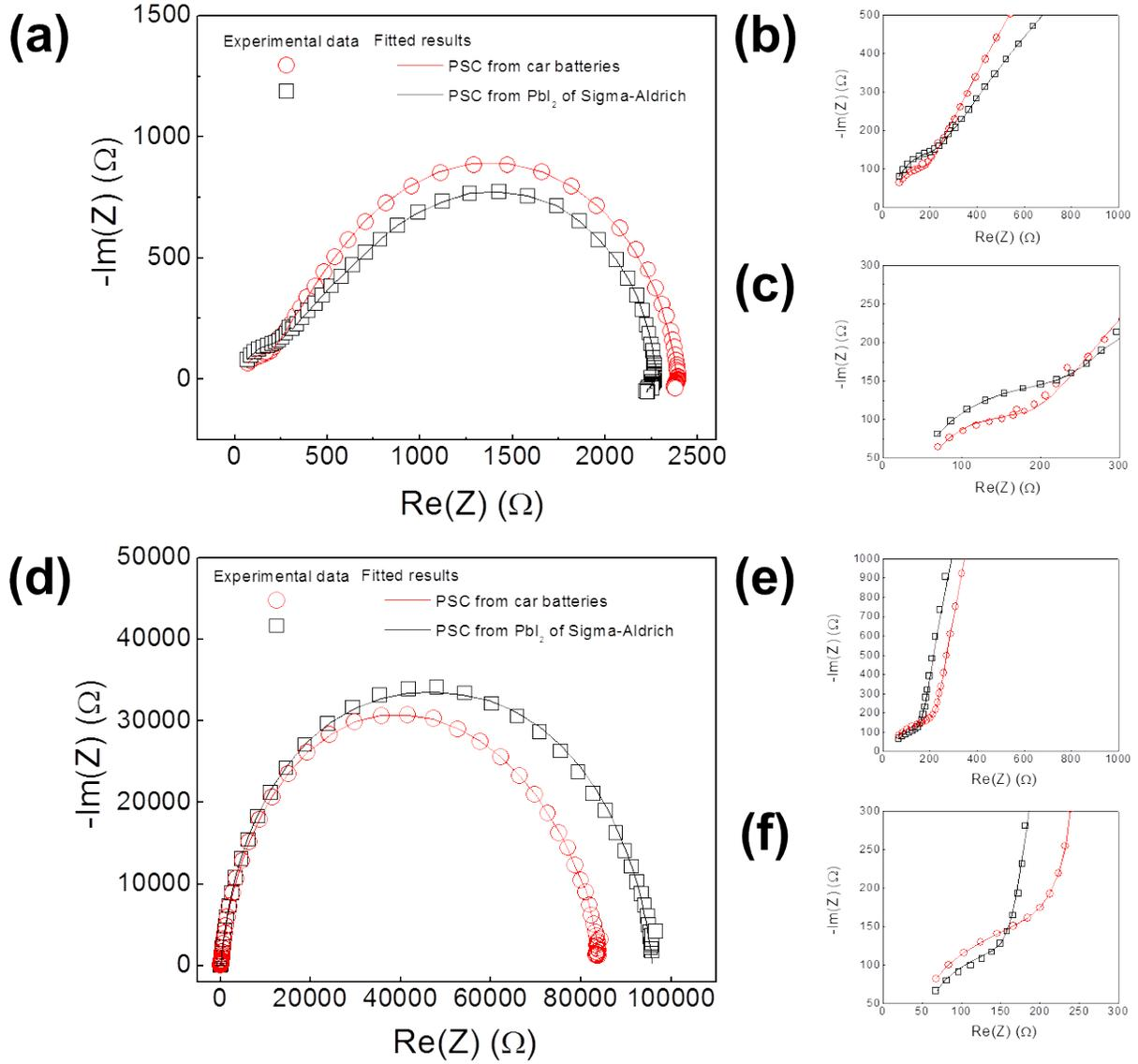
**Fig. S4** Nyquist diagrams of PSCs fabricated from car batteries and high-purity commercial  $\text{PbI}_2$ . (a)-(c) and (d)-(e) are the Nyquist diagrams corresponding to the
