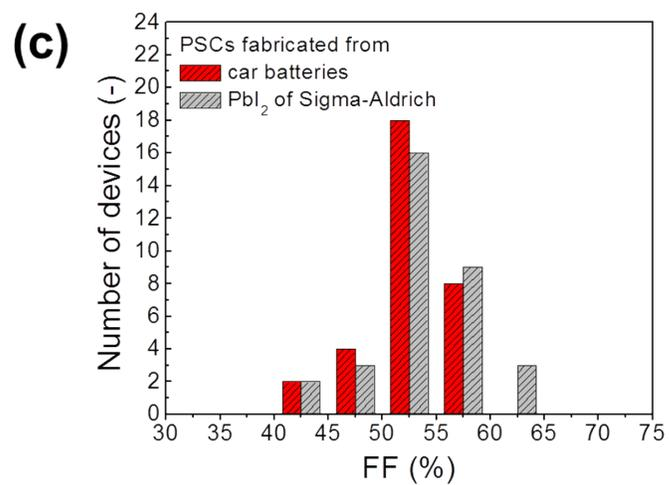
**Fig. S3** Static data of photovoltaic performance of PSCs fabricated from car batteries and high-purity  $\text{PbI}_2$ . Histogram plots of solar cell performance parameters: (a)  $V_{OC}$ , (b)  $J_{SC}$ , and (c) FF from multiple batches of  $\text{CH}_3\text{NH}_3\text{PbI}_3$ -sensitized  $\text{TiO}_2$  photovoltaic devices (total of 65 devices).
