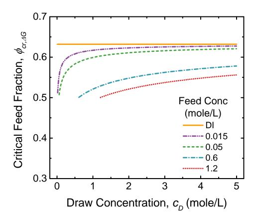
**Fig. S1.** The critical feed fraction,  $\phi_{cr,\Delta G}$ , (i.e. the feed fraction that maximizes the Gibbs free energy of mixing) as a function of draw solution NaCl concentration. The 0.015, 0.05, 0.6, and 1.2 M NaCl feed concentrations correspond to river water or waste water, brackish water, seawater, and brine, respectively. Deionized water (DI) is also shown as a potential feed solution.
