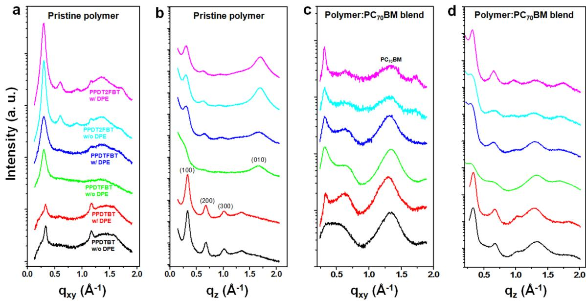
**Fig. S12** In-plane (a and c) and out-of-plane (b and d) GIWAXS data for pristine polymers (a and b) and polymer:PC<sub>70</sub>BM (c and d) films with and without DPE.
