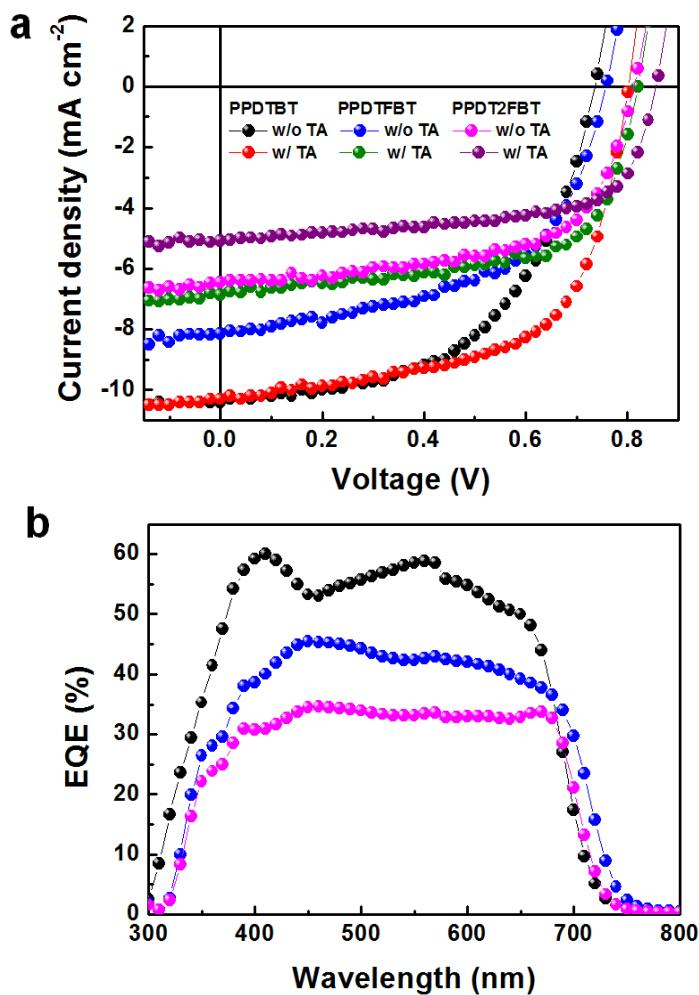
**Fig. S6** (a)  $J$ - $V$  characteristics (w/o TA: without thermal annealing, w/ TA: with thermal annealing) and (b) EQE of polymer:PC<sub>70</sub>BM PSCs prepared from a chlorobenzene solution without processing additives.
