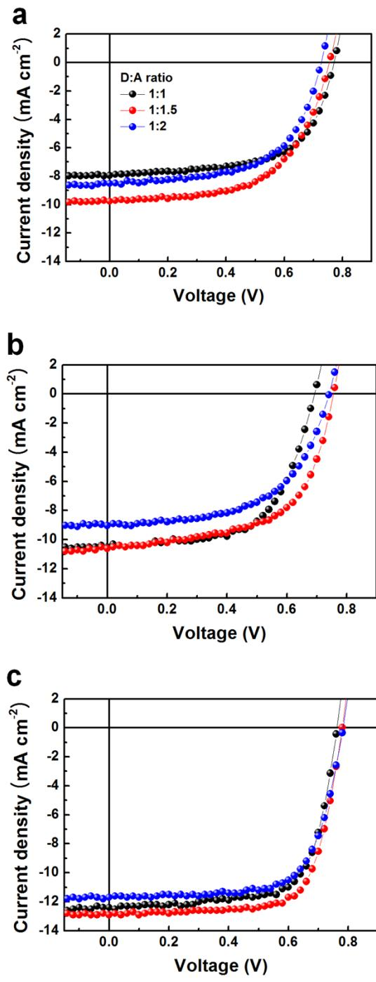
**Fig. S5** *J-V* characteristics of (a) PPDTBT, (b) PPDTFBT and (c) PPDT2FBT based PSCs with different polymer:PC<sub>70</sub>BM blend ratios (solvent: o-dichlorobenzene).
