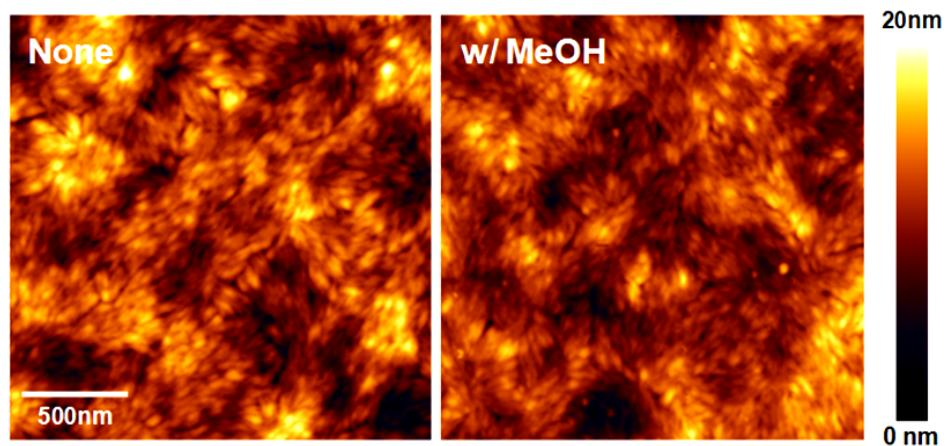
**Fig. S9** AFM topography images of PPDT2FBT:PC<sub>70</sub>BM without (left) and with (right) MeOH treatments. (solvent: CB:DPE, 98:2 vol%).
