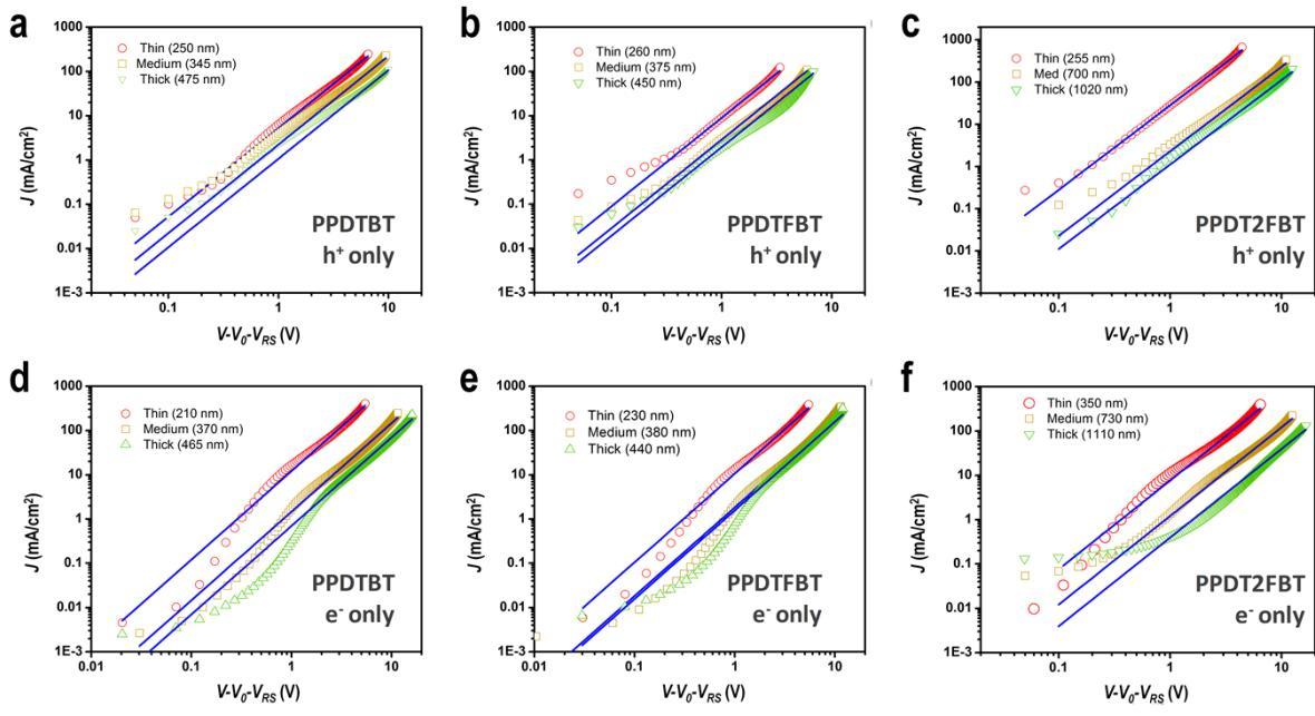
**Fig. S11** J-V characteristics of (a)~(c) hole-only and (d)~(f) electron-only devices based on polymer:PC<sub>70</sub>BM blend films with various film thickness (solvent: CB:DPE = 98:2 vol%). Blue lines represent fits of the curves using the Mott-Gurney relationship.
