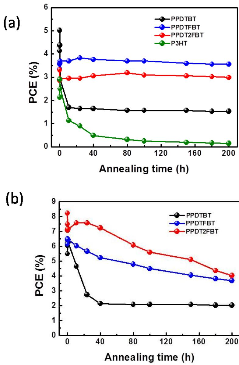
**Fig. S8** Temporal stability of polymer:PC<sub>70</sub>BM PSCs (a) without and (b) with DPE at an annealing temperature of 130 °C for 200 h (P3HT-based device for comparison). All devices were prepared from chlorobenzene.
