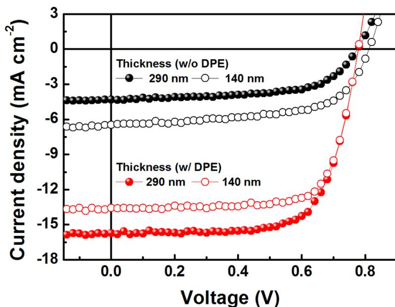
**Fig. S7**  $J$ - $V$  characteristics of PPDT2FBT:PC<sub>70</sub>BM PSCs with variable film thickness.
