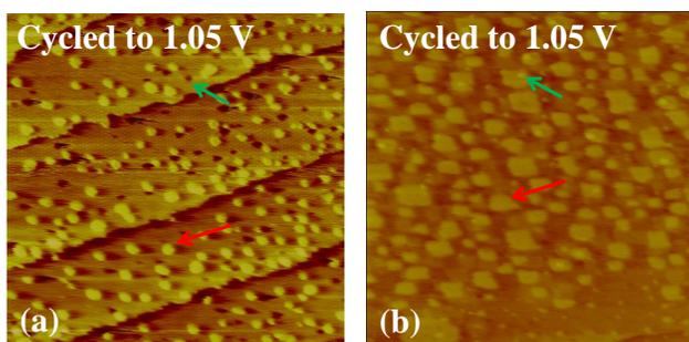
**Fig. S1** (a) STM images of Pt(111) after cycled to 1.05V, red arrow points out ad-island; green arrow points out hole. (a) STM image of Pt (100) after cycled to 1.05 V, additional ad-island is pointed out by the green arrow; red arrow indicates the loss of sharp corners from those square islands.
