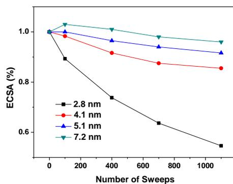
**Fig. S4** Changes of electrochemically active surface area (ECSA) during potential cycling between 0.6V and 1.1V at 50mV/s, 60°C in 0.1 M perchloric acid.
