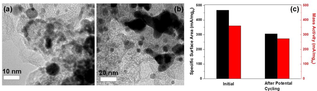
**Fig. S5** Mixed 2.8 nm and 7.2 nm catalyst suspension: TEM images (a) before and (b) after stability test, (c) Specific surface area (black) and ORR mass activity at 0.90V (Red) before and after stability test. Same stability test protocol was used. (i.e. 60°C, scan between 0.6V and 1.1V for 4000 sweeps at 50mV/s in 0.1M perchloric acid).
