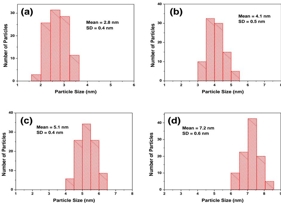
**Fig. S2** Histograms of the as-synthesized (a)  $2.8 \pm 0.4$  nm, (b)  $4.1 \pm 0.5$  nm, (c)  $5.1 \pm 0.4$  nm, (d)  $7.2 \pm 0.6$  nm Pt nanoparticles. 100 particles were counted for each of them.
