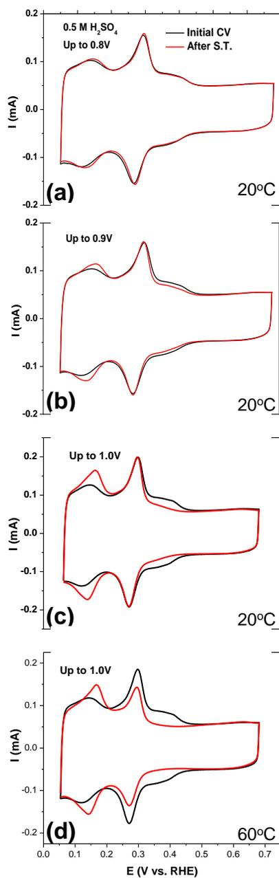
**Fig. S3** Cyclic voltammograms (CVs) of Pt nanocubes on carbon support before and after 4000 potential cyclings from 0.6V to (a) 0.8 V (b) 0. 9V (c) 1.0 V (d) 1.0 V. (a) to (c) were conducted at room temperature (20 °C). (d) was conducted at 60 °C. All the CVs were recorded in 0.5 M H<sub>2</sub>SO<sub>4</sub>. The potential cycling was conducted in 0.1 M HClO<sub>4</sub>.
