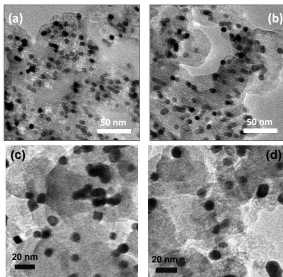
**Fig. S6** TEM images of nanocubes (a) before and (b) after stability test. TEM images of nano-octahedrons (c) before and (d) after stability test. Stability test protocol is the same as in Figure S5.
