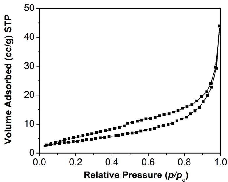
**Fig. S9** N<sub>2</sub> adsorption-desorption isotherm of as-prepared MoS<sub>2</sub> microparticles.
