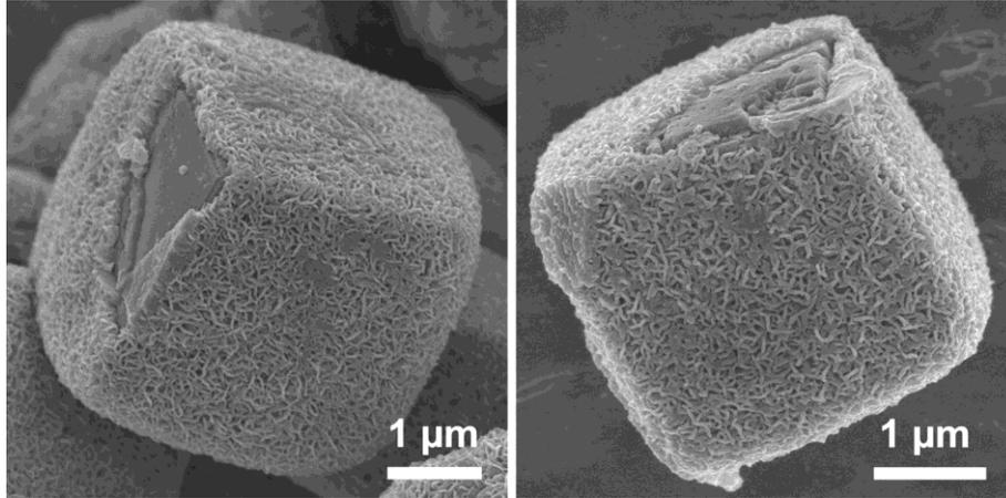
**Fig. S3** FESEM images of cracked MnS@MoS<sub>2</sub> core-shell microcubes with hierarchical shell structures.
