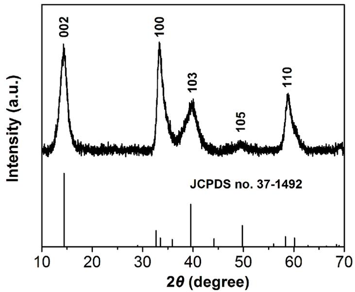
**Fig. S4** XRD pattern of annealed hierarchical MoS<sub>2</sub> microboxes.
