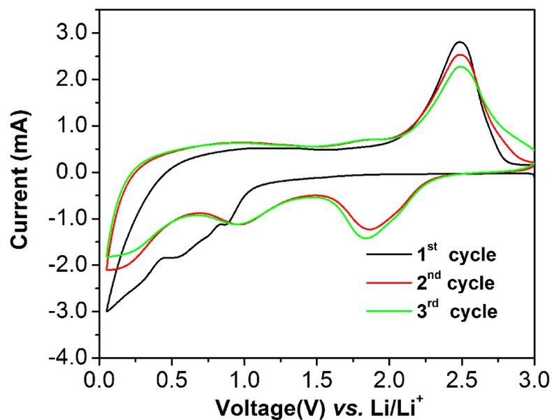
**Fig. S7** CV profiles of annealed hierarchical MoS<sub>2</sub> microboxes showing the 1<sup>st</sup>, 2<sup>nd</sup> and 3<sup>rd</sup> cycles between 0.05 and 3.0 V at a scan rate of 0.5 mV s<sup>-1</sup>.
