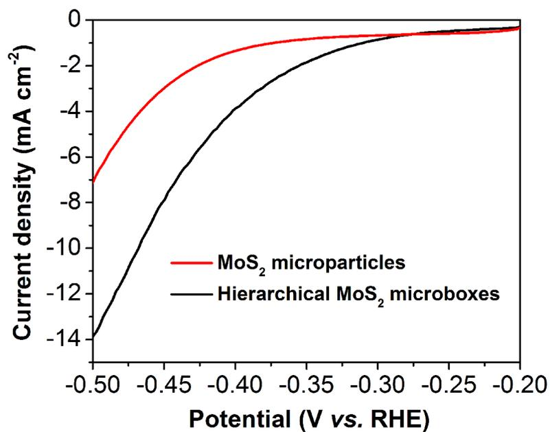
**Fig. S13** Polarization curves (the 500<sup>th</sup> cycle) of the as-prepared hierarchical MoS<sub>2</sub> microboxes and MoS<sub>2</sub> microparticles.
