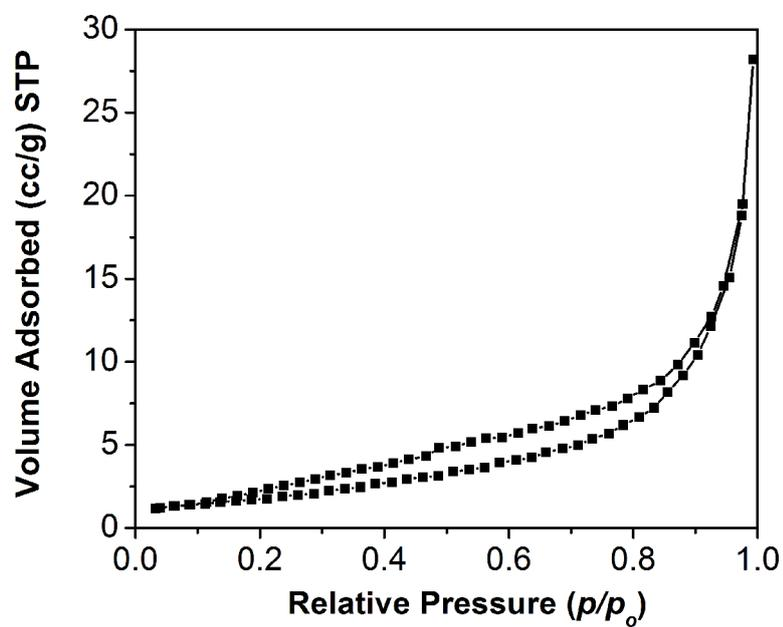
**Fig. S10** N<sub>2</sub> adsorption-desorption isotherm of annealed MoS<sub>2</sub> microparticles.
