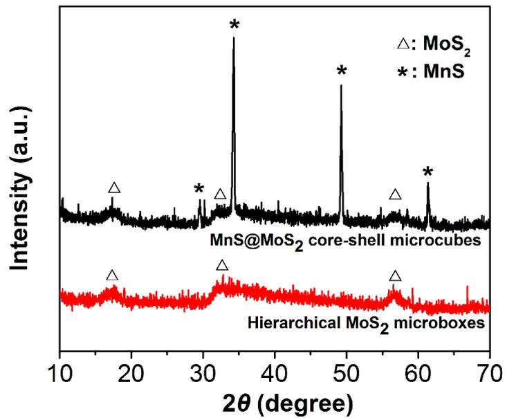
**Fig. S2** XRD patterns of as-prepared hierarchical MoS<sub>2</sub> microboxes and MnS@MoS<sub>2</sub> core-shell microcubes.
