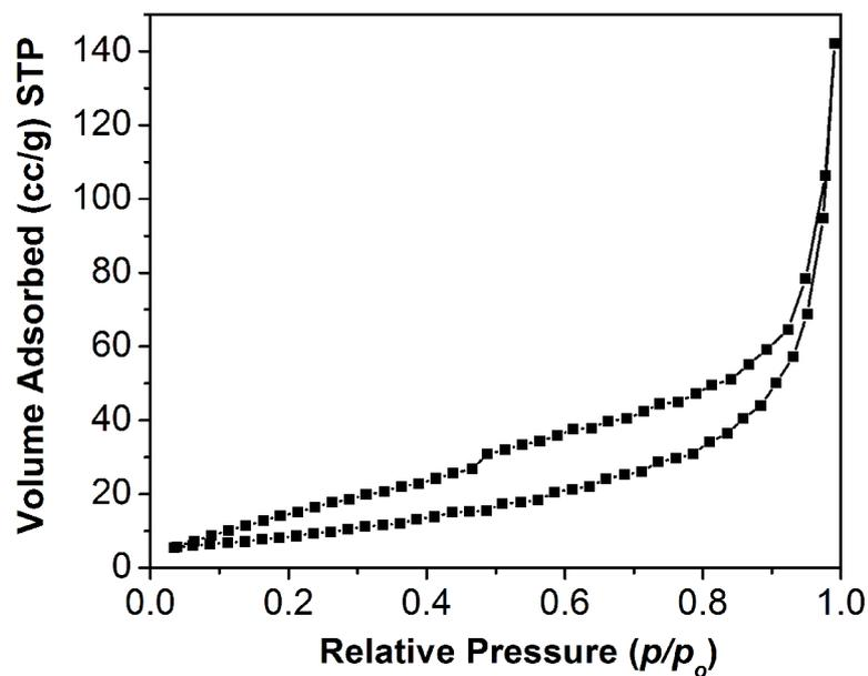
**Fig. S5** N<sub>2</sub> adsorption-desorption isotherm of as-prepared hierarchical MoS<sub>2</sub> microboxes.
