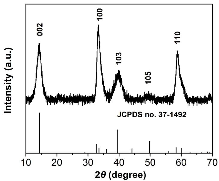
**Fig. S11** XRD pattern of annealed MoS<sub>2</sub> microparticles.
