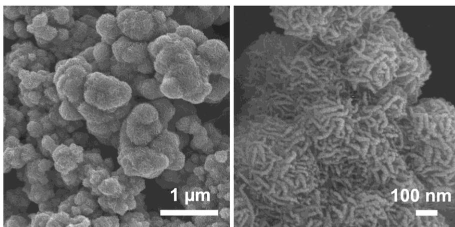
**Fig. S8** FESEM images of the MoS<sub>2</sub> microparticles obtained without adding MnCO<sub>3</sub> microcubes templates.
