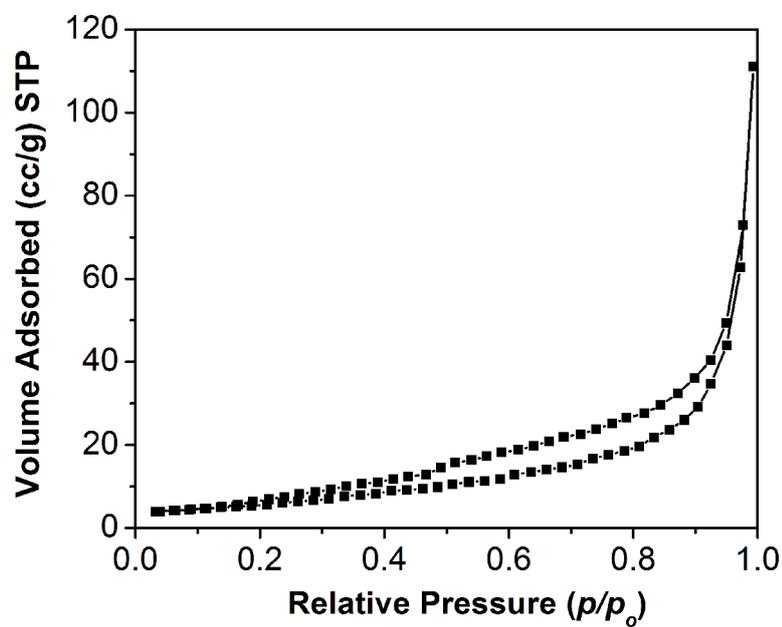
**Fig. S6** N<sub>2</sub> adsorption-desorption isotherm of annealed hierarchical MoS<sub>2</sub> microboxes.
