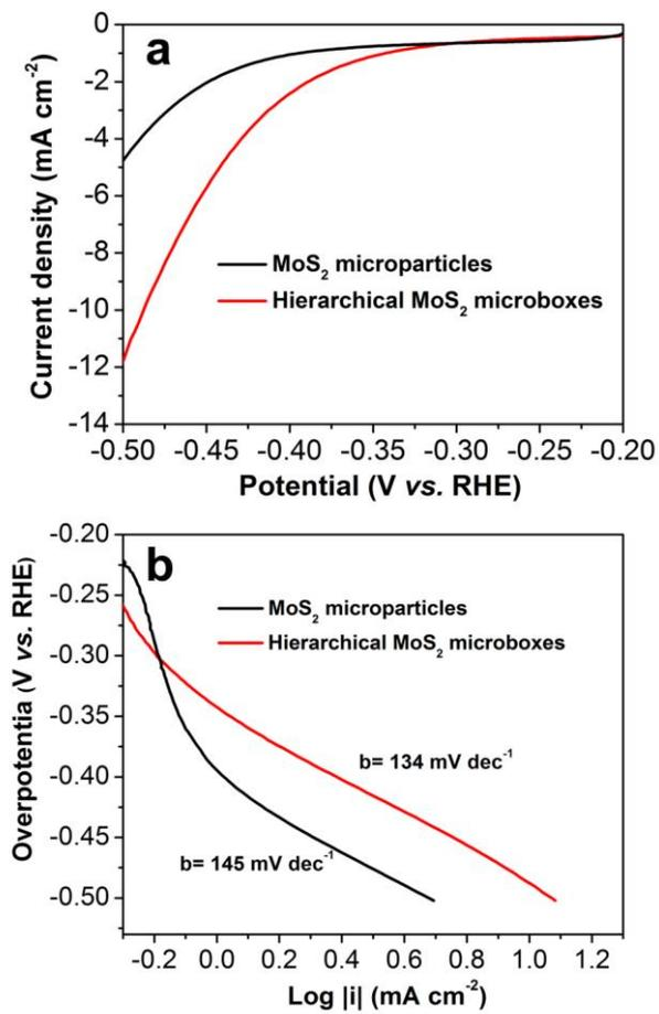
**Fig. S12** (a) Polarization curves and (b) Tafel plots for the as-prepared hierarchical MoS<sub>2</sub> microboxes and MoS<sub>2</sub> microparticles.
