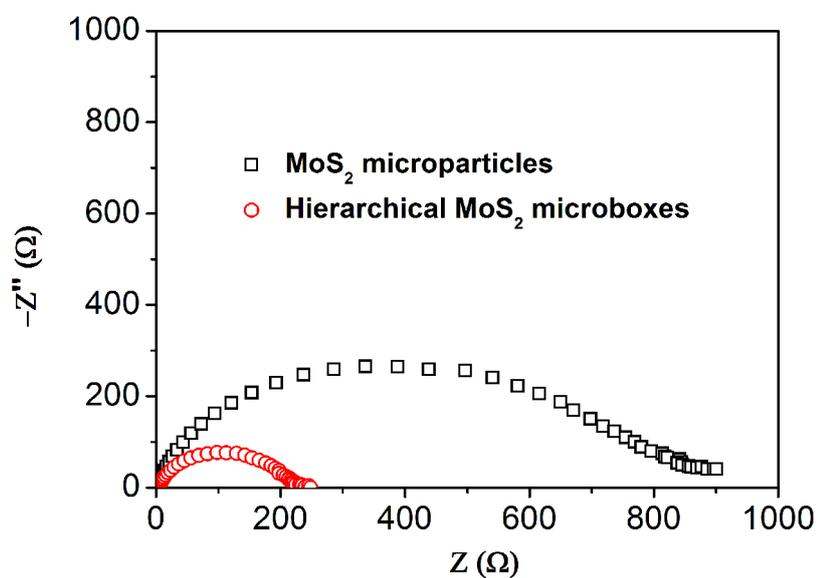
**Fig. S14** Nyquist plots of the electrodes composed of as-prepared hierarchical MoS<sub>2</sub> microboxes and MoS<sub>2</sub> microparticles.
