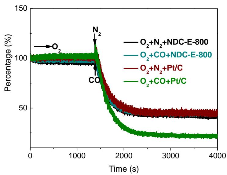
**Fig. S11** The percentage of current density ( $j$ ) vs. time chronoamperometric responses obtained at the NDC-E-800 and 20 wt% Pt/C electrodes at -0.30 V in  $O_2$ -saturated 0.1 M KOH. The arrow indicates the introduction of  $N_2$  or CO into the electrolyte.
