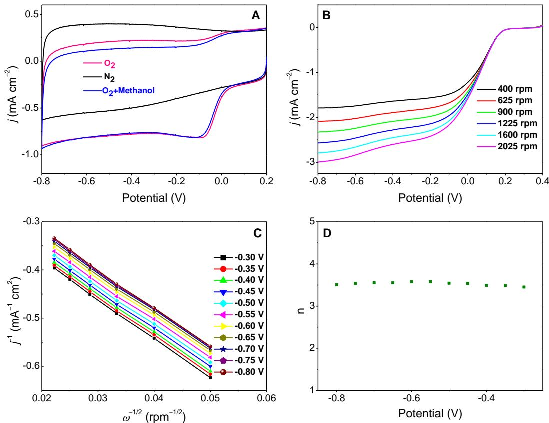
**Fig. S10** A) CV curves of NDC-E-800 in  $\text{N}_2$ -saturated,  $\text{O}_2$ -saturated 0.1 M KOH solution, and  $\text{O}_2$ -saturated 0.1 M KOH with 10 vol% methanol at a scan rate of  $10 \text{ mV s}^{-1}$ . B) RDE curves for NDC-E-800 in  $\text{O}_2$ -saturated 0.1 M KOH with a scan rate of  $10 \text{ mV s}^{-1}$  at different rotation speeds. C) K-L plots for the ORR in  $\text{O}_2$ -saturated 0.1 M KOH solution for NDC-E-800. D) The electron number calculated from K-L plot.
