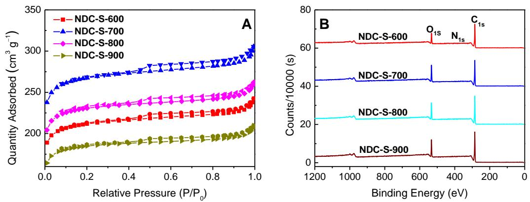
**Fig. S14** A) N<sub>2</sub> adsorption–desorption isotherms and B) Full-scan XPS of NDC-S-600, NDC-S-700, NDC-S-800, NDC-S-900.
