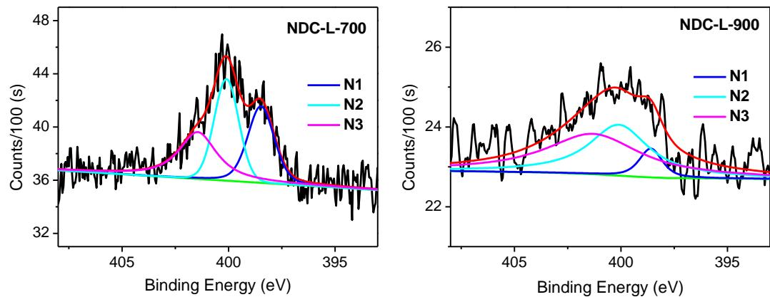
**Fig. S2** High resolution N1s XPS scan of NDC-L-700, NDC-L-900.
