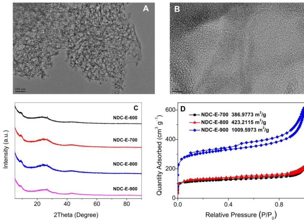
**Fig. S7** A) TEM, B) HRTEM images of NDC-E-800. C, D) XRD patterns over the  $2\theta$  range of  $5^\circ$ – $90^\circ$  and  $\text{N}_2$  adsorption–desorption isotherms of NDC-E-700, NDC-E-800, NDC-E-900.
