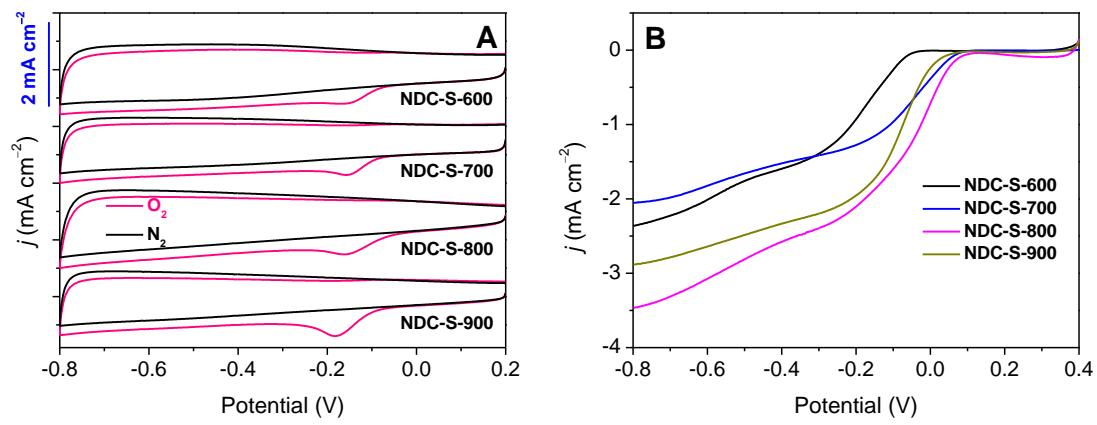
**Fig. S18** A) CV curves of NDC-S-600, NDC-S-700, NDC-S-800, NDC-S-900 in  $\text{N}_2$ -saturated,  $\text{O}_2$ -saturated 0.1 M KOH solution at a scan rate of  $10 \text{ mV s}^{-1}$ . B) RDE curves for NDC-S-600, NDC-S-700, NDC-S-800, NDC-S-900 in  $\text{O}_2$ -saturated 0.1 M KOH with a scan rate of  $10 \text{ mV s}^{-1}$  and a rotation speed of 1600 rpm.
