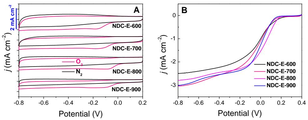
**Fig. S12** A) CV curves of NDC-E-600, NDC-E-700, NDC-E-800, NDC-E-900 in  $\text{N}_2$ -saturated,  $\text{O}_2$ -saturated 0.1 M KOH solution at a scan rate of  $10 \text{ mV s}^{-1}$ . B) RDE curves for NDC-E-600, NDC-E-700, NDC-E-800, NDC-E-900 in  $\text{O}_2$ -saturated 0.1 M KOH with a scan rate of  $10 \text{ mV s}^{-1}$  and a rotation speed of 1600 rpm.
