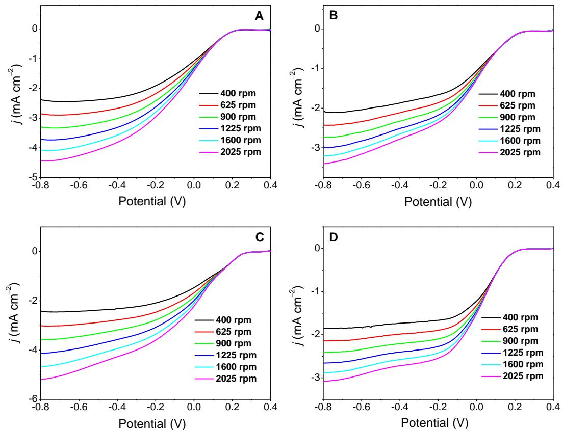
**Fig. S4** A, B, C, D) RDE curves for NDC-L-600, NDC-L-700, NDC-L-800, NDC-L-900 in  $\text{O}_2$ -saturated 0.1 M KOH with a scan rate of  $10 \text{ mV s}^{-1}$  at different rotation speeds.
