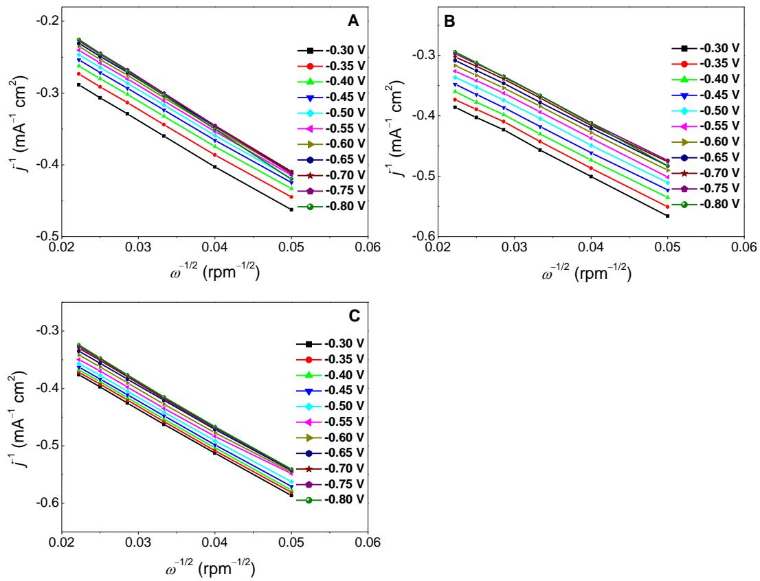
**Fig. S5** A, B, C,) K-L plots for the ORR in  $\text{O}_2$ -saturated 0.1 M KOH solution for NDC-L-600, NDC-L-700, NDC-L-900.
