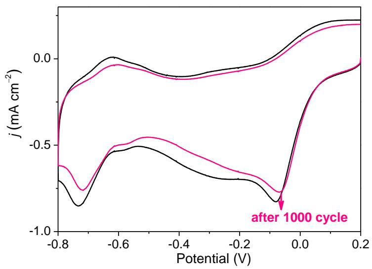
**Fig. S6** Electrochemical stability of 20 wt% Pt/C as determined by continuous CV scanning in O<sub>2</sub>-saturated 0.1 M KOH. Scan rate: 10 mV s<sup>-1</sup>.
