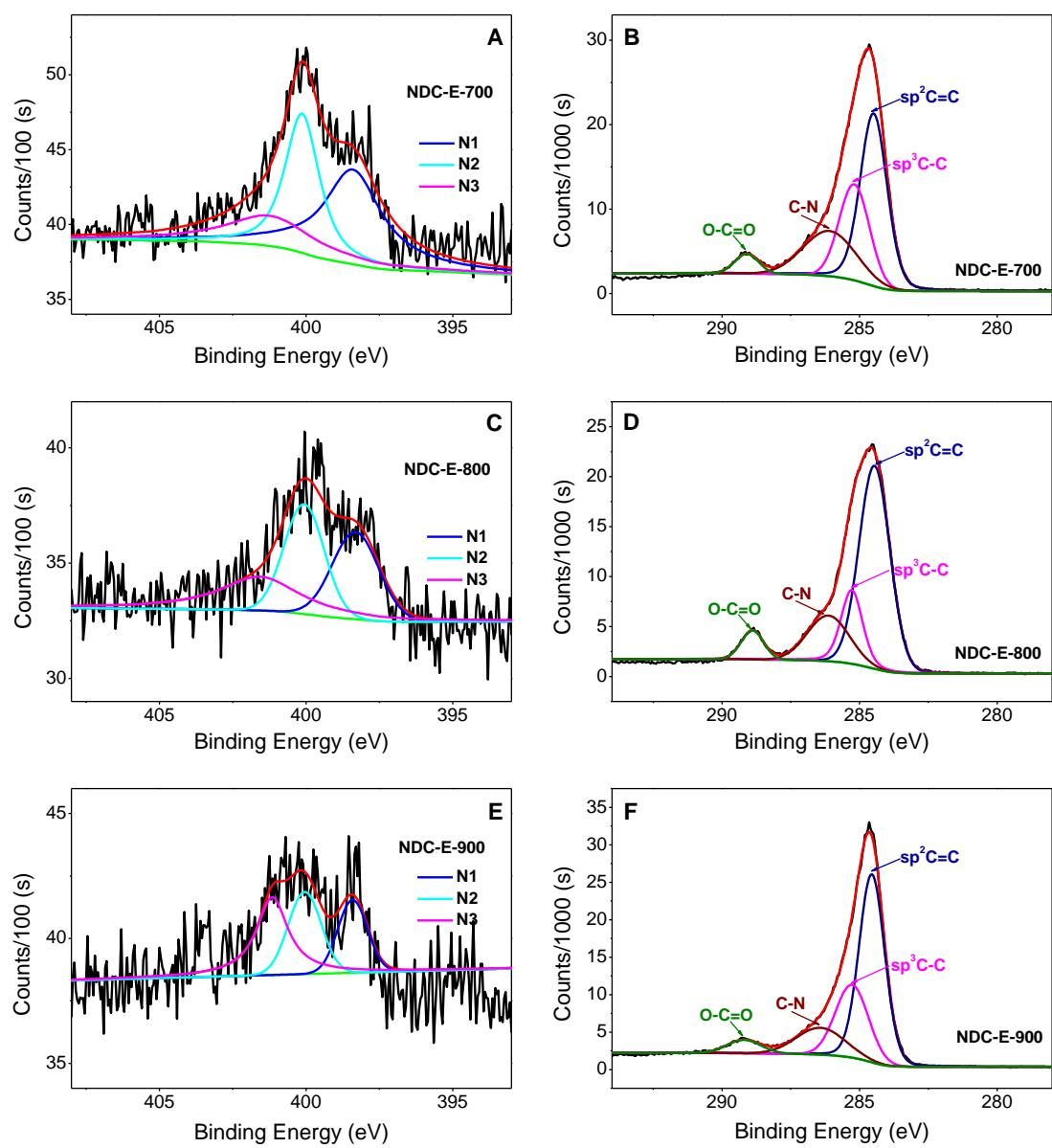
**Fig. S9** High resolution N1s and C1s XPS scan of NDC-E-700, NDC-E-800, NDC-E-900.
