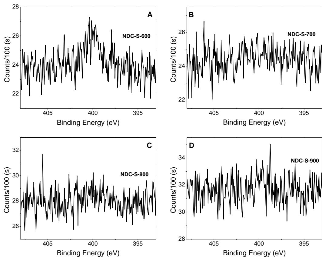
**Fig. S16** High resolution N1s XPS scan of NDC-S-600, NDC-S-700, NDC-S-800, NDC-S-900.
