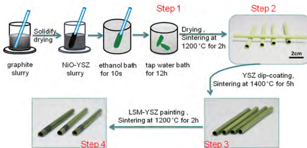
Fig. S2 Schematic diagram for the fabrication process of the tubular unit.
