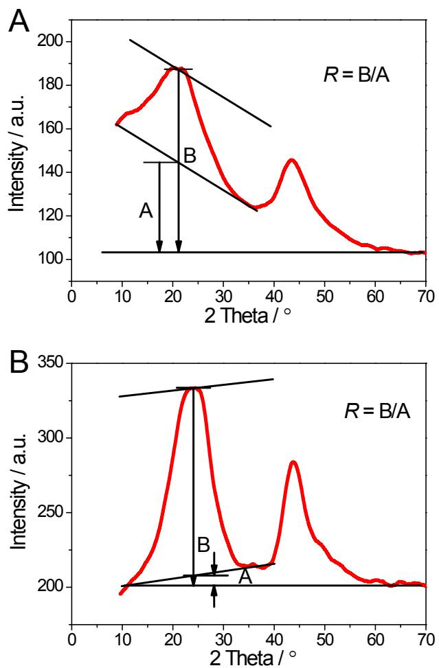
**Figure S5:** Scheme illustrating the  $R$  values calculation based on XRD patterns for PSNCs (A) and PSOCs (B).
