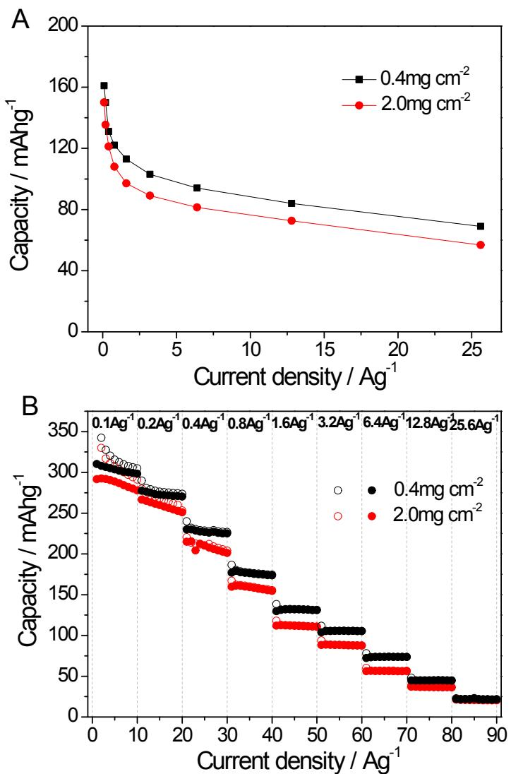
**Figure S13:** The electrochemical performance of PSNC-3-800 (A) and PSOC-A (B) with two different electrode mass loadings.
