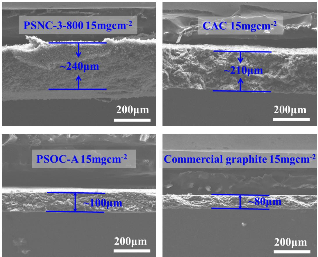
**Figure S14:** Cross section SEM images of (A) PSNC-3-800 (B) CAC, (C) PSOC-A and (D) commercial graphite thin film electrodes with commercial mass loadings.
