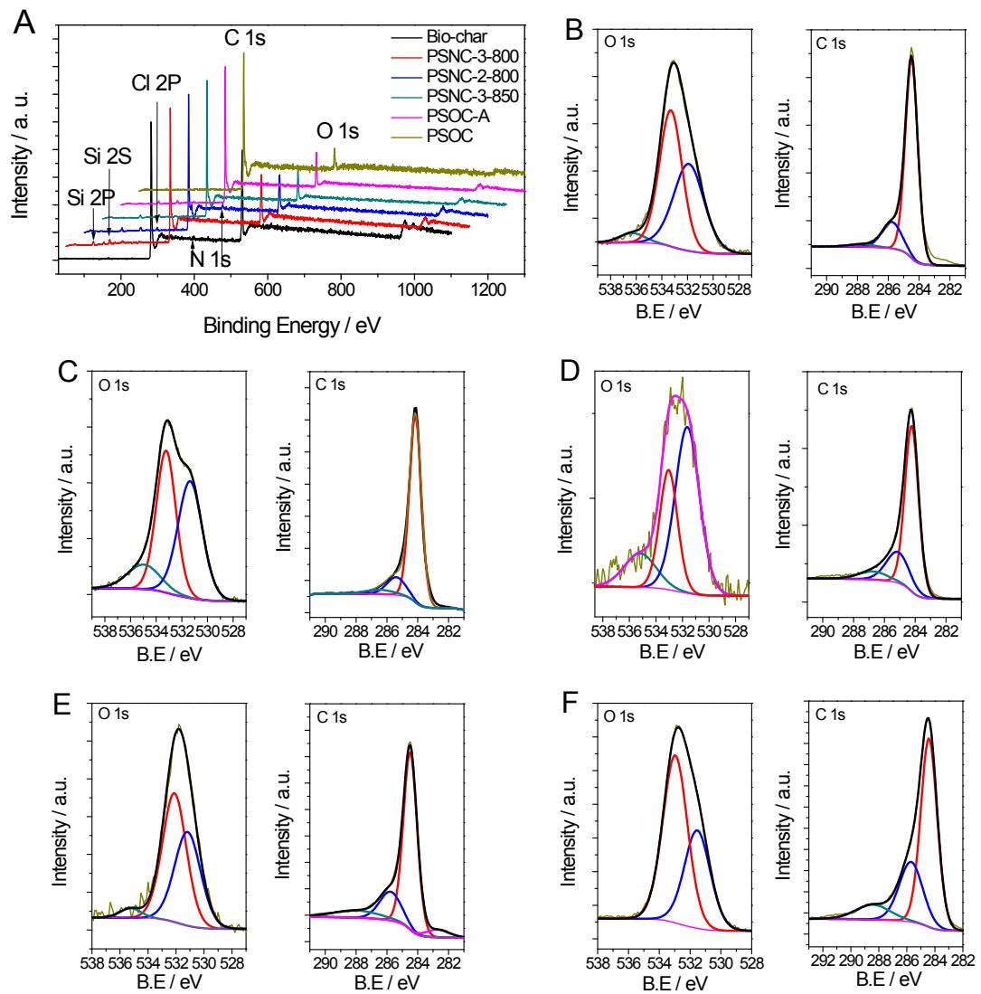
**Figure S8:** (A) XPS survey spectra of PSNC, PSOC and hydrothermal biochar. Magnified views of the C 1s, N 1s and O 1s core level XPS spectra with fits for (B) PSNC-3-850, (C) PSNC-2-800, (D) PSOC, (E) PSOC-A, (F) hydrothermal obtained biochar.
