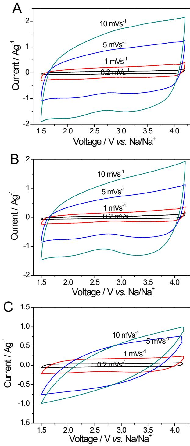
**Figure S9:** (A-C) Cyclic voltammograms (CVs) of PSNC-3-850, PSNC-2-800, and CAC, respectively.
