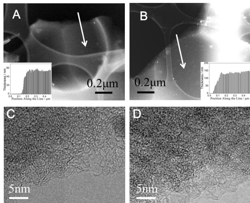
**Figure S3:** HAADF TEM micrographs and thickness profiles (insert) of (A) PSNC-3-850 and (B) PSNC-2-800, measured from low-loss EELS along the white arrows. HRTEM micrographs of (C) PSNC-3-850, and (D) PSNC-2-800.
