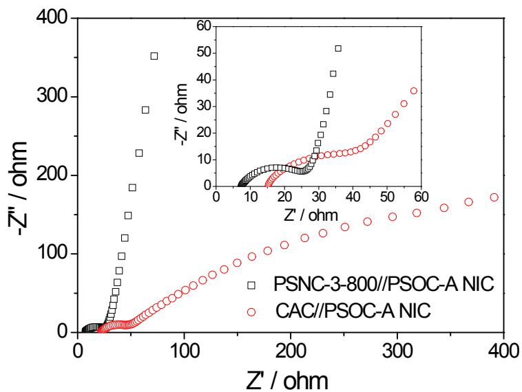
**Figure S19:** Nyquist plots of PSNC-3-800//PSOC-A and CAC//PSOC-A after rate tests.
