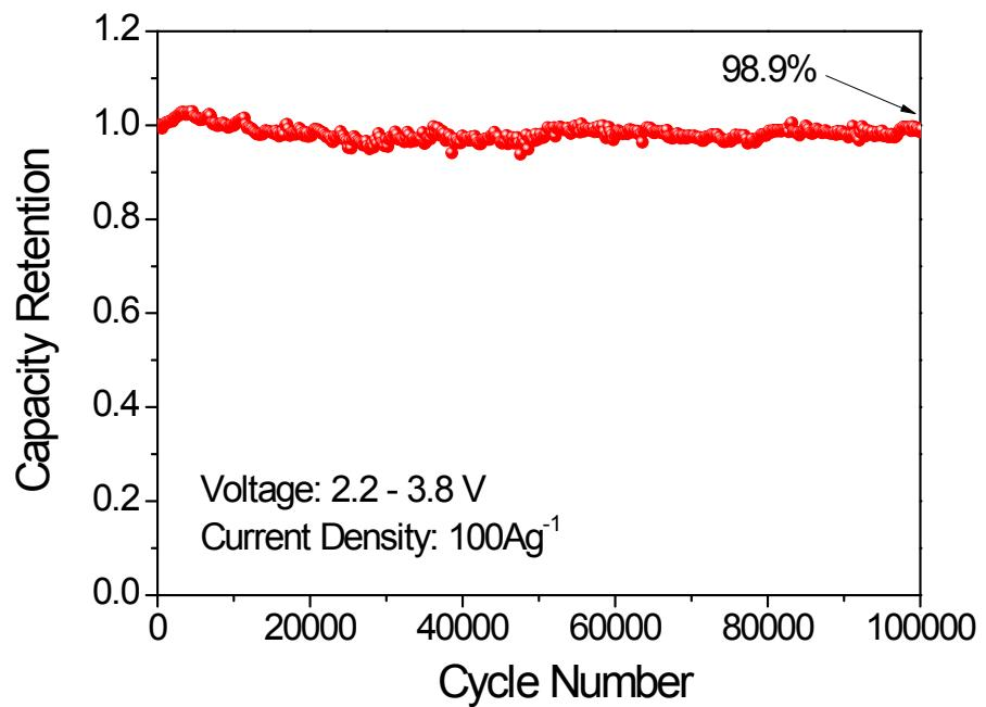
**Figure S18:** Cycling stability of PSNC-3-800//PSOC-A hybrid ion capacitor at a current density of  $100\text{Ag}^{-1}$  and voltage window of 2.2-3.8V.
