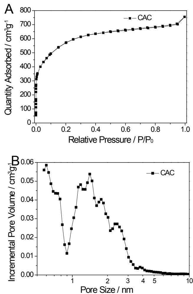
**Figure S7:** (A)-(B) Nitrogen adsorption-desorption isotherms and pore size distributions of CAC.
