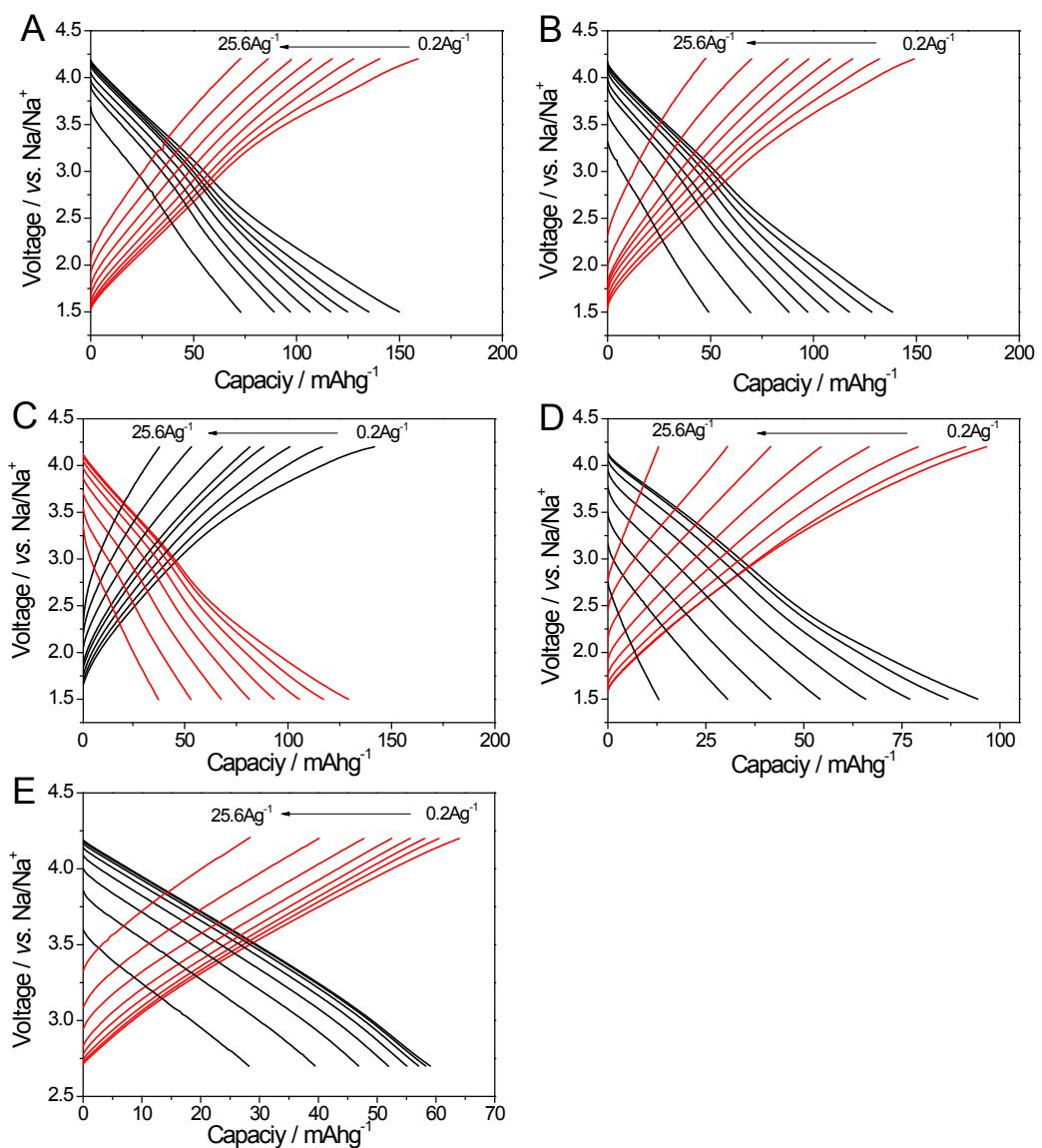
**Figure S10:** Galvanostatic discharge/charge profiles of (A) PSNC-3-800, (B) PSNC-3-850, (C) PSNC-2-800 and (D) CAC, (E) PSNC-3-800 within voltage region of 2.7-4.2 V vs. Na/Na<sup>+</sup>.
