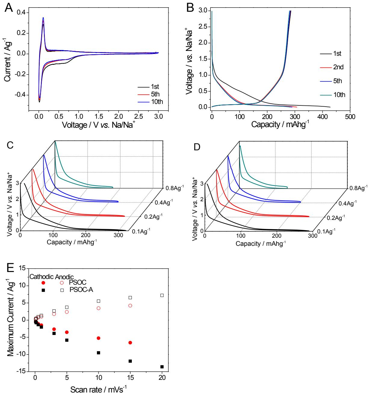
**Figure S16:** (A) CVs of PSOC specimen at a scan rate of  $0.1\text{mVs}^{-1}$ . (B) Galvanostatic discharge/charge profiles of PSOC at density of  $0.1\text{Ag}^{-1}$ . (C-D) Galvanostatic discharge/charge profiles of PSOC-A (C) and PSOC (D) at current densities of 0.1, 0.2, 0.4 and  $0.8\text{Ag}^{-1}$ . (E) Dependence of anodic and cathodic peak currents on scan rate for PSOC and PSOC-A.
