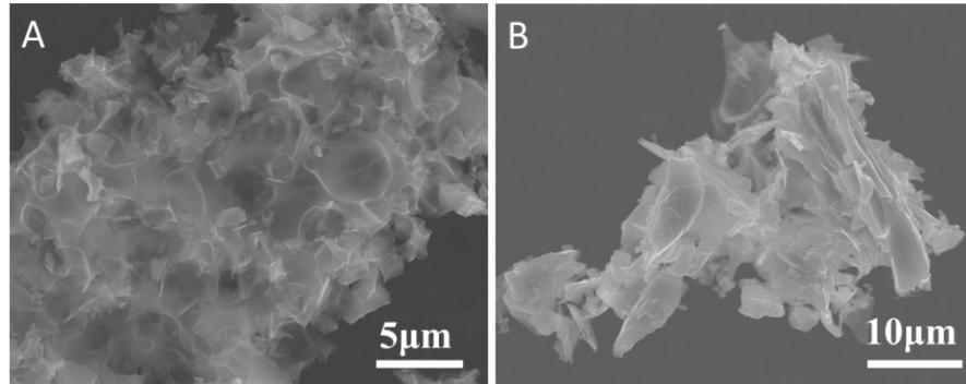
**Figure S2:** SEM micrographs of cathode and anode carbons achieved when employing the entire peanut shell as a single precursor for either synthesis process. (A) cathode carbon. (B) anode carbon.
