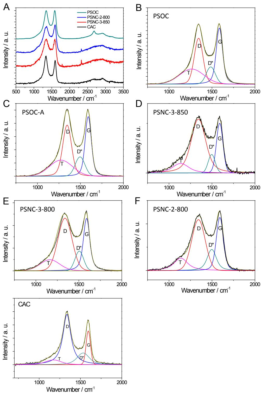
**Figure S6:** (A) Raman spectra of PSNC-2-800, PSNC-3-850 and PSOC specimens.
