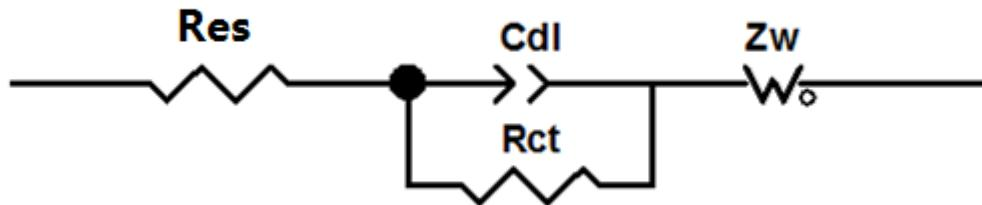
**Figure S20:** Equivalent electronic circuits used to simulate the EIS data.  $R_{es}$  is the sum of resistances of electrical connections in the experiment setup including ionic diffusion resistance in the electrolyte.  $R_{ct}$  reflects the charge transfer resistance and  $Z_w$  (Warburg-type element) represents Na diffusion impedance within carbon materials.
