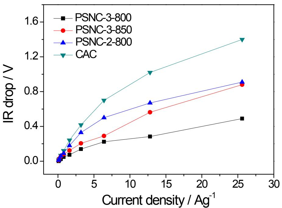
**Figure S11:** IR drops of PSNC specimens and CAC in half cells.
