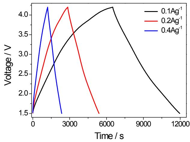
**Figure S17:** (A) Galvanostatic discharge/charge profiles of PSNC-3-800//PSOC-A hybrid Na-ion capacitor at low current densities.
