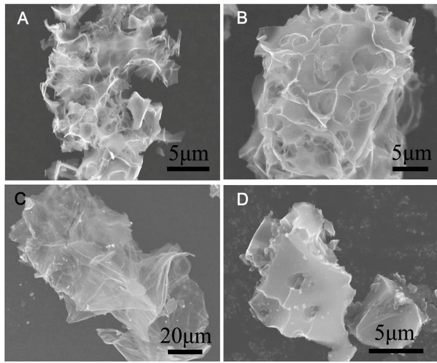
**Figure S1:** SEM micrographs of (A) PSNC-3-850 and (B) PSNC-2-800, (C) PSOC, (D) the baseline commercial activated carbon (CAC).
