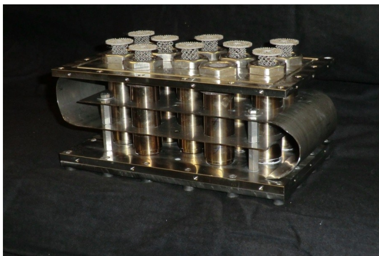
Fig. S1 Hydrogen release unit (HRU) consisting of ten parallel reactors mounted in vertical direction – photograph of the open HRU unit with ten SEBM-manufactured and catalytically functionalized reactor tubes. The unit is surrounded by a box to guide the hot air flow.
