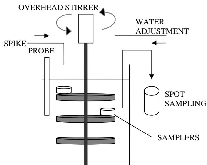
**Figure S1.** Diagram of the tank test.
