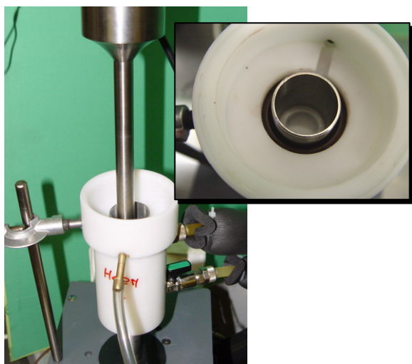
Figure 1. Immersion horn inserted in the cup-horn (cavitating tube); the inset shows the latter as seen from the top.
