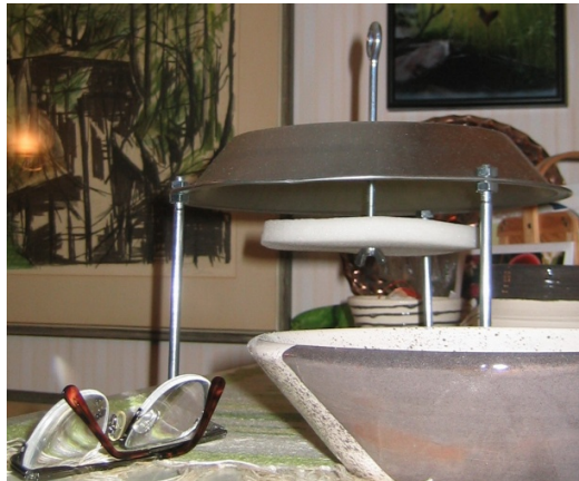
Figure S1 Examples of PUF-based passive air samplers deployed in outdoor and indoor environments.
