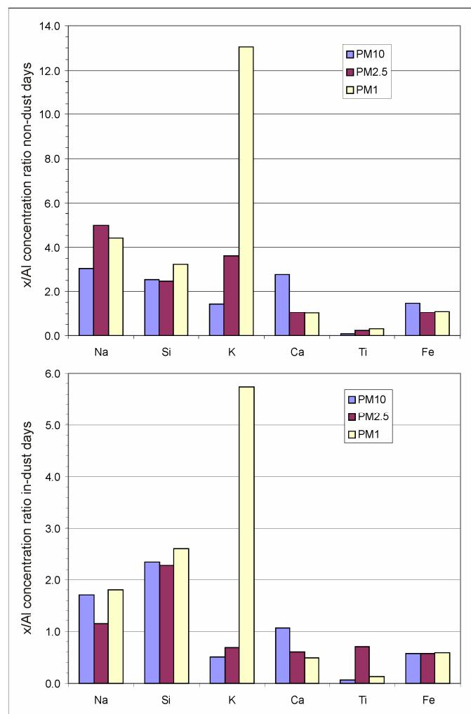
**Fig. S13** Concentration values mean ratio (crustal element to Al ratio) for the different PM fractions, non-dust days (above) and in-dust days (below).
