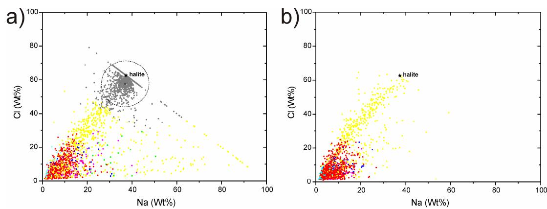
**Fig. S8** Na-Cl binary graphics for the  $\text{PM}_{10}$  at CR station, non-dust days (a) and in-dust days (b). Graphics showed compositions of halite and confidence ellipses of 95% (prediction and mean) for [Cl, Na] cluster. See color legend in Fig. 2 or Fig. S6.
