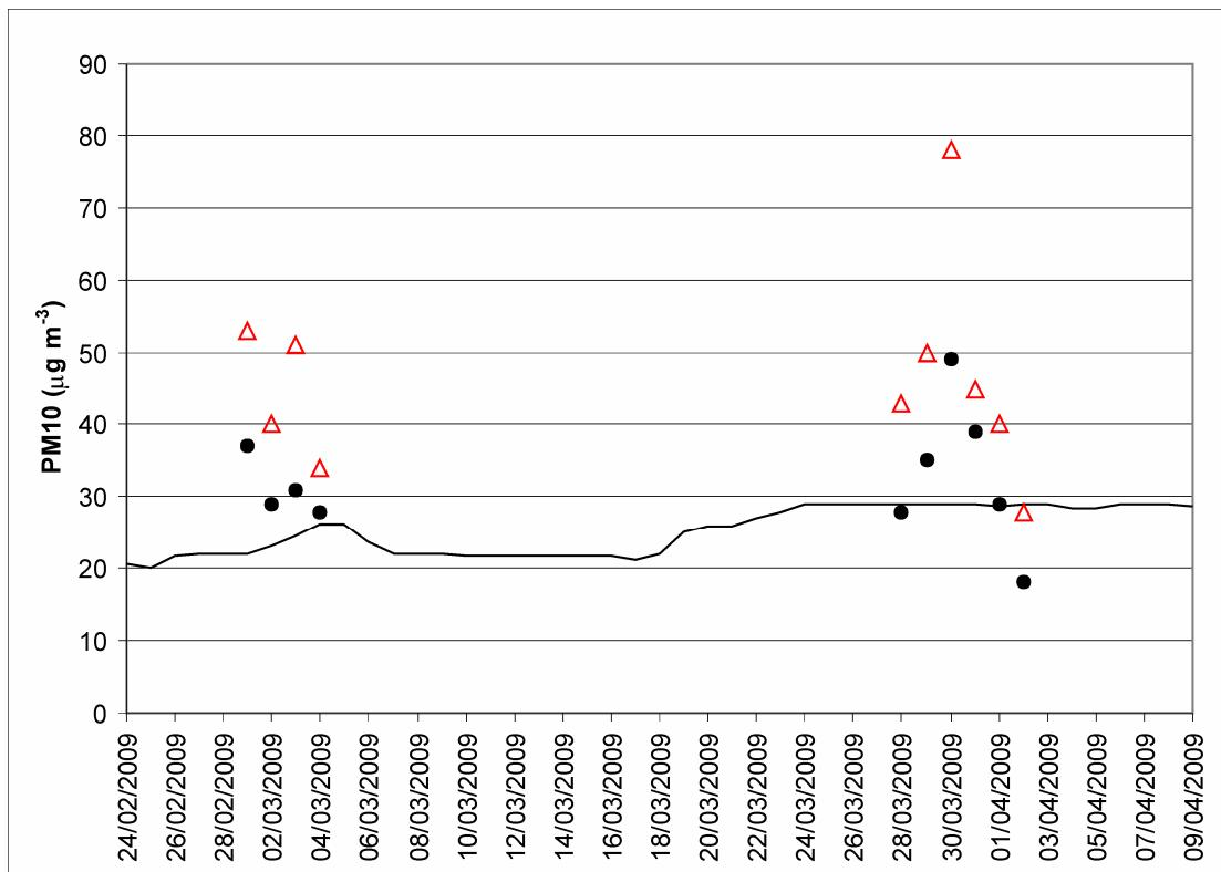
**Fig. S4** Daily mean of the PM<sub>10</sub> concentration values during in-dust days at suburban CR station (dots) and at urban CF station (triangles) compared to the monthly moving 30th percentile of non-dust days calculated at CR (solid line). The Saharan contribute was evaluated at CR station as gap from dot to solid line at the same day; then this contribution was compared to the triangle value to evaluate his influence to the urban area.
