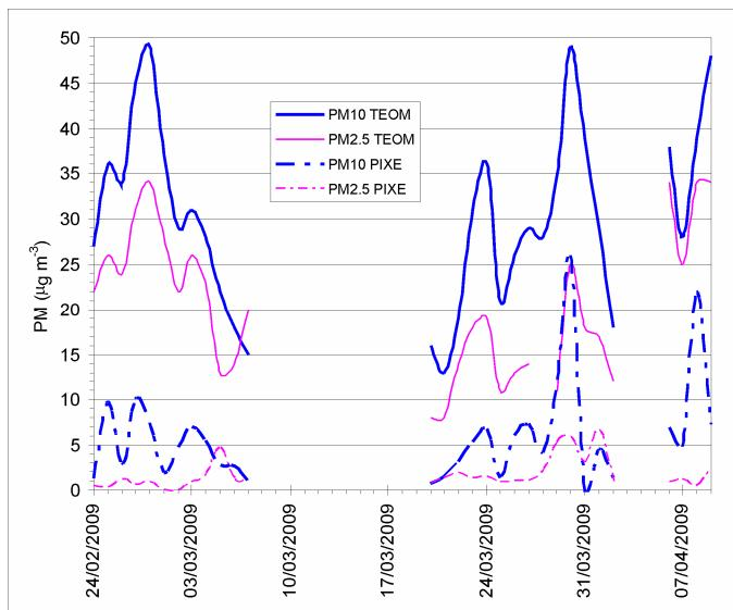
**Fig. S11** PM Concentration values measured at CR station by TEOM (solid lines) and calculated as sum of elements by PIXE analysis (dashed lines).
