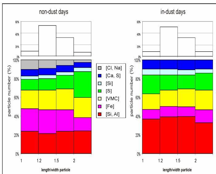
**Fig. S10** Particles distribution in different aspect classes based on their aspect ratio (length to width ratio), total (above) and by cluster membership (below), non-dust days (left) and in-dust days (right).
