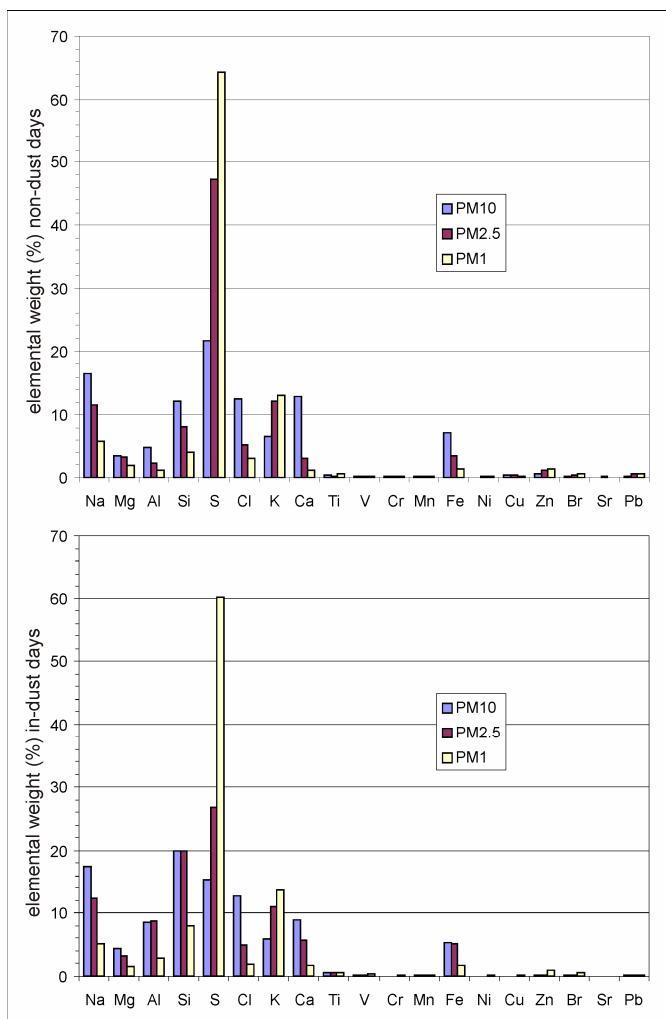
**Fig. S12** Weight percent average of elements by PIXE analysis in the different PM fractions, non-dust days (above) and in-dust days (below).
