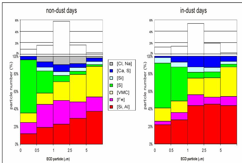
**Fig. S9** Particles distribution in different size classes based on their Equivalent Circular Diameter (ECD), total (above) and by cluster membership (below), non-dust days (left) and in-dust days (right).
