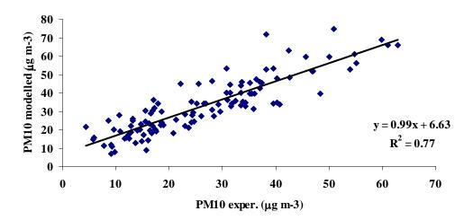
**Figure S1.** Plot between the experimental and the modelled PM10 obtained by the PCA-APCS receptor model ( $R^2$ = correlation coefficient).
