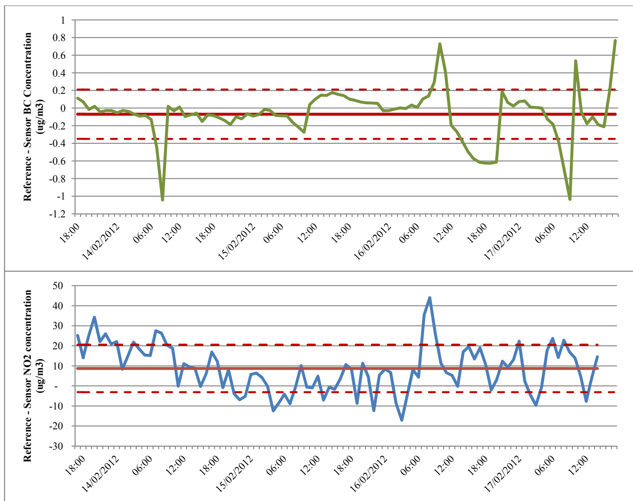
Figure S2 Black carbon (top) and NO 2 (bottom) drift of sensors ( \mu\text{g}/\text{m}^3 ) measured at Birmingham Tyburn as the difference between the reference method and the sensor during the validation campaign of the sensors at field conditions.
