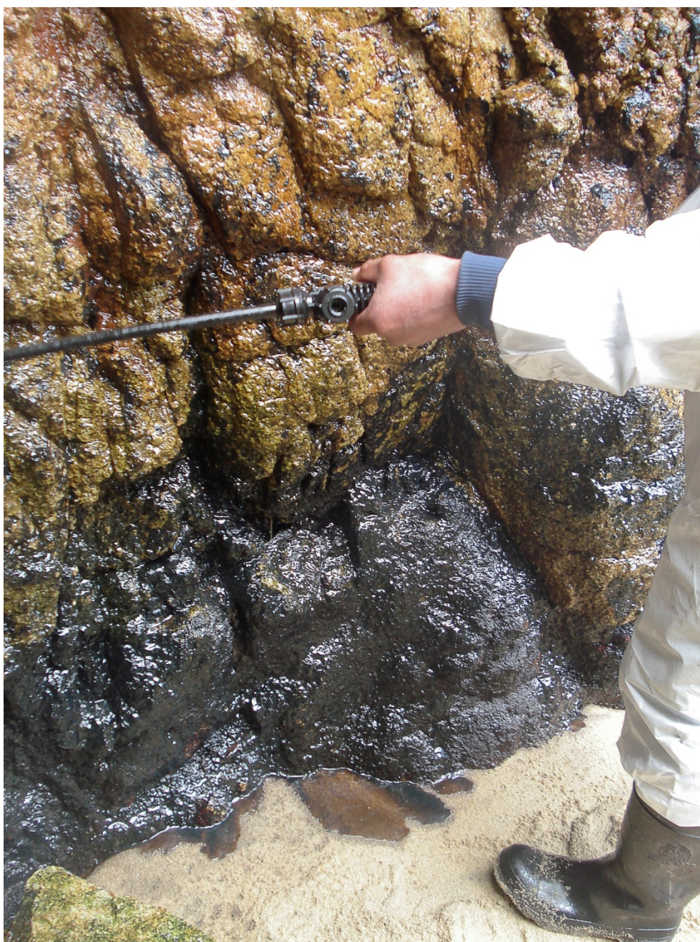
Figure S1. Cleaning oil off a rock face. The upper portion of the rock face has been cleaned with the biosolvent and the dissolved weathered oil can be seen flowing down the face into the sand.
