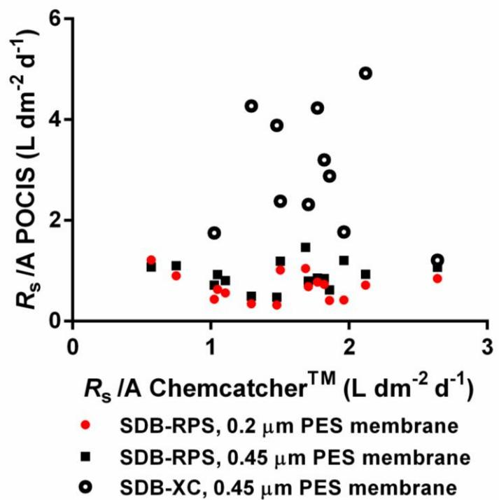
**Fig. S4. Sampling rates normalized on surface area ( $R_s/A$ ;  $\text{L dm}^{-2} \text{ d}^{-1}$ ) for target chemicals with POCIS vs. Chemcatchers<sup>TM</sup>, showing no correlation.**
