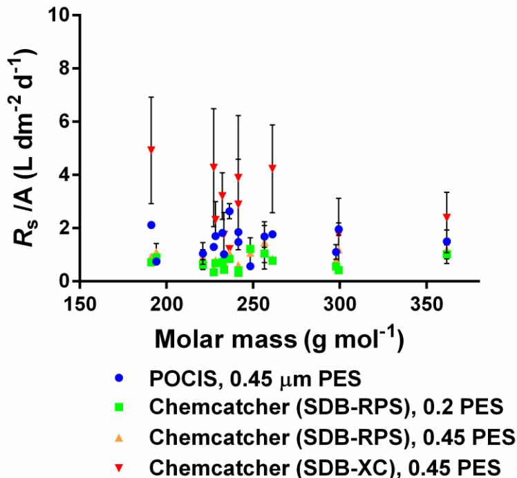
Fig. S6. Sampling rates normalized on surface area ( $R_s/A$ ;  $\text{L dm}^{-2} \text{d}^{-1}$ ) vs. molar mass for target chemicals with POCIS and Chemcatcher<sup>TM</sup>.
