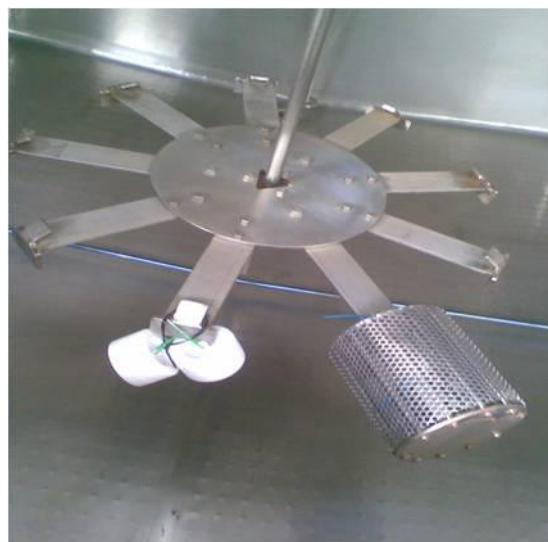
**Fig S2. Photograph showing the position of Chemcatcher™ samplers (left) and a POCIS deployment cage (right) in the calibration water tank.**
