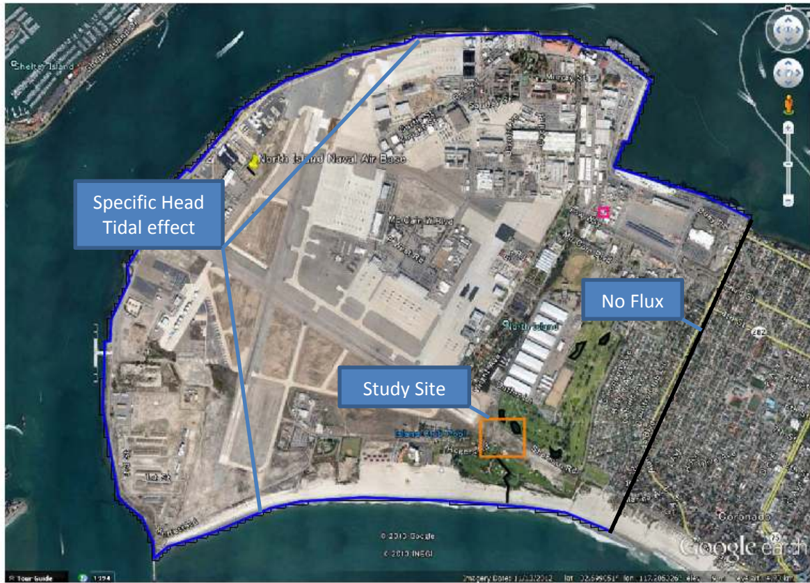
Figure 2-3. Domain of the areal model to simulate the hydrology of the study site (in the orange square) and the surrounding area. Elevation of the observed sea level was imposed along the solid blue line to simulate the tidal effect. No flux boundary condition was set for the eastern boundary (black line).
