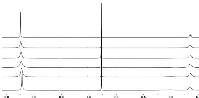
Figure S3. Addition of MeOH to a solution of **2** in  $CDCl_3$ . From the bottom: 0%, 0.25%, 0.5%, 0.75%, 1% and 2% MeOH
