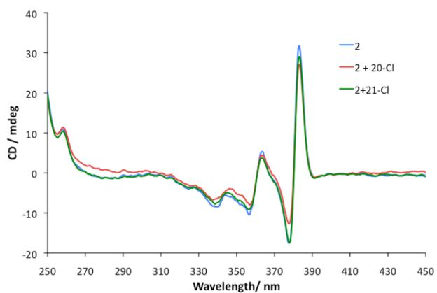
Figure S12. CD spectra of **2** upon addition of acetylcholine chloride (**20-Cl**) and **21-Cl**.
