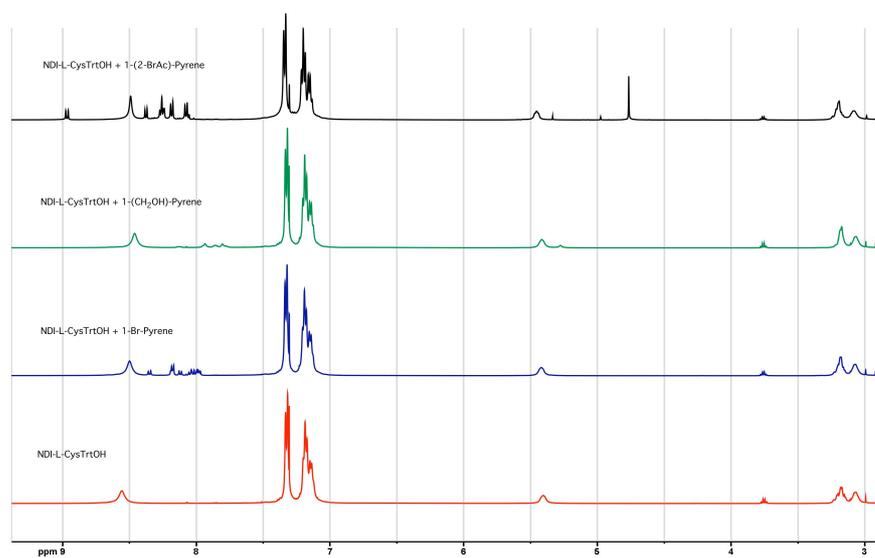
Figure S13.  $^1\text{H-NMR}$  spectra (bottom to top) of 1:2 mixtures of **1** + **6**, **7**, and **9**, in  $\text{CDCl}_3$ .
