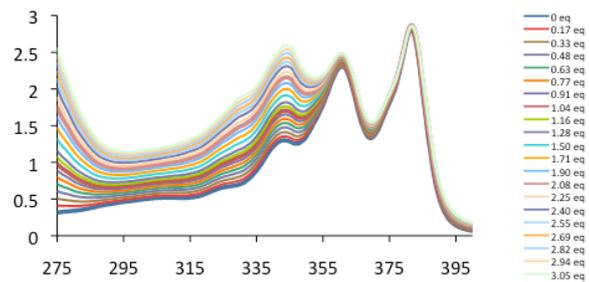
Figure S4. UV-Vis spectra of **2** titrated with a solution of **13** in  $\text{CHCl}_3$
