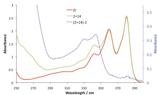
Figure S11. UV-Vis spectra of **2** and a mixture **2+14** (1:1 ratio) and the contribution of **14** to the **2+14** solution (dotted line).
