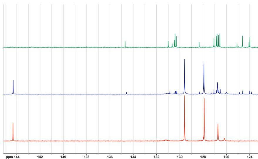
Figure S16.  $^{13}\text{C}$ -NMR spectra (bottom to top) of **1**, **1 + 9** (1:2 mixture), **9** in  $\text{CDCl}_3$  (zoom)
