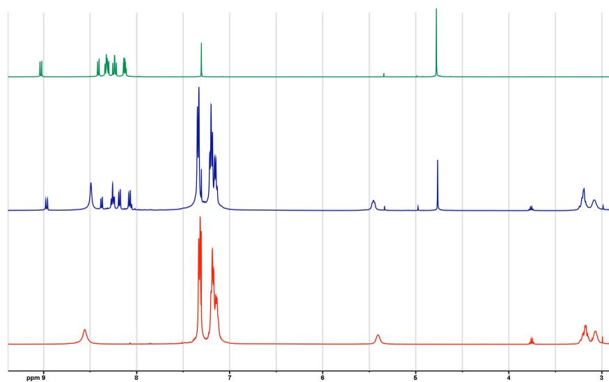
Figure S14.  $^1\text{H-NMR}$  spectra (bottom to top) of **1**, **1** + **9** (1:2 mixture), **9** in  $\text{CDCl}_3$
