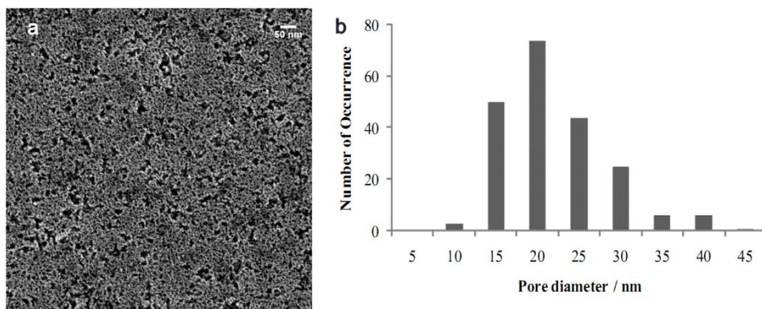
Figure S4. a) Top view scanning electron micrograph of the PSi rugate filter. b) Histogram of the pore size distribution.
