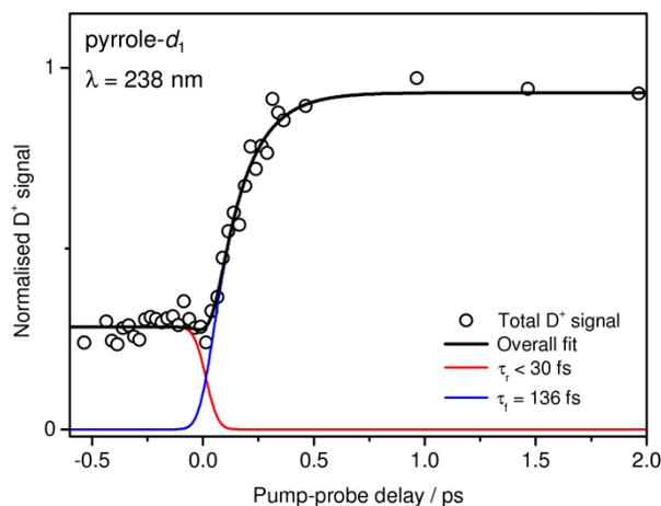
**Fig. S2** Normalised D<sup>+</sup> signal transient from pyrrole-*d*<sub>1</sub> obtained using TR-IY (open circles), with a 238 nm pump and 243.1 nm probe combination, together with the resultant kinetic fit (black line). A one-colour 243.1 nm background signal has been subtracted from the displayed transient. Individual fit components associated with  $\tau_f = 136$  fs (blue) and  $\tau_r < 30$  fs (red) are also shown.
