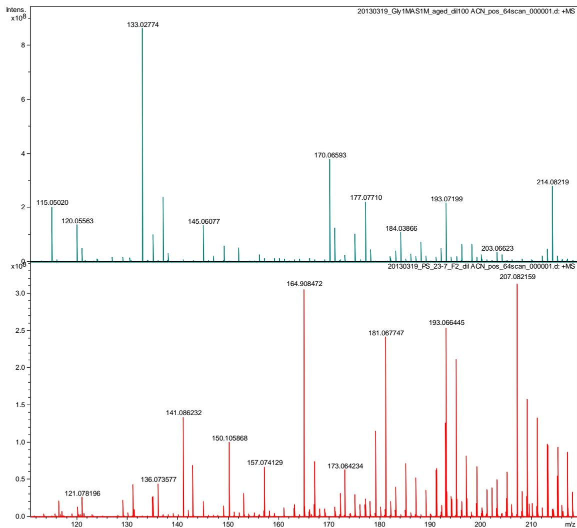
Supp Fig 2: FTICR-MS positive ionization mass spectra. Upper: 1 M GLY + 1M AS lab solution (aged 6 months). Lower: Filter F2 aqueous extract from 23/07/12 GLY+AS+HONO+light experiment.
