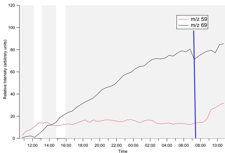
Supp Fig 4: Temporal evolution of ATOFMS  $m/z$  59 and  $m/z$  69 ions during the experiment on 23-24/07/2012. Shaded grey areas = chamber closed. White shaded areas = chamber open. Vertical blue line = flushing begins.
