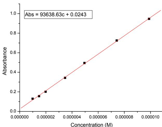
**Figure 1** Calibration plot relating concentration (c) of dye solution with UV absorbance (Abs)
