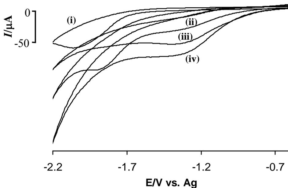
**Figure 1A** Cyclic voltammograms (scan rate of  $100 \text{ mVs}^{-1}$ ) obtained at a 3 mm diameter Pt disc electrode immersed in 0.1 M  $n\text{-Bu}_4\text{NBF}_4\text{-DMF}$  for (i) 3 mM benzyl bromide, (ii) 3 mM benzyl bromide in the presence of 15 mM acetic anhydride, (iii) 3 mM benzyl bromide in the presence of 30 mM acetic anhydride, and (iv) 3 mM benzyl bromide in the presence of 60 mM acetic anhydride.
