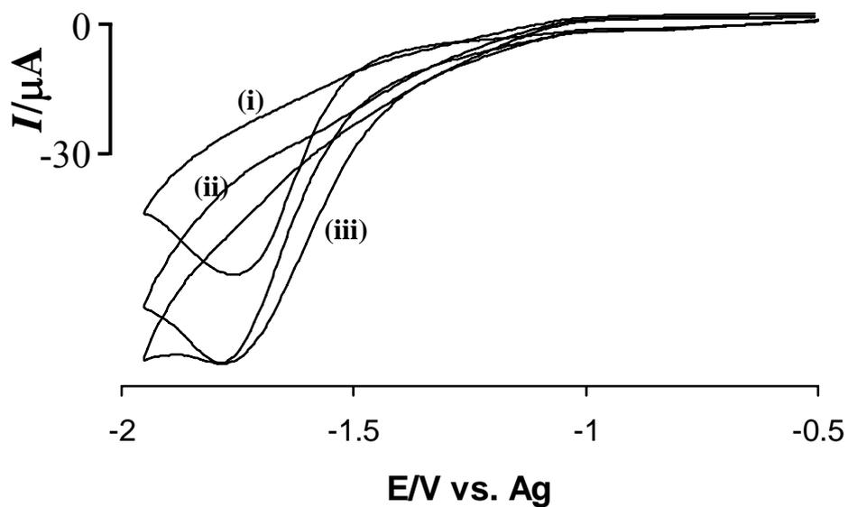
**Figure 1B** was cyclic voltammograms (scan rate of  $100 \text{ mVs}^{-1}$ ) obtained at a 3 mm diameter Au disc electrode immersed in  $0.1 \text{ M } n\text{-Bu}_4\text{NBF}_4\text{-DMF}$  for (i) 3 mM benzyl bromide, (ii) 3 mM benzyl bromide in the presence of 30 mM acetic anhydride, and (iii) 3 mM benzyl bromide in the presence of 60 mM acetic anhydride.
