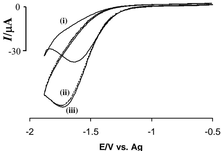
**Figure 1C** was cyclic voltammograms (scan rate of  $100 \text{ mVs}^{-1}$ ) obtained at a 3 mm diameter GC (glass carbon) disc electrode immersed in  $0.1 \text{ M } n\text{-Bu}_4\text{NBF}_4\text{-DMF}$  for (i) 3 mM benzyl bromide, (ii) 3 mM benzyl bromide in the presence of 30 mM acetic anhydride, and (iii) 3 mM benzyl bromide in the presence of 60 mM acetic anhydride.
