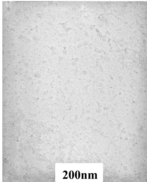
SI-1: TEM images of silica fragments obtained for [\text{SiO}_2] = 0.02 \text{ M} and [\text{alginate}] = 0.05 \text{ wt\%} and re-dispersion in water at 95 \text{ }^\circ\text{C}
