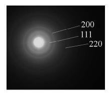
Figure S1 SAED pattern of gold nanoparticles prepared in the presence of IL-NH<sub>2</sub>.
