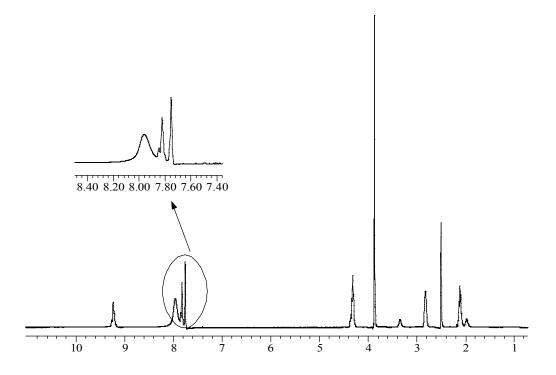
Figure S4 <sup>1</sup>H NMR spectrum of IL-NH<sub>2</sub>. Inset indicated the presence of -NH<sub>2</sub>.
