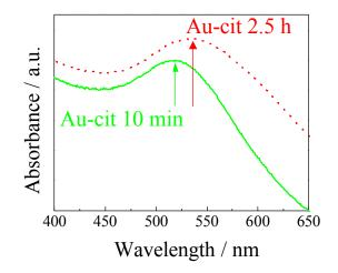
Figure S7 UV-vis spectra of Au-cit nanoparticles kept at room temperature over time.
