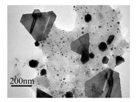
Figure S6 TEM image of Au-IL after the dialysis.
