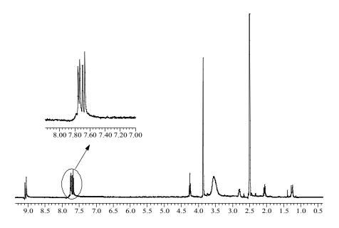
Figure S5 <sup>1</sup>H NMR spectrum of Au-IL. Inset indicated the  $-NH_2$  disappeared after the reaction.
