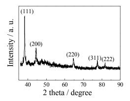
Figure S2 XRD pattern of gold nanoparticles prepared in the presence of IL-NH<sub>2</sub>.
