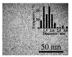
Figure S8 TEM image of Au-SH nanoparticles.
