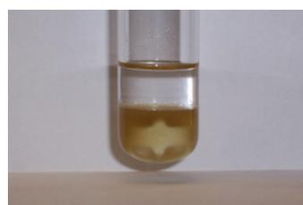
The ionic liquid is washed with water
