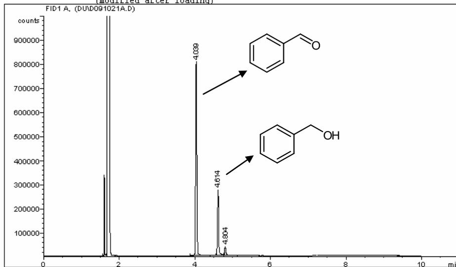
Fig. 17 GC chromatogram of the reaction mixture (Table 1, Entry 2 in the main text)
