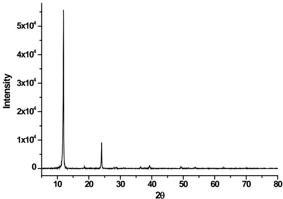
Fig. 4 XRD pattern of VOPO<sub>4</sub>·2H<sub>2</sub>O.
