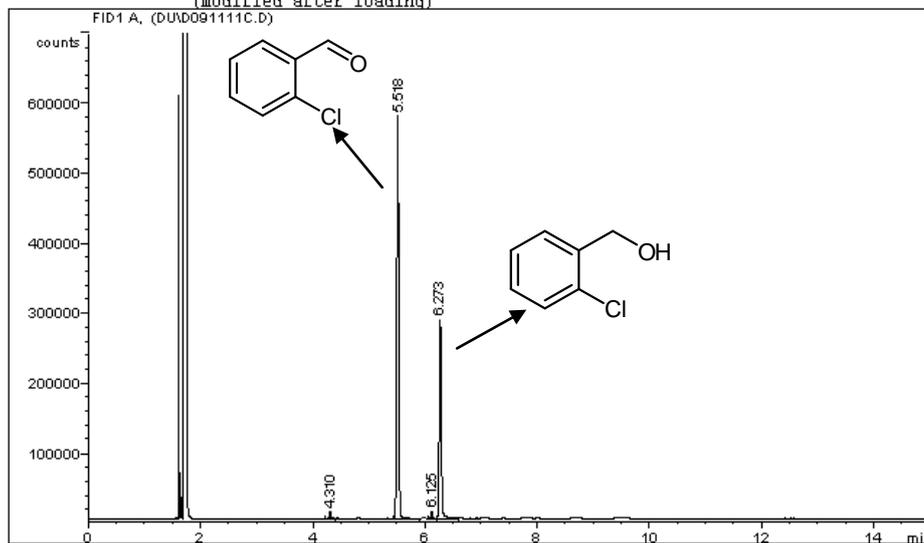
Fig. 23 GC chromatogram of the reaction mixture (Table 1, Entry 8 in main text)
