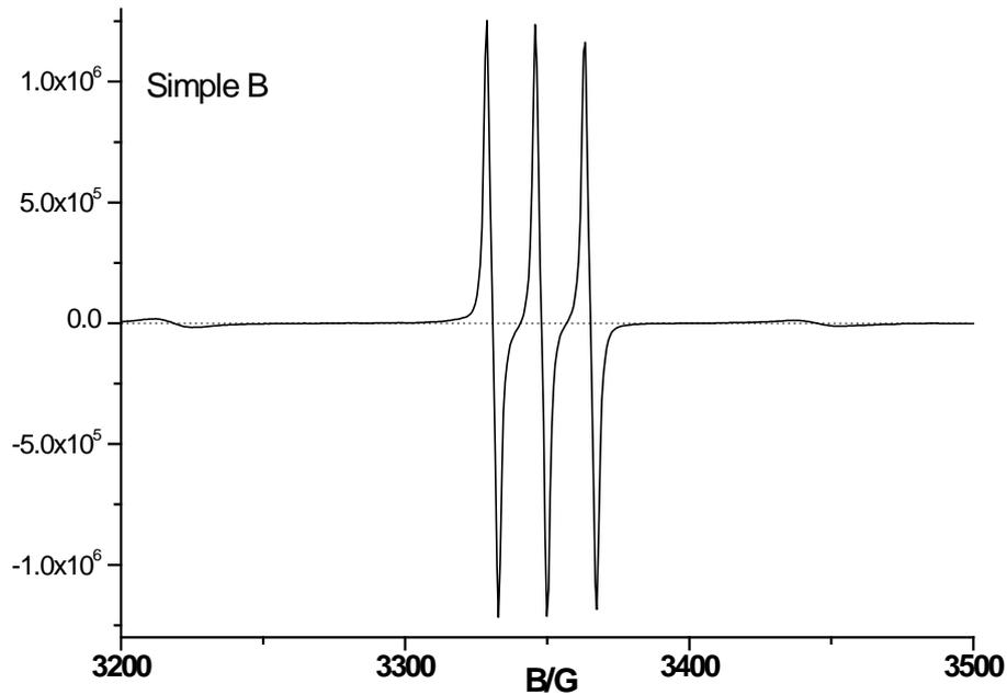
Fig. 13 EPR spectrum of TEMPO remaining in Sample B.
