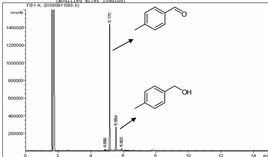
Fig. 18 GC chromatogram of the reaction mixture (Table 1, Entry 3 in main text)
