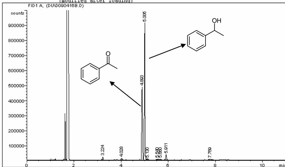
Fig. 24 GC chromatogram of the reaction mixture (Table 1, Entry 9 in main text)
