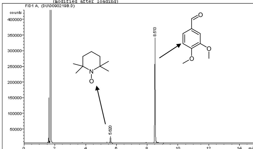
Fig. 16 GC chromatogram of the reaction mixture (Table 1, Entry 1 in the main text)
