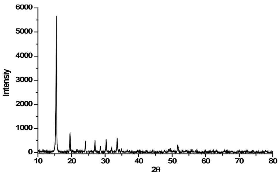
Fig. 6 XRD pattern of VOHPO<sub>4</sub>·0.5H<sub>2</sub>O.
