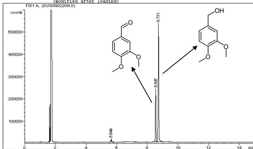
Fig. 15 GC chromatogram of the reaction mixture (Fig. 1, experiment 5 in the main text)
