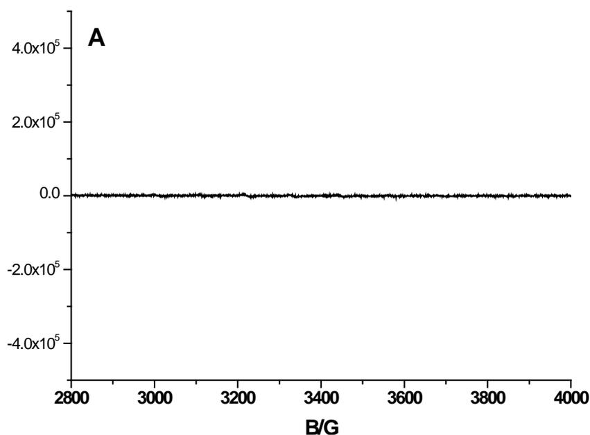
Fig. 10 EPR of VOPO<sub>4</sub> aqueous solution (Sample A).
