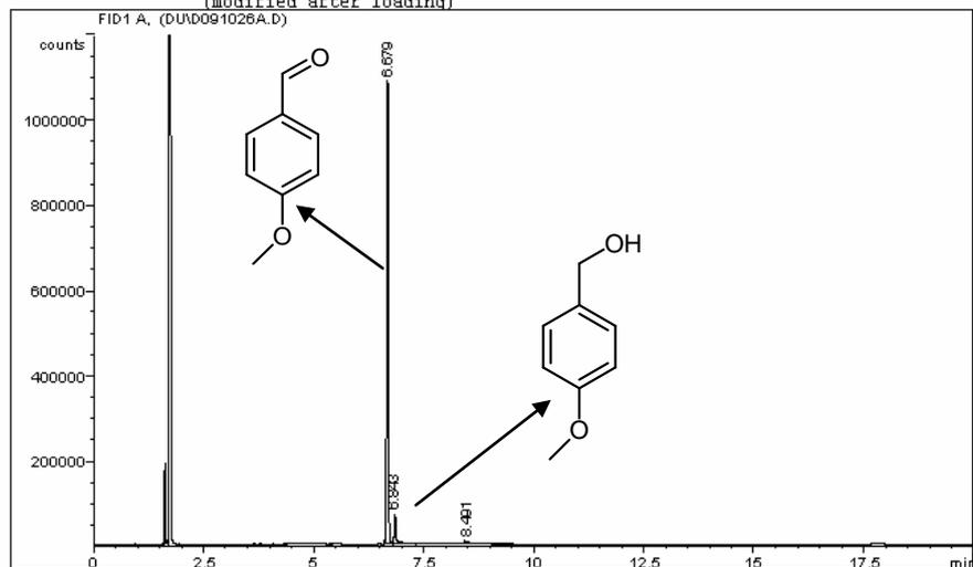
**Fig. 21** GC chromatogram of the reaction mixture (Table 1, Entry 6 in main text)
