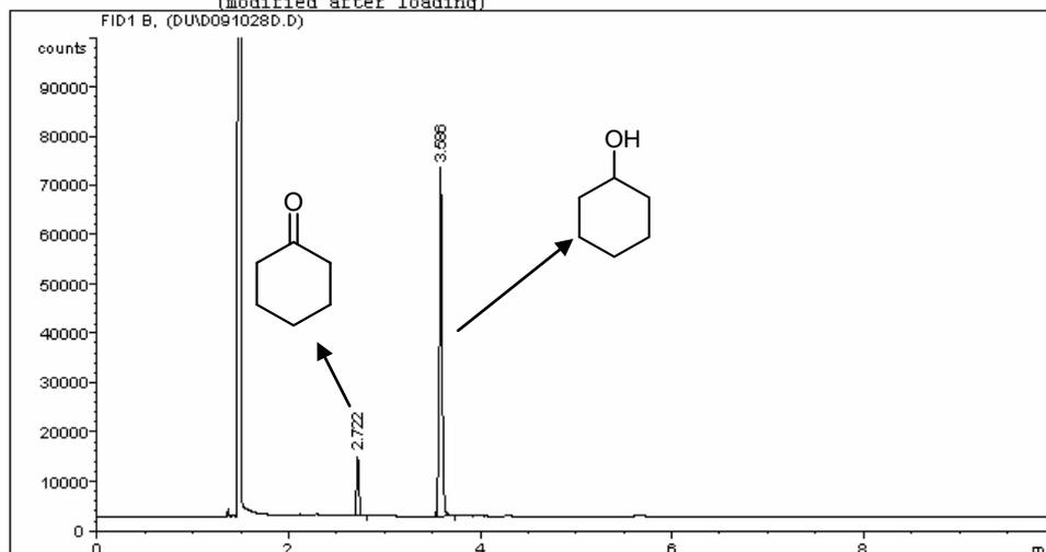
Fig. 25 GC chromatogram of the reaction mixture (Table 1, Entry 10 in main text)
