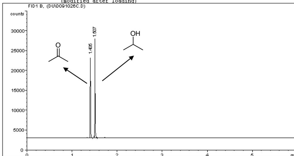
Fig. 26 GC chromatogram of the reaction mixture (Table 1, Entry 11 in main text)
