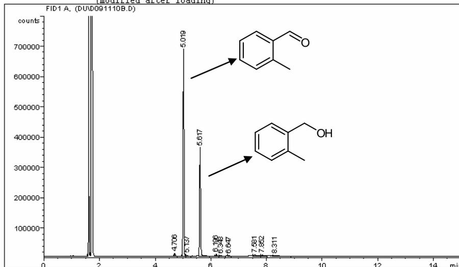
Fig. 19 GC chromatogram of the reaction mixture (Table 1, Entry 4 in main text)
