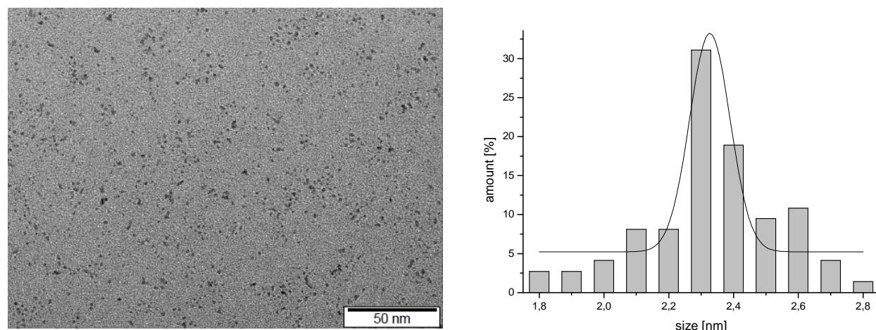
Figure 2. TEM image of Ru@[EMIM][Acetate] (left) and size distribution for 100 particles (right).
