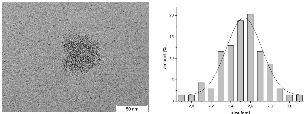
Figure 3. TEM image of Ru@[EMIM][Acetate] left and size distribution for 100 particles (right) after catalysis.
