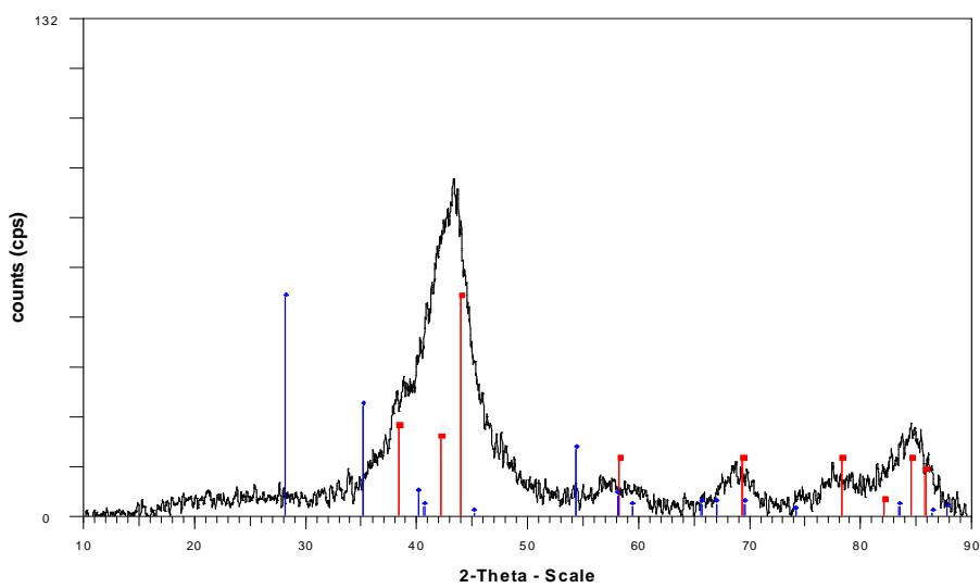
Figure 1. X-ray diffractogram of Ru@[C<sub>12</sub>MIM][BTA] (washed with acetone).
