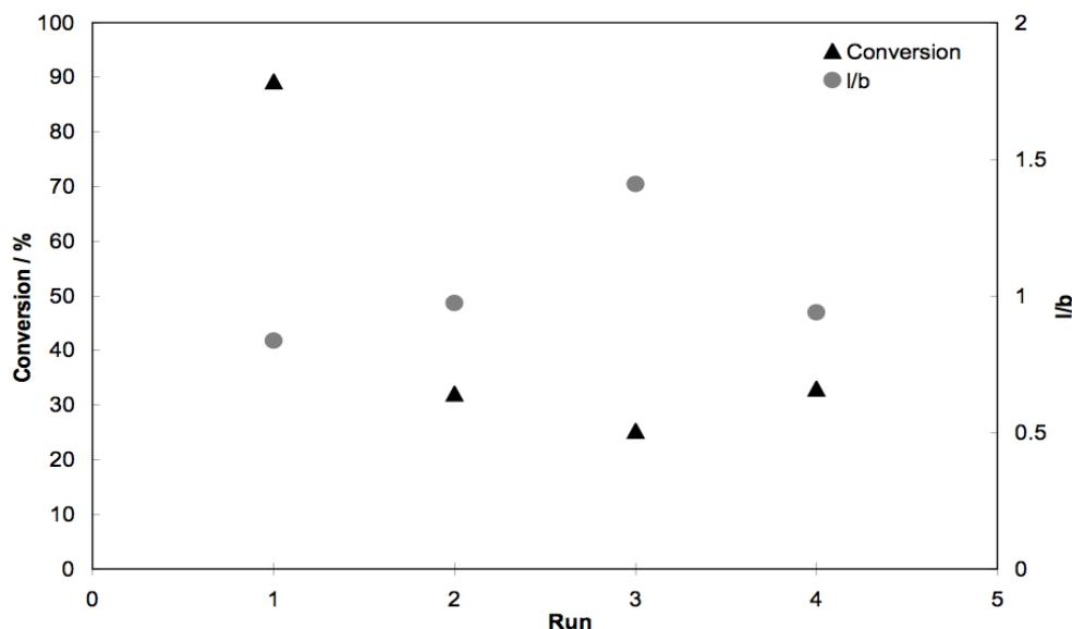
**Figure S 1** Repetitive batch experiments for the hydroformylation of 1-octene with complex **1** supported onto Trisopor 50 ( $80^\circ\text{C}$ ,  $\text{pCO}_2 = 100$  bar,  $\text{CO}/\text{H}_2 = 20$  bar, 2.35 mmol 1-octene; S/C = 500, 3h)
