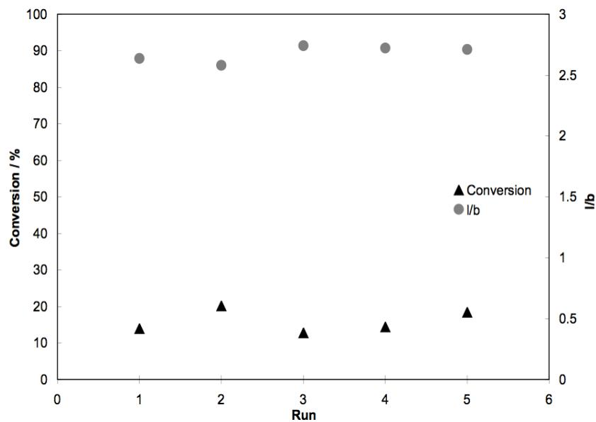
**Figure S 4** Repetitive batch experiments for the hydroformylation of 1-octadecene with complex **1** supported onto Amberlyst 26 OH ( $80^\circ\text{C}$ ,  $\text{pCO}_2 = 100$  bar,  $\text{CO}/\text{H}_2 = 20$  bar, 2.19 mmol 1-octene; S/C = 2000, 20h)
