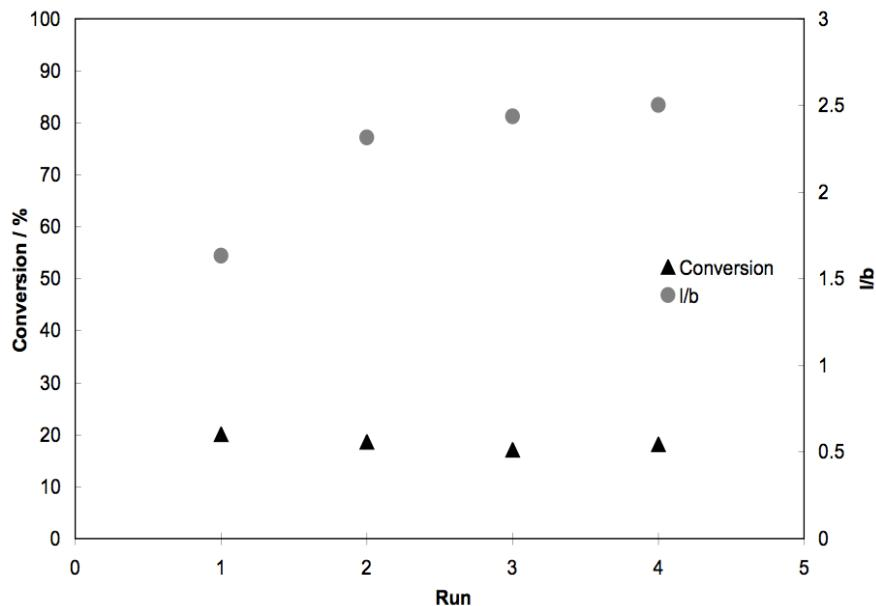
**Figure S 3** Repetitive batch experiments for the hydroformylation of 1-octadecene with complex **1** supported onto Dowex marathon A2 ( $80^\circ\text{C}$ ,  $\text{pCO}_2 = 100$  bar,  $\text{CO}/\text{H}_2 = 20$  bar, 2.19 mmol 1-octene; S/C = 2000, 20h)
