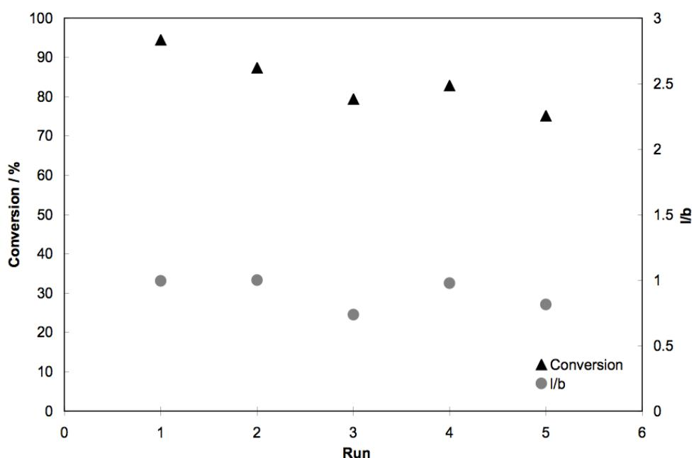
**Figure S 2** Repetitive batch experiments for the hydroformylation of 1-octene with complex **1** supported onto Trisopor 137 ( $80^\circ\text{C}$ ,  $\text{pCO}_2 = 100$  bar,  $\text{CO}/\text{H}_2 = 20$  bar, 2.35 mmol 1-octene; S/C = 500, 3h)
