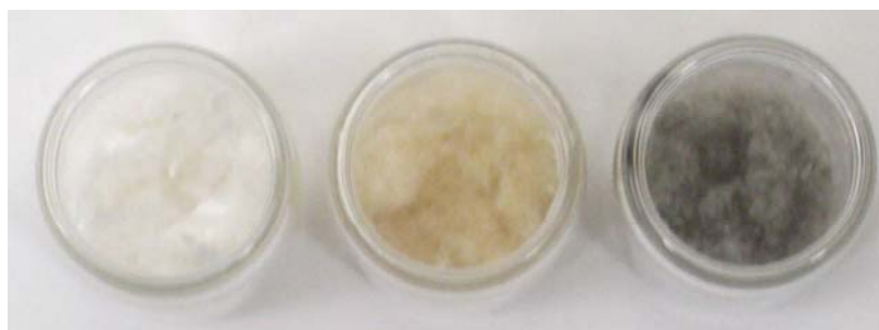
Figure S1. Digital camera images of CNCs freeze-dried powder before impregnation (left), after impregnation, before reduction (middle) and after impregnation and reduction (right)
